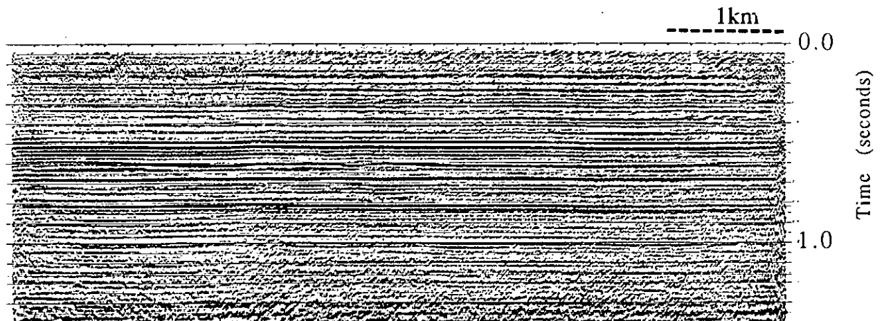
Fig. 2b: Vertical (P-P) component stack section with final statics applied.
