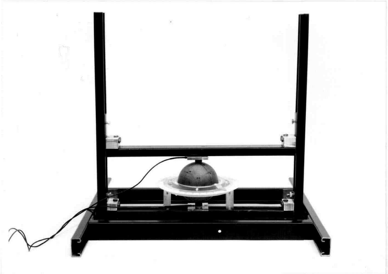
FIG. 2. Photograph of the laboratory set-up used in shooting and recording on the phenolic sphere. Transducers are in contact with the sphere at its top and bottom.
