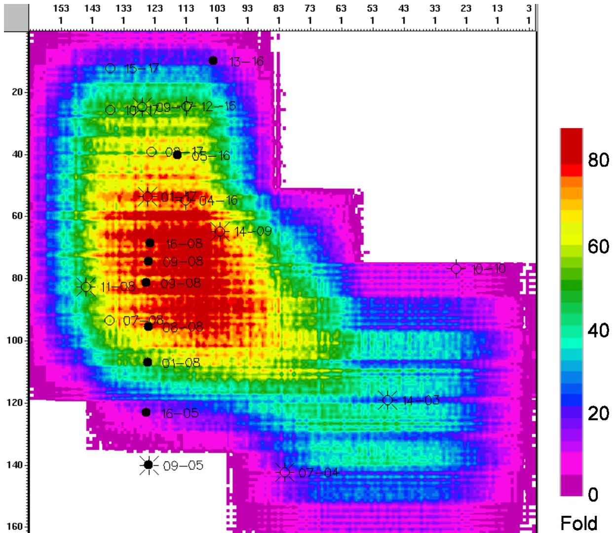
Fig. 15. Processed stacking P-S fold distribution at 2200 ms. Bin size 30 m x 30 m. Beaverhill Lake target level.
