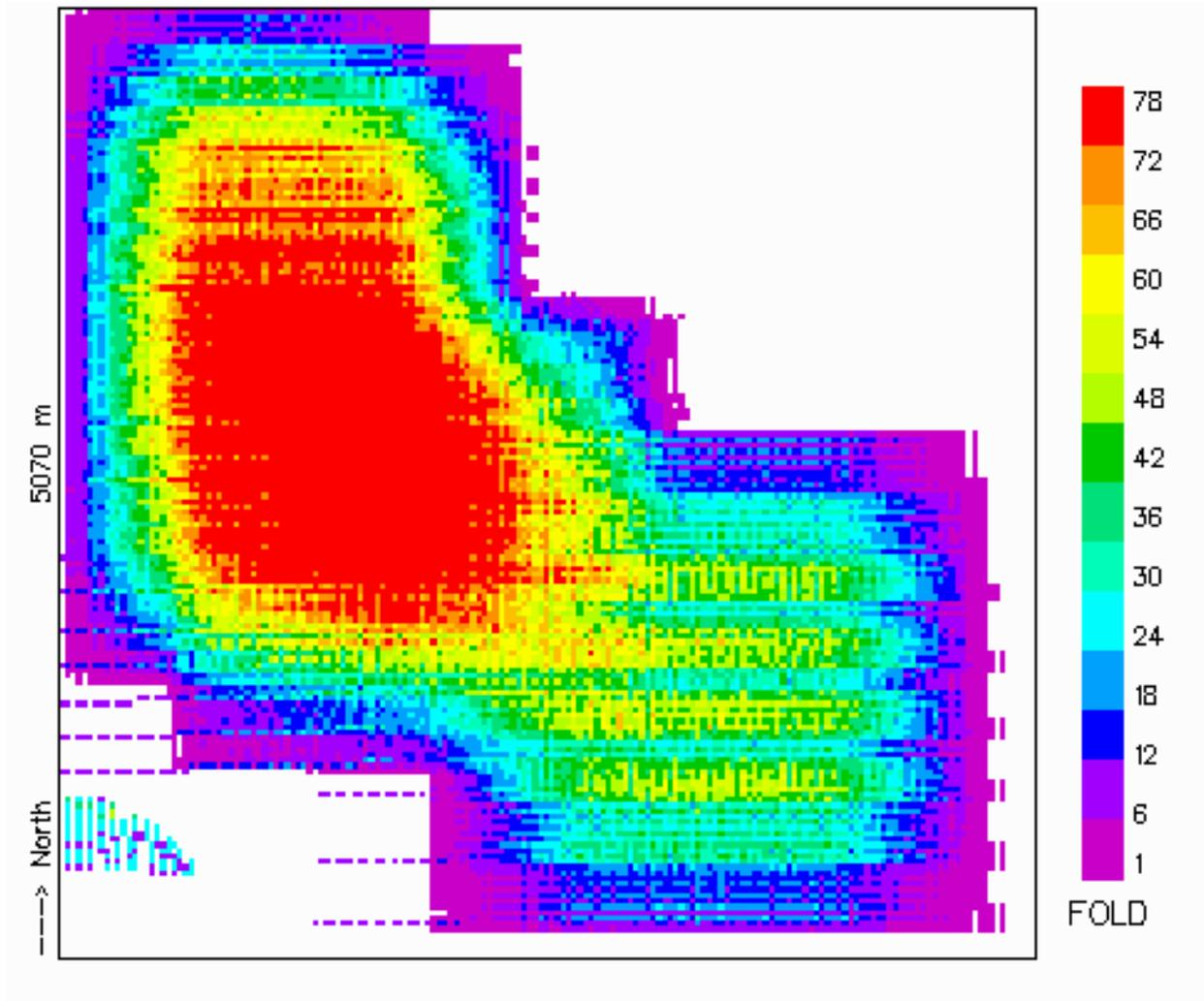
Fig 12. Post-survey depth-variant P-S fold distribution. Bin size 30 m x 30 m. Beaverhill Lake target level.
