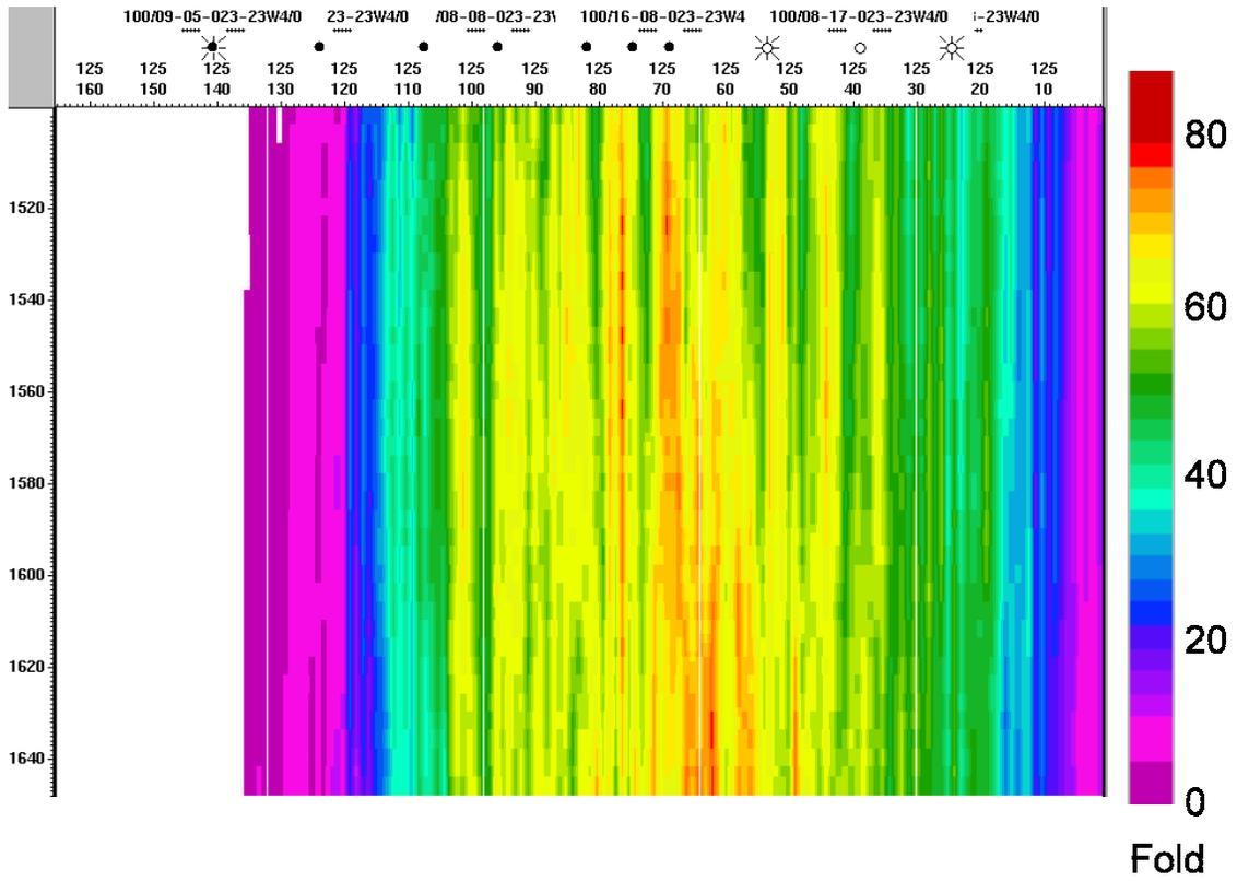
Fig. 20. Detail of processed stacking fold for P-S data from cross-line 125 through survey volume at Glauconitic reservoir level. Trace spacing is 30 m x 30 m.
