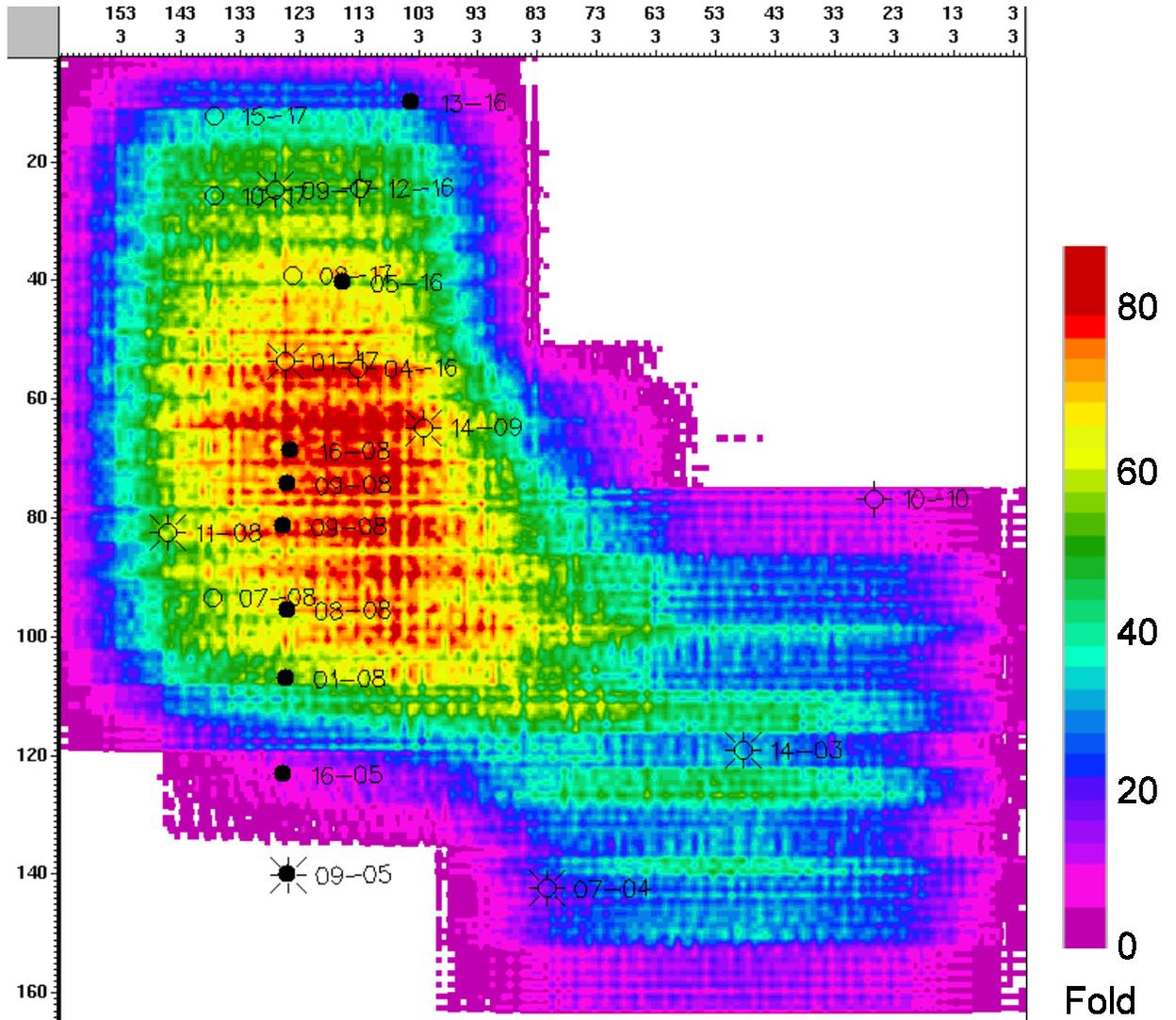
Fig. 14. Processed stacking P-S fold distribution at 1700 ms. Bin size 30 m x 30 m. Glauconitic target level.
