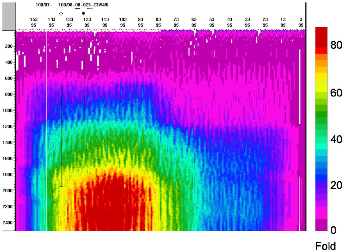
Fig. 17. Processed stacking fold for P-S data from in-line 95 through survey volume. Trace spacing is 30 m.
