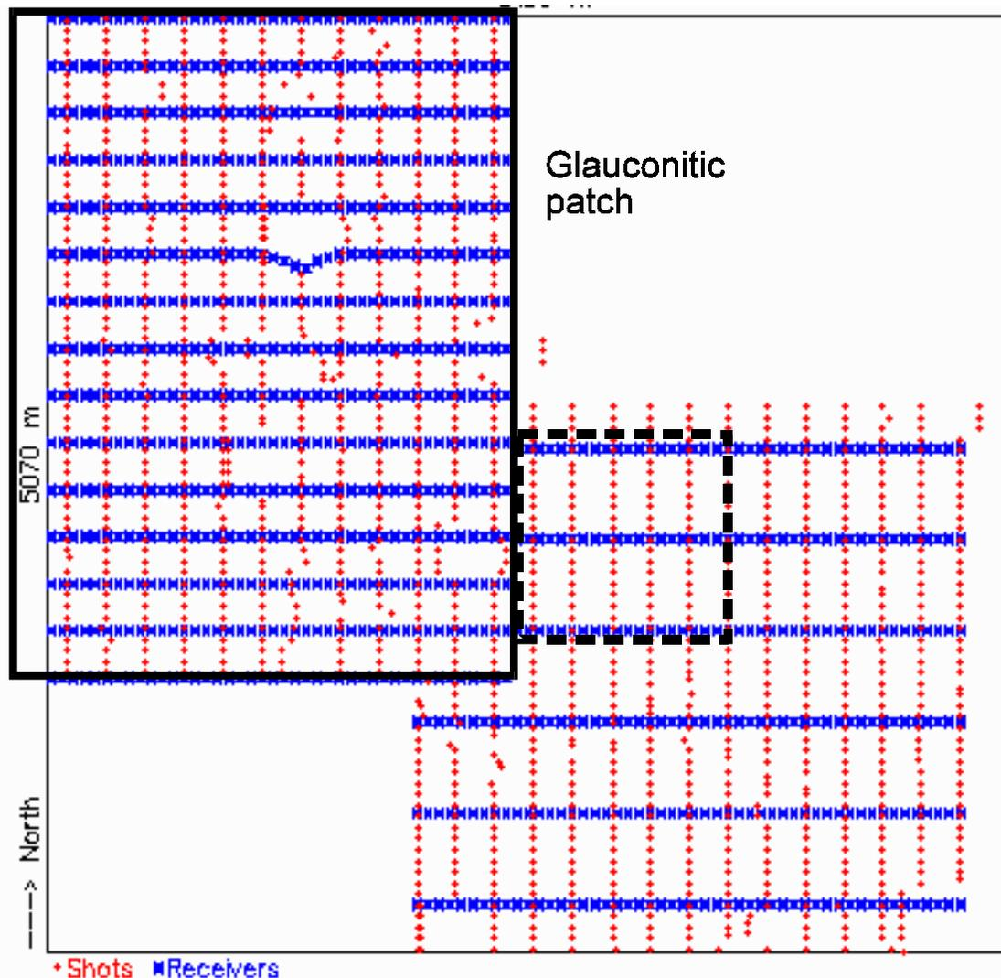
Fig 4. Geometry of Glauconitic path. All shots were fired in rectangle outlined by a solid line; receivers in dashed box were also live.
