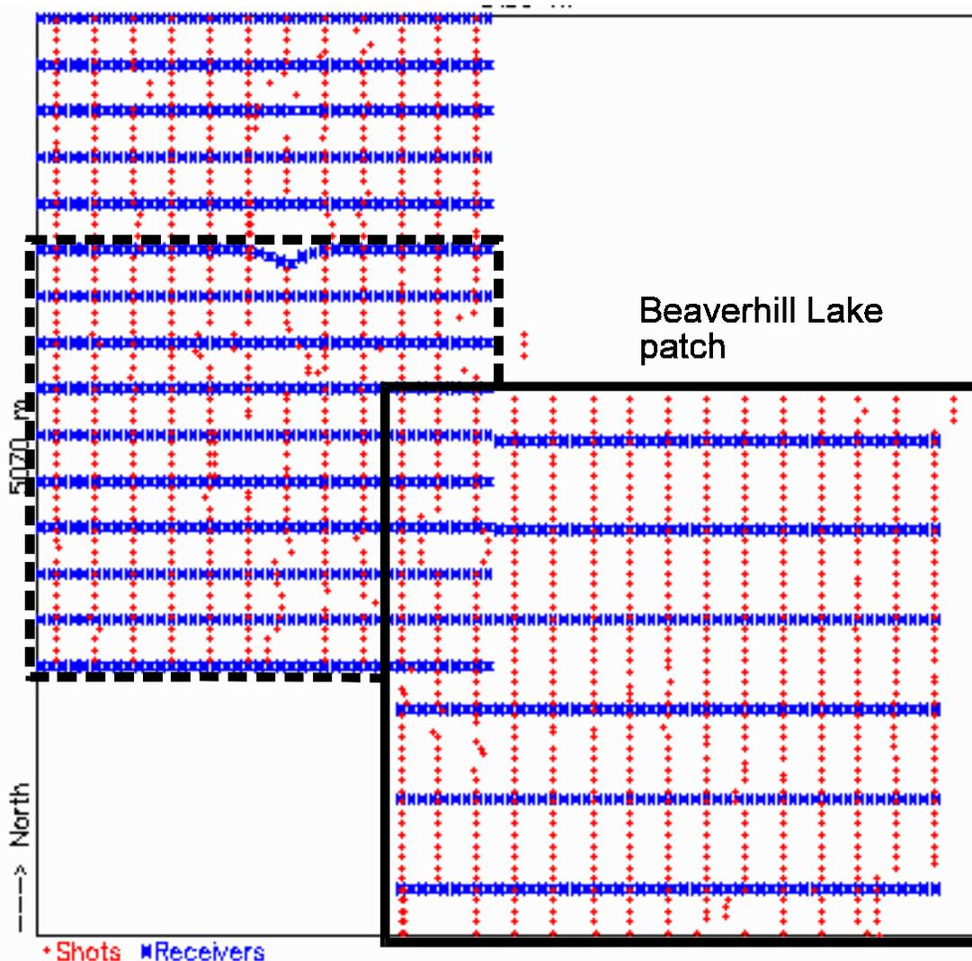
Fig 5. Geometry of Beaverhill Lake path. All shots were fired in rectangle outlined by a solid line; receivers in dashed box were also live.
