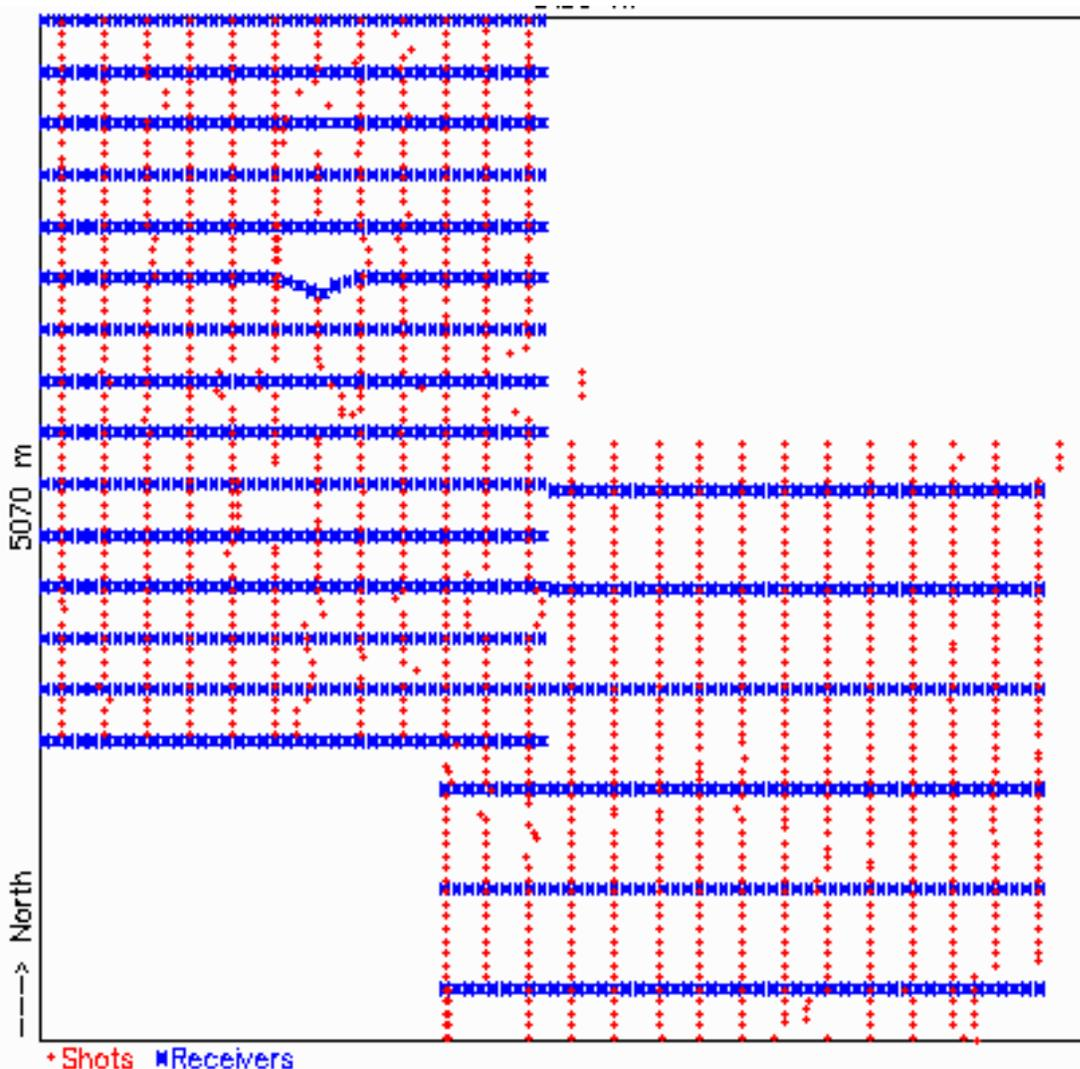
Fig. 3. Field survey source and receiver line geometry for Blackfoot 3C-3D program
