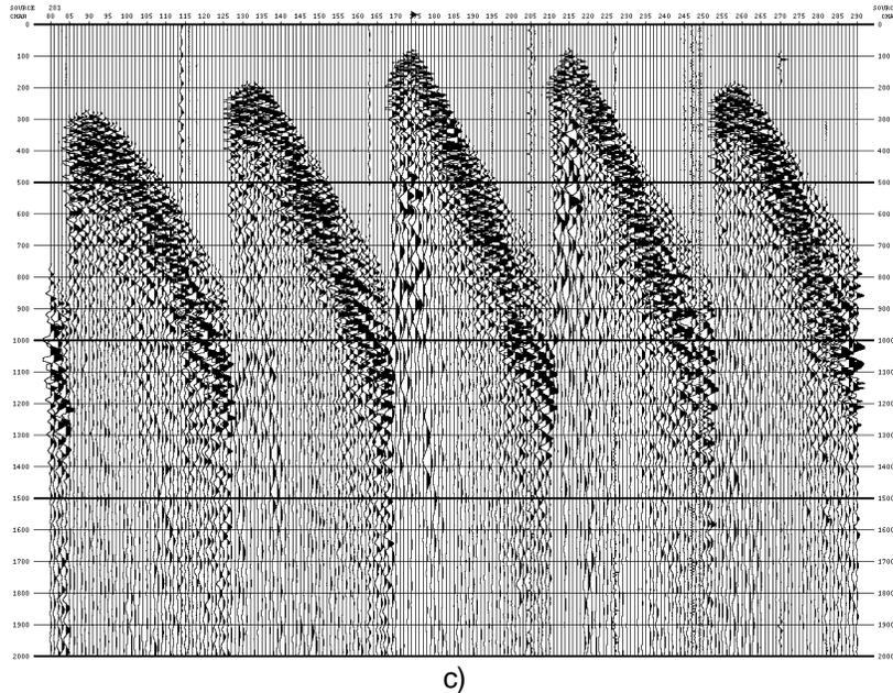
Fig.2. Portion of representative field records from a) vertical, b) north and c) east components
