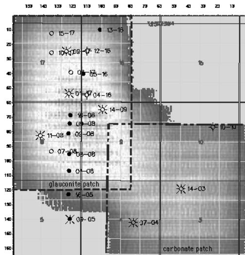
Fig.1. Fold map of the Blackfoot 3C 3D seismic survey
