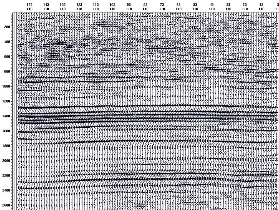
Fig.8. Inline 110 display from Pulsonic's radial migrated volume
