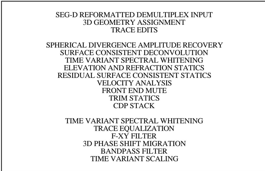
Fig.6. Sensor's vertical processing flow
