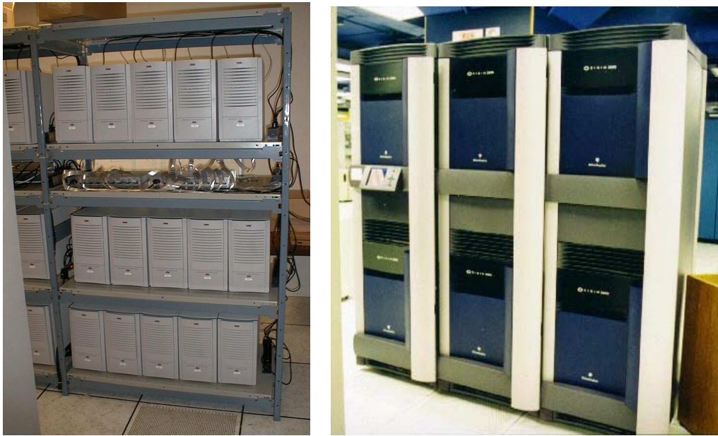
Figure 1. MACI systems: (left) A tightly networked cluster of 30 Compaq / DEC Alpha systems running at 500MHz is installed at the University of Calgary. (right) a 42 processor SGI Origin 2000 is installed at the University of Alberta.
