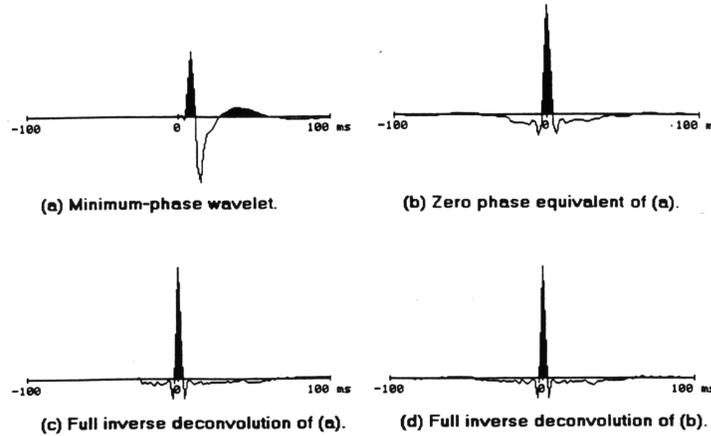
Fig. 1: The effect of deconvolution on known minimum-phase and zero-phase wavelets (from B. Russell, SEG inversion course notes).
