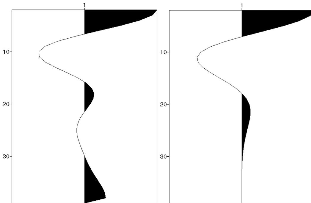
Fig. 28: The trace autocorrelation (left) and the Ricker wavelet autocorrelation (right).
