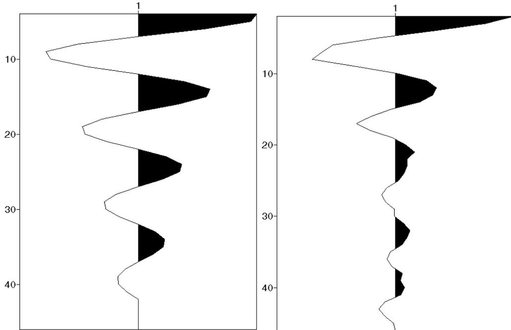
Fig. 4: The model wavelet (left) and a Wiener-Levinson wavelet estimate (right).
