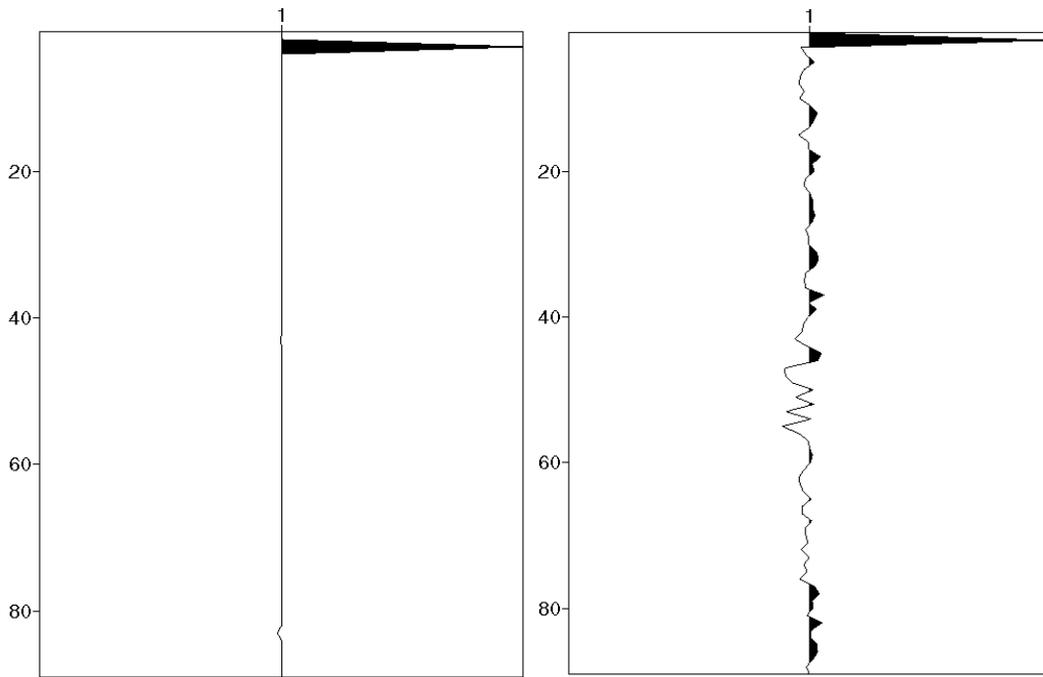
Fig. 16: Model wavelet deconvolution (left) and Hilbert wavelet deconvolution (right).
