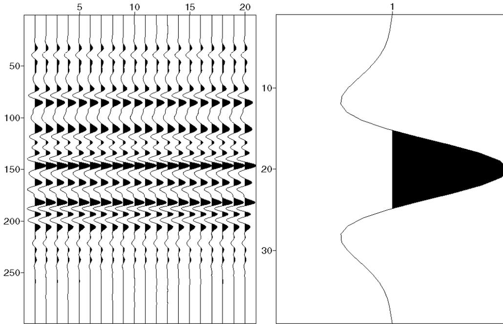
Fig. 20: primaries only zero-phase synthetic trace and the Ricker wavelet used to create it.
