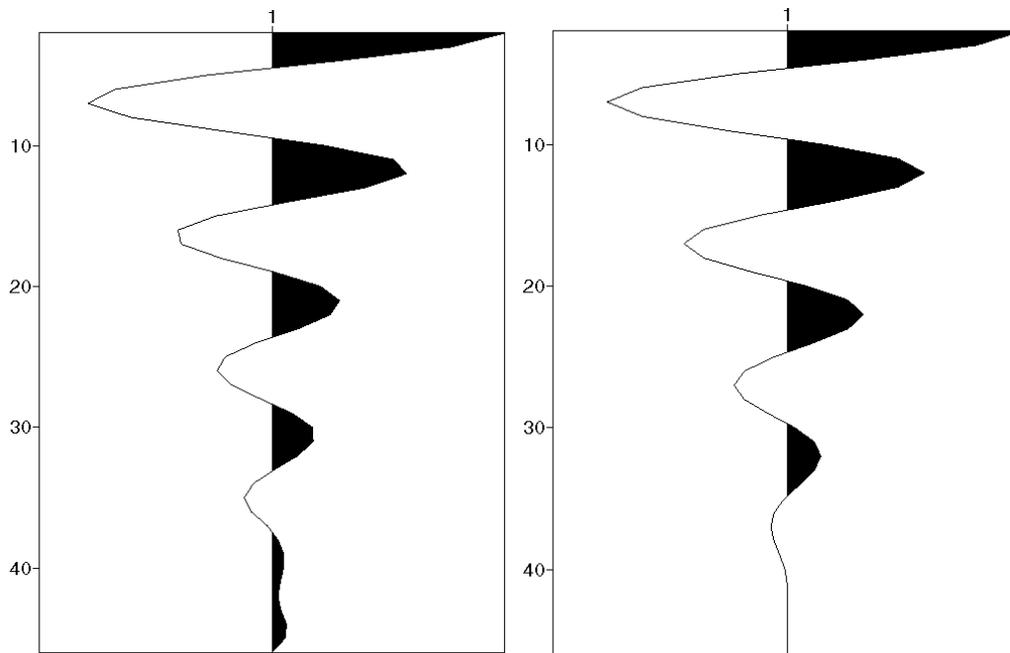
Fig. 12: The trace autocorrelation (left) and the wavelet autocorrelation (right).
