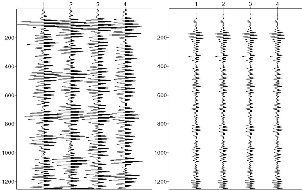
Fig. 43: Near offset traces (left) and their convolution with a Klauder zero-phase filter (right).
