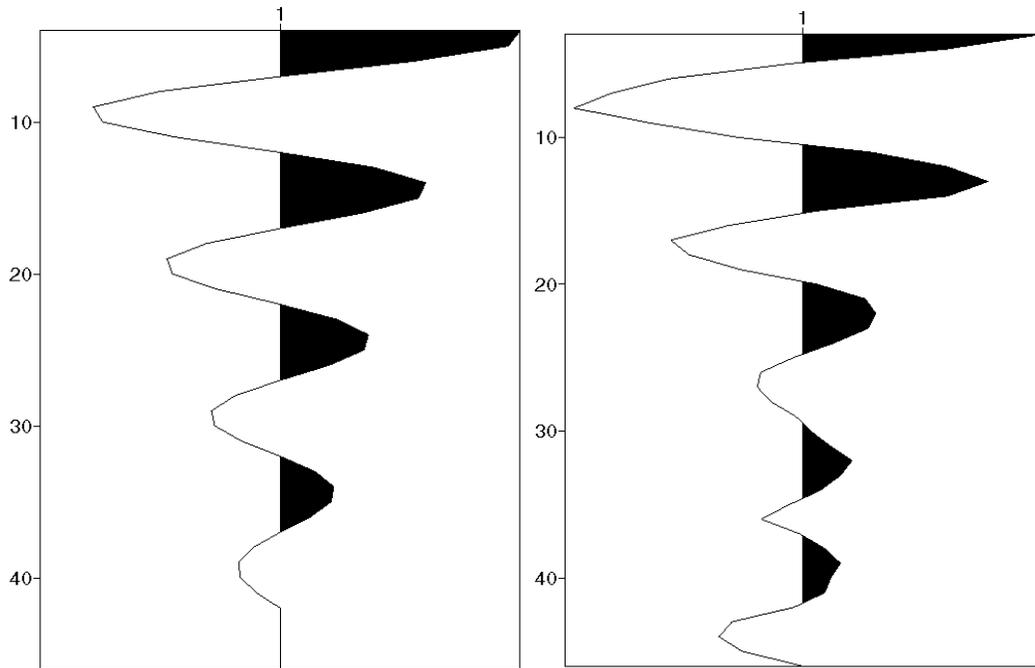
Fig. 14: The model wavelet (left) and a Hilbert transform wavelet estimate (right).
