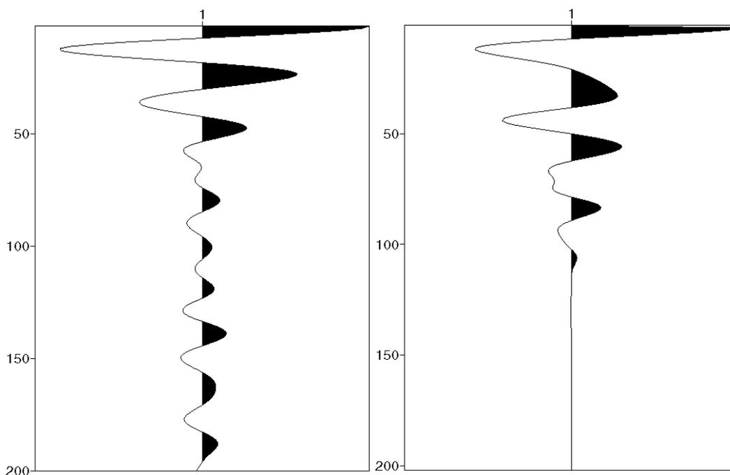
Fig. 37: Near offset trace autocorrelation (left) and truncated wavelet autocorrelation (right).
