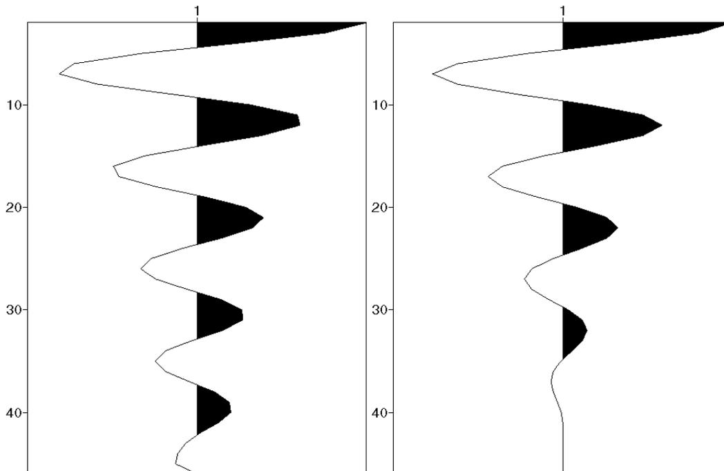
Fig. 3: The trace autocorrelation (left) and the minimum-phase wavelet autocorrelation (right).
