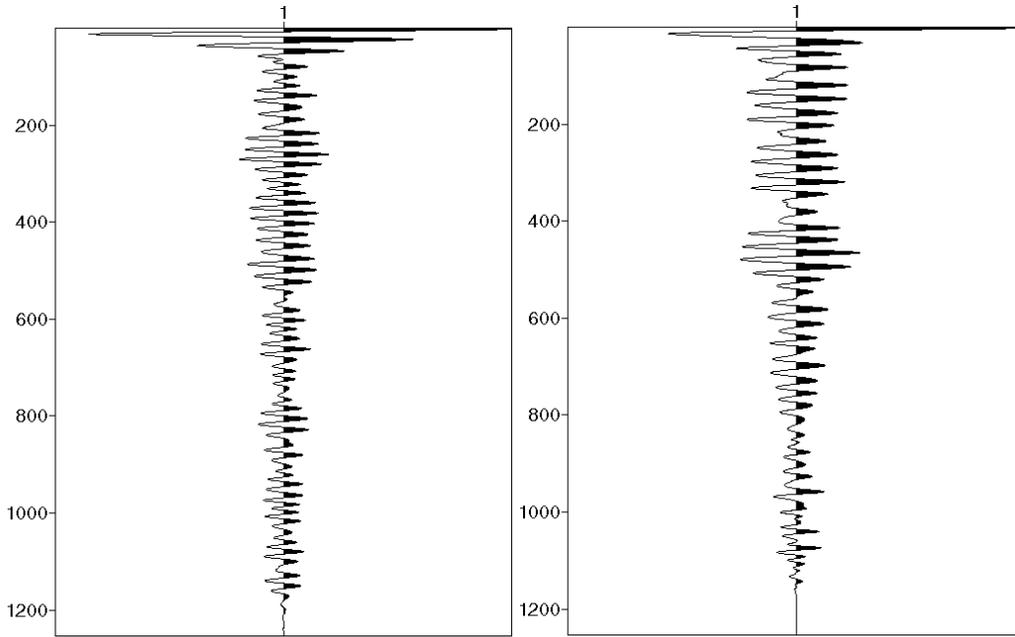
Fig. 35: Near offset trace autocorrelation (left) and in-situ wavelet autocorrelation (right).
