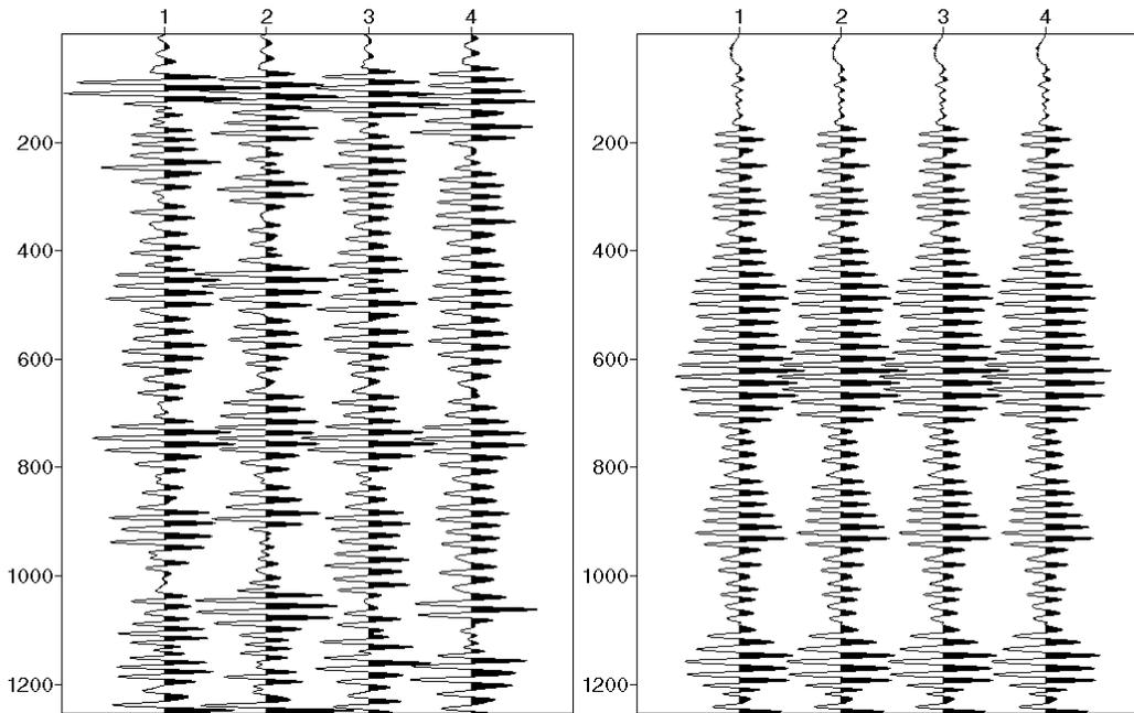
Fig. 41: Near offset traces (left) and their convolution with an in-situ filter (right).
