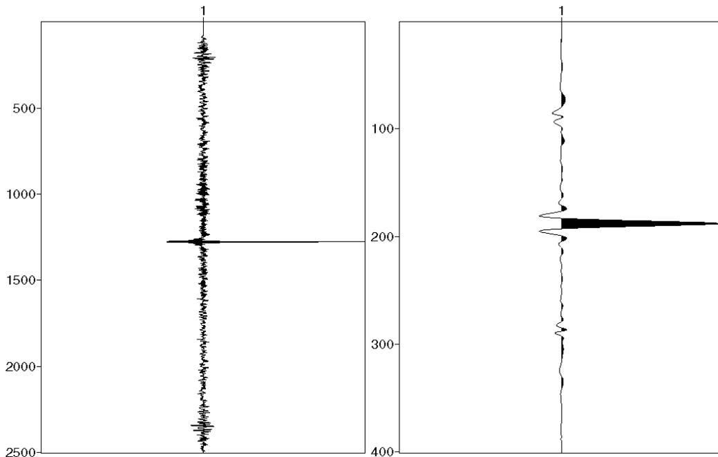
Fig. 40: Measured wavelet deconvolution (left) and Klauder wavelet deconvolution (right).
