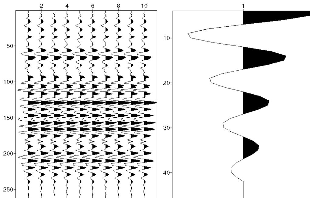
Fig. 11: A primaries with multiples minimum-phase synthetic trace and the model wavelet used to create it.
