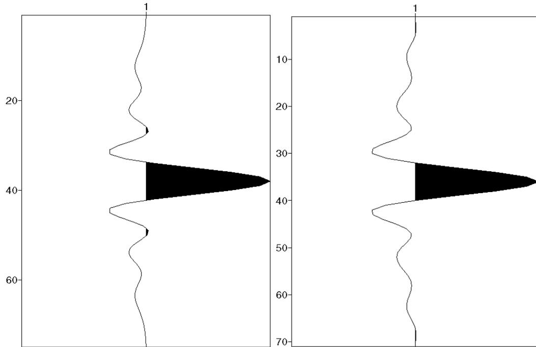
Fig. 30: Ricker wavelet deconvolution (left) and Klauder wavelet deconvolution (right).
