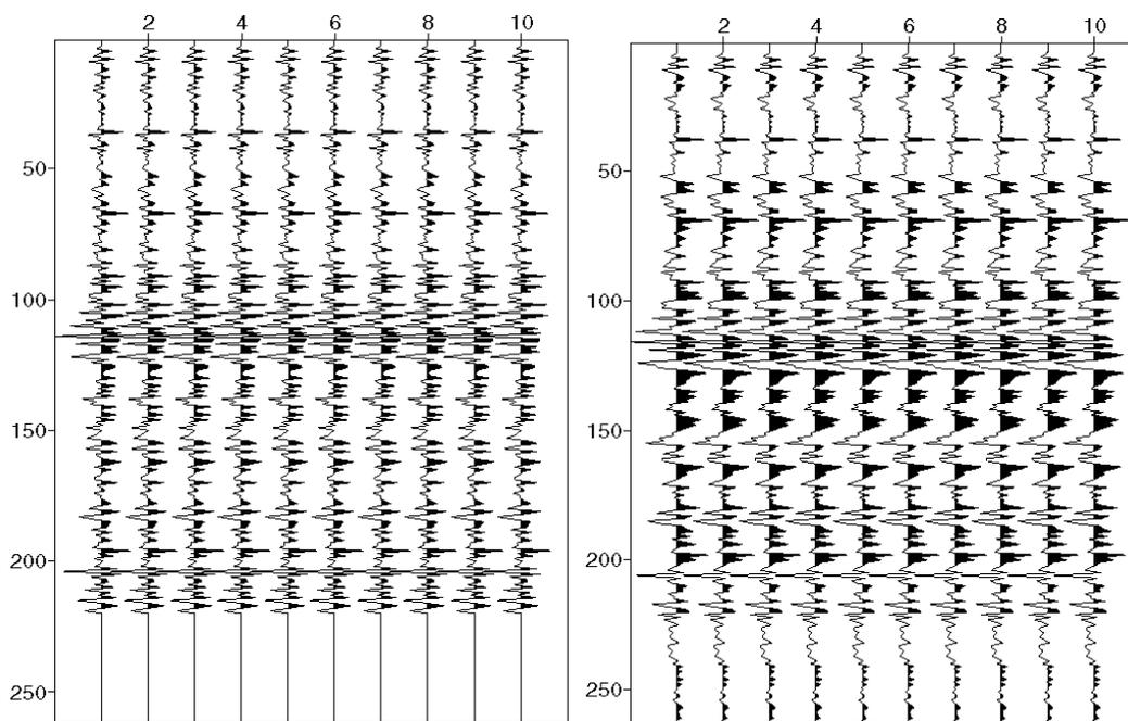
Fig. 18: The actual well-log derived reflectivity series (left) and the Hilbert transform reflectivity series estimate (right).
