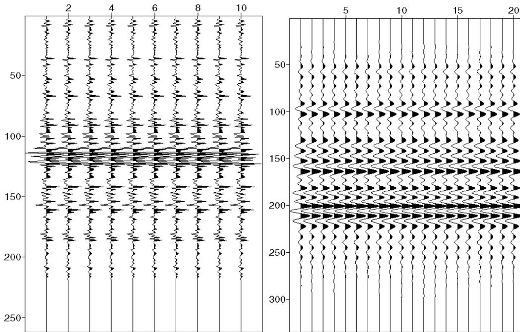
Fig. 24: The actual well-log derived reflectivity series (left) and the Ricker band-limited reflectivity series estimate (right).
