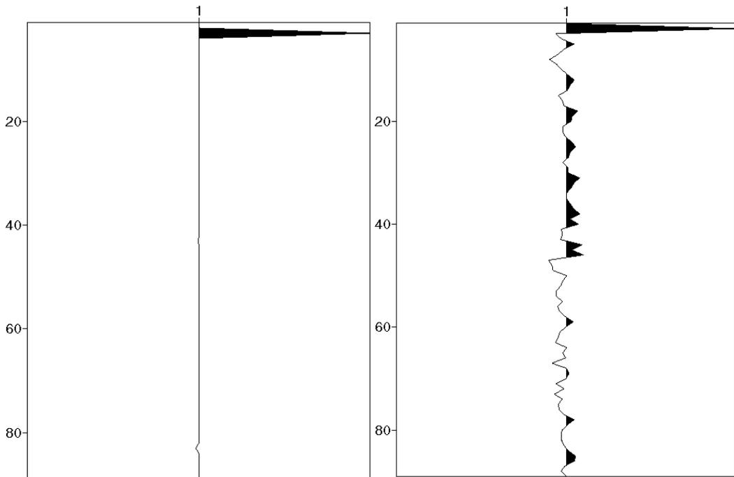
Fig. 7: Model wavelet deconvolution (left) and Hilbert wavelet deconvolution (right).
