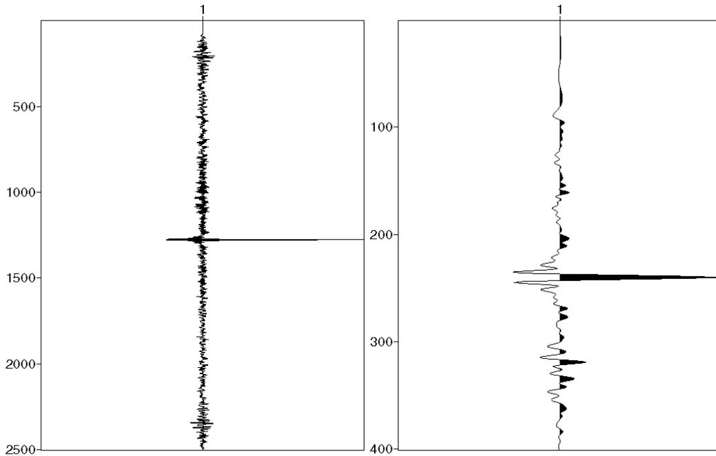
Fig. 39: Measured wavelet deconvolution (left) and truncated wavelet deconvolution (right).
