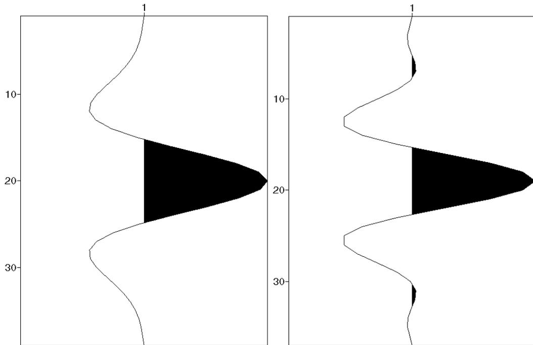
Fig. 22: The model Ricker wavelet (left) and a Klauer zero-phase wavelet estimate (right).
