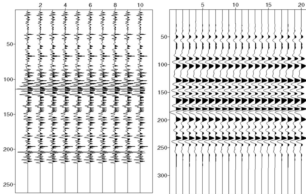
Fig. 31: The actual well-log derived reflectivity series (left) and the Ricker band-limited reflectivity series estimate (right).
