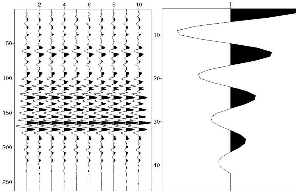
Fig. 2: A primaries only minimum-phase synthetic trace and the wavelet used to create it.
