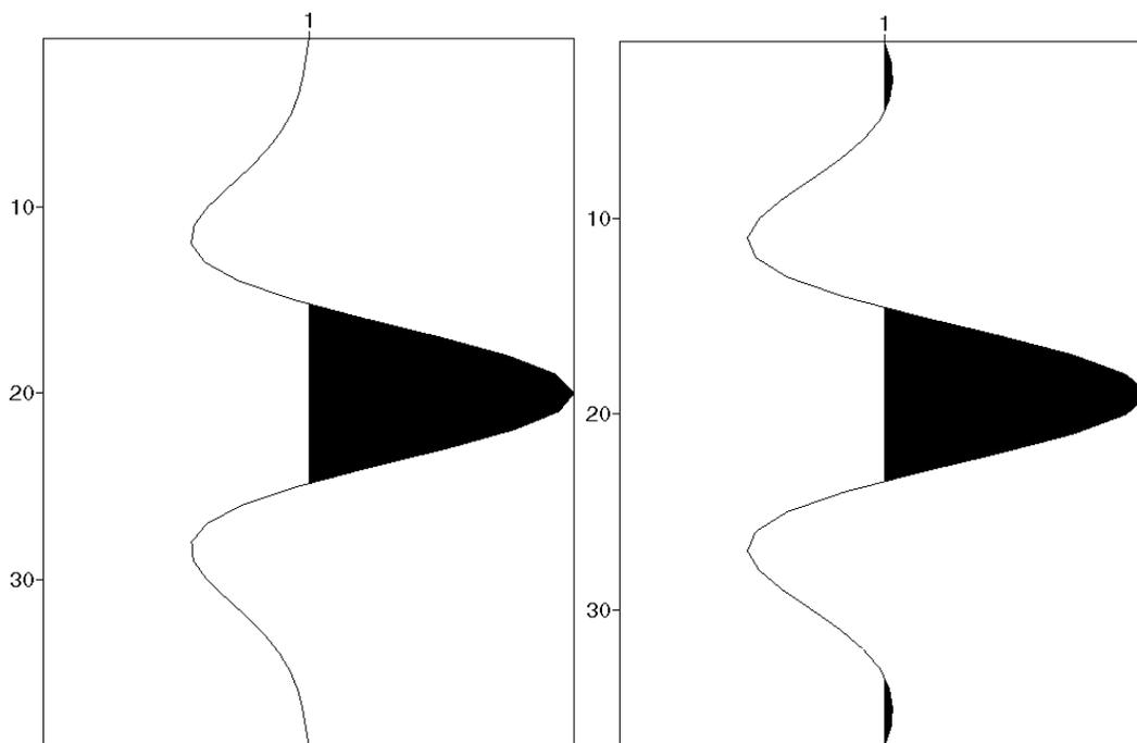
Fig. 29: The model Ricker wavelet (left) and a Klauer zero-phase wavelet estimate (right).
