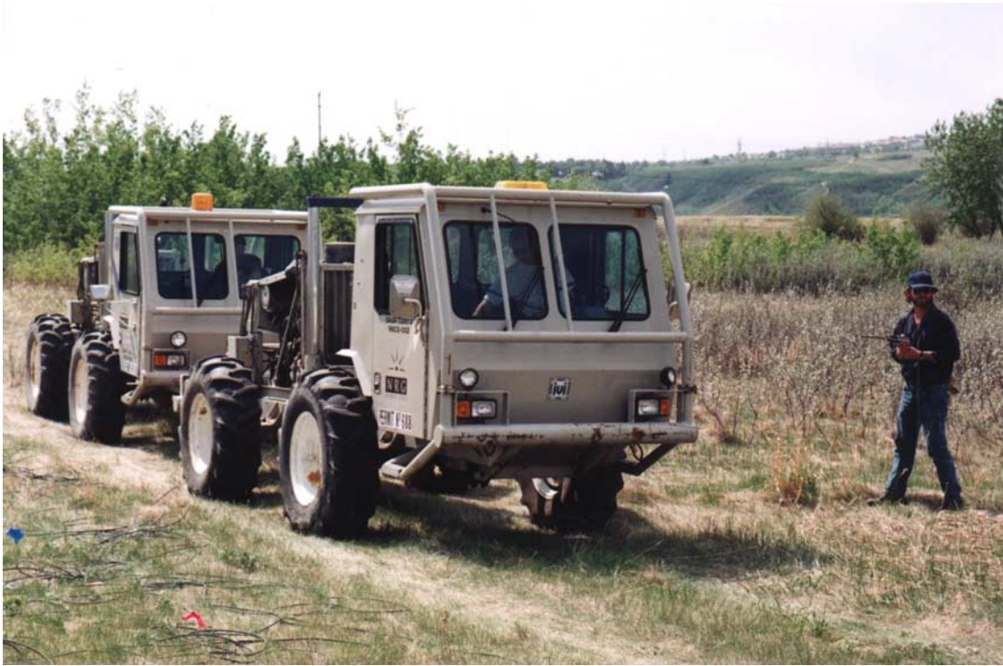
Figure 3. Two buggy-mounted IVI Minivib sources were loaned by NRG for work on the 2-D test line (shown) and the 3C-3D survey at Shaganappi. One buggy was fitted with a P-wave pad, while the other was fitted with a shear-wave pad.
