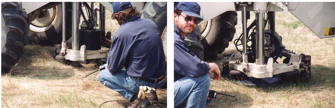
Figure 4. IVI Minivib vibrator sources: a vertically vibrating pad (left) for P and P-S surveys and a horizontally vibrating pad (right) for pure-shear surveying.
