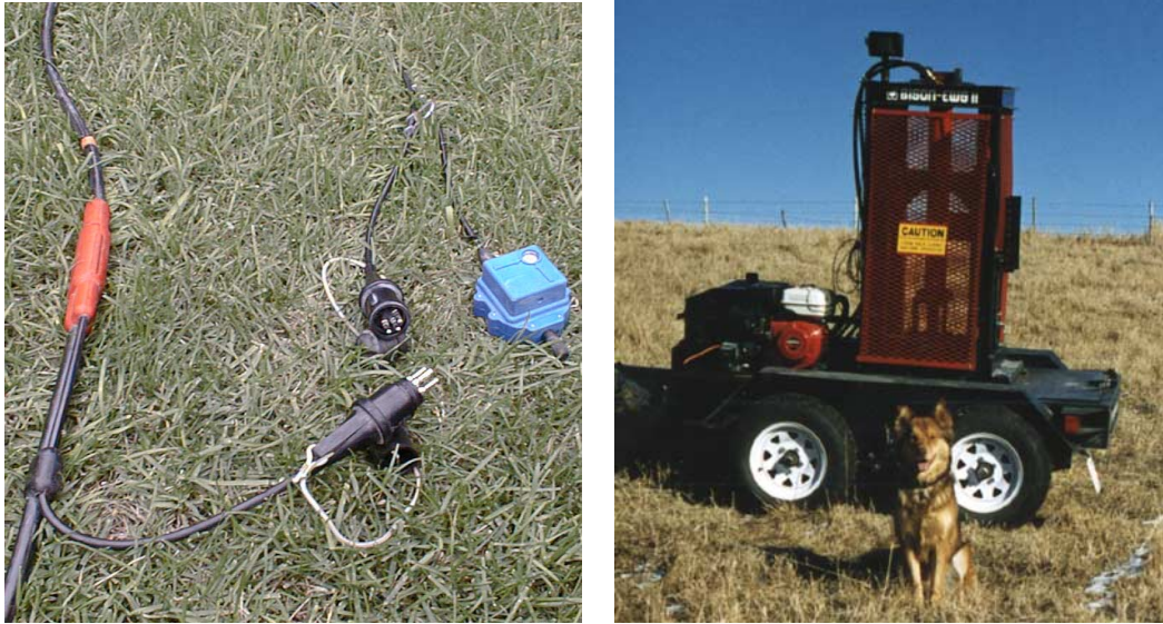
Figure 2. Acquisition equipment for 2-D test line. Special-purpose 3-C cable (left) uses a single 6-pin geophone connector to ease deployment and eliminate field-connection errors. Bison EWG-II "Thumper" (right) uses an accelerated-mass drop as a source (Sue Miller's dog "Tundra" is shown for scale).
