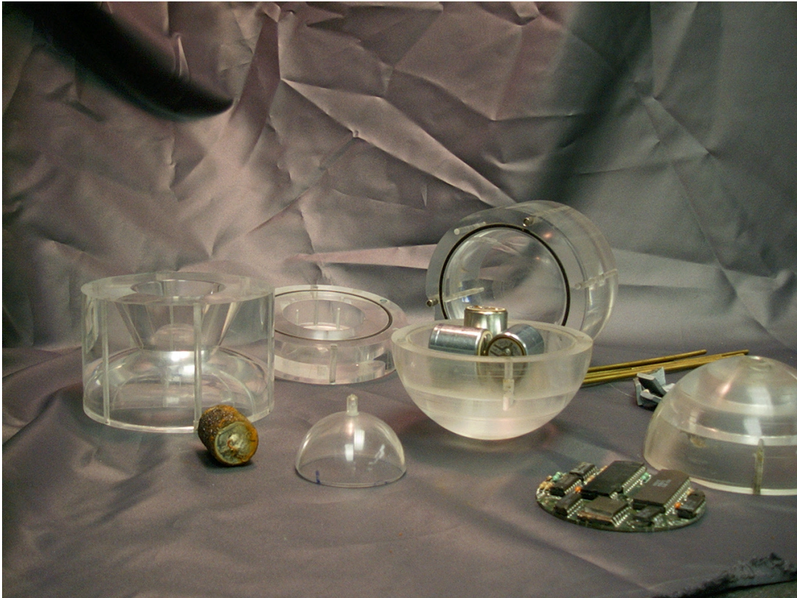
Figure 3. Disassembled parts of the geophone prototypes
