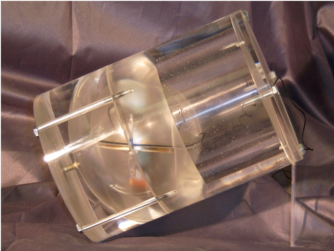
Figure 20. The prototype OBC (Ocean Bottom Cable) device.
