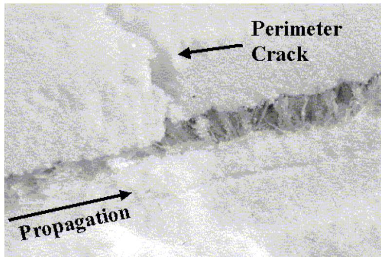
Figure 1. Photograph of a weak layer after a whumpf has occurred. This whumpf was triggered approximately 8 m to the left of the area photographed. The left side of the photo shows the fractured weak layer that has collapsed. The weak layer on the right side has not fractured. A crack extends vertically between the fractured and unfractured portions of the weak layer. This crack can be seen on the surface, marking the perimeter of the failed weak layer region.
