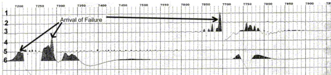
Figure 5. Signal traces produced by the Bison recorder clearly indicating the time of arrival for fracture in the weak layer.
