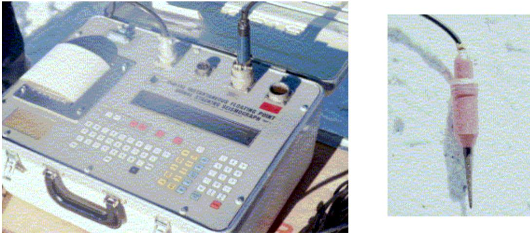
Figure 3. Bison 9000 Series Digital Seismograph and geophones used to measure propagation of fracture through a weak snow layer.
