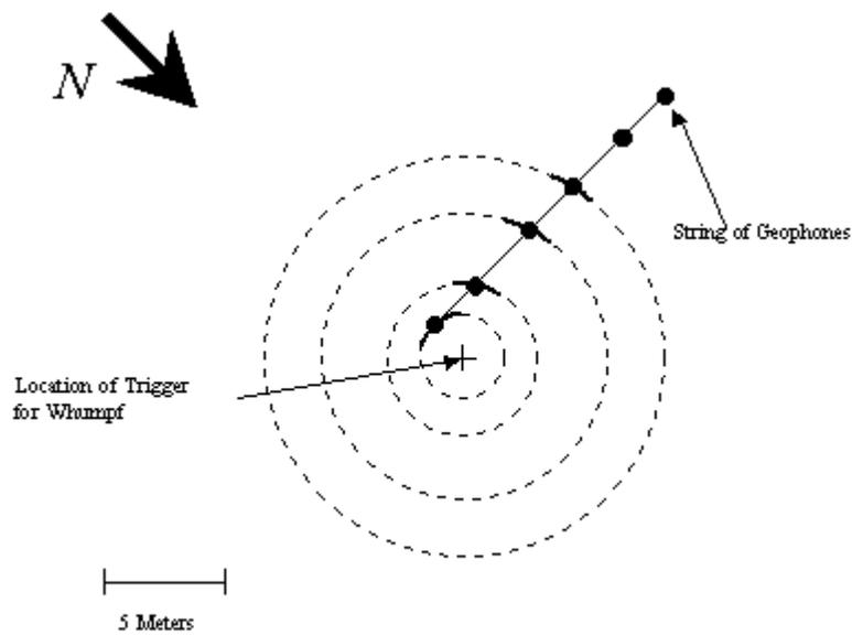
Figure 4. Schematic of propagation experiment. This shows the relative positions of the whumpf trigger point, the recorder and the six geophones. The concentric circles represent the propagating fracture of the weak layer. The dashed lines show assumed propagation.
