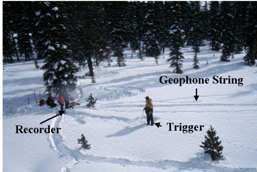
Figure 2. Experiment site showing the location of the geophone string, geophone recorder and spot where a whumpf was successfully triggered.
