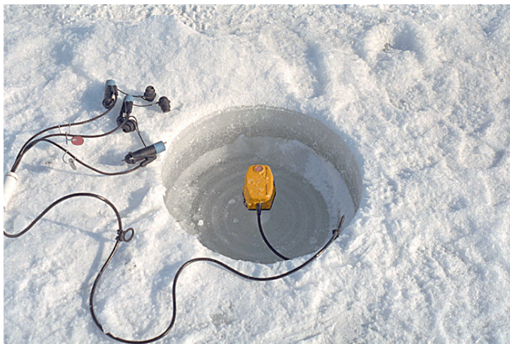
FIG. 4. Typical 3-C geophone plant in an augured hole in the sea ice. Geophones were frozen in with fresh water.
