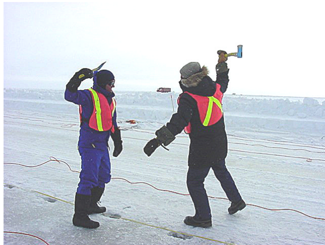
FIG. 7. CREWES personnel preparing V shaped notches in the ice for forty-five degree hammer hits. Notches were chopped every meter for thirty meters (bottom left of picture).
