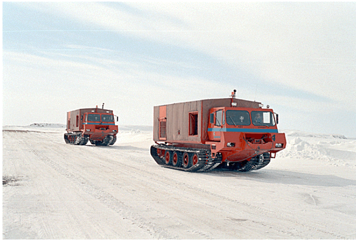
FIG. 6. Mertz 18HD tracked vibrators, heading north to the beginning of the line.
