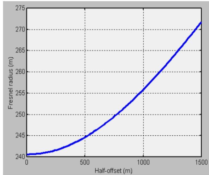
FIG. 10. Fresnel radius varies with half-offset of lower layer
