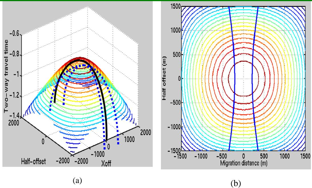
FIG. 4. Specular energy and Fresnel zone of a horizontal reflector in a) Cheops pyramid in  $(x, h, t)$ , and b) contours of Cheops pyramid in  $(x, h)$ .
