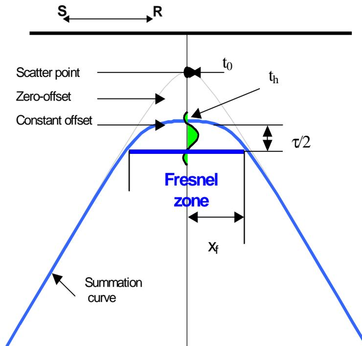
FIG. 2. Fresnel zone for offset section.
