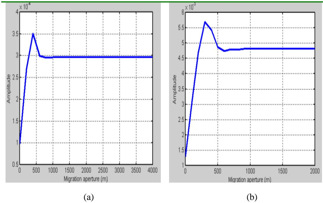
FIG. 9. Migration aperture relates to Fresnel zone of lower layer. a) Zero-offset; b) Half-offset equals 500m.
