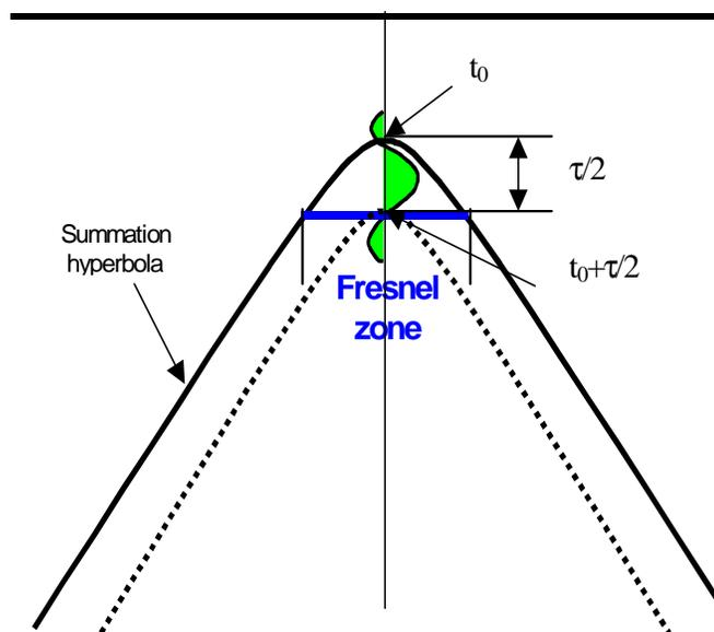
FIG. 1. Fresnel zone for zero-offset section.
