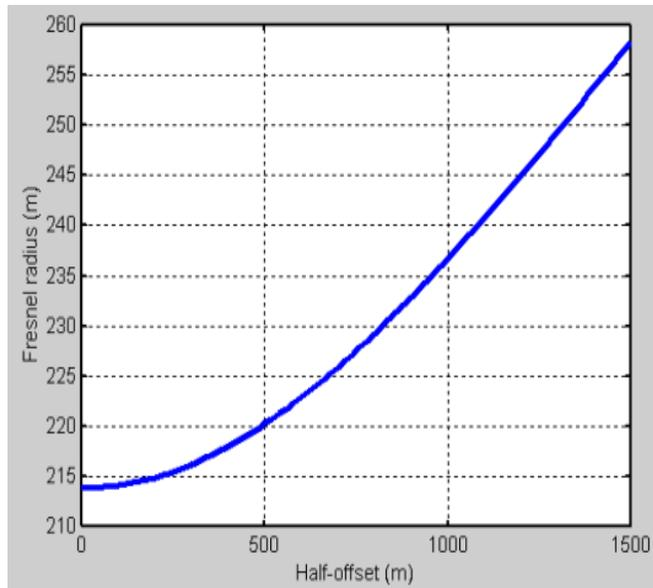
FIG. 8. Fresnel radius varies with half-offset of upper layer.
