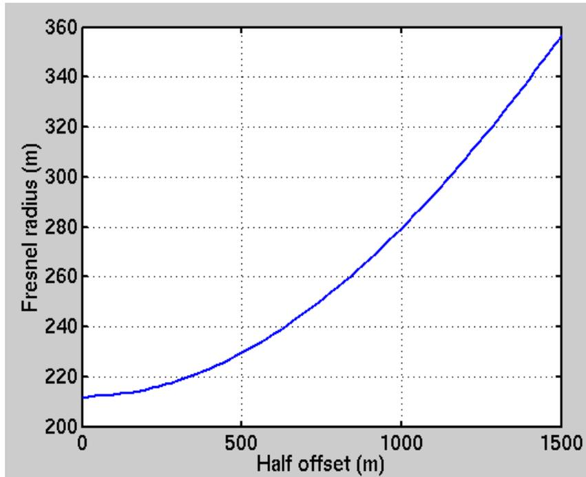
FIG. 3. Fresnel zone radius varies with half source-receiver offset.
