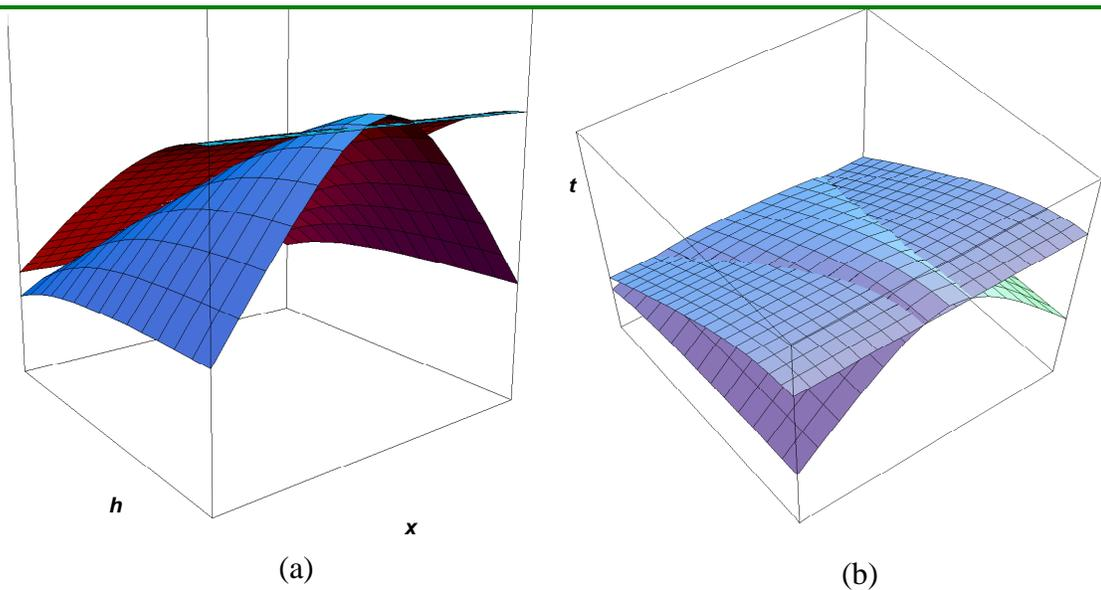
FIG. 5. Prestack Fresnel zone for a horizontal reflector defined by intersecting the hyperbolic cylinder with Cheops pyramid, a) frontal view and b) from above.
