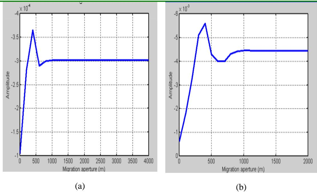
FIG. 7. Migration aperture relates to Fresnel zone of upper layer. a) Zero-offset; b) Half-offset equals 500m.
