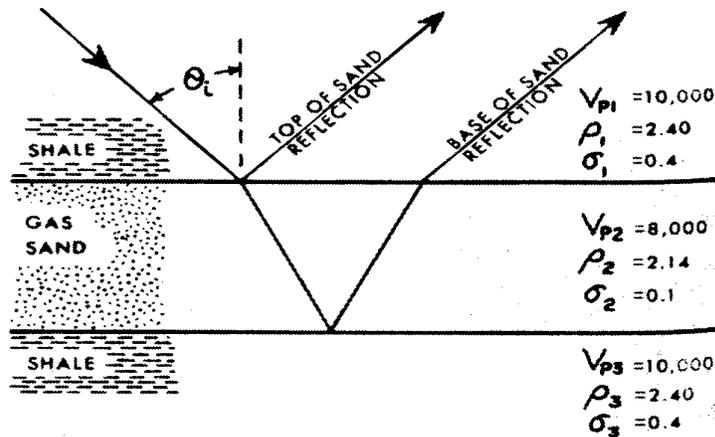
FIG. 6. Two-dimensional geology model used in the numerical example.
