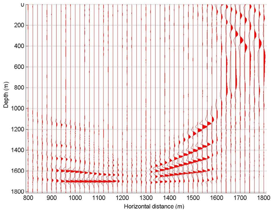
FIG. 6a. Migrated section (model 2) using shots every 400 m, from SP101 to SP114.
