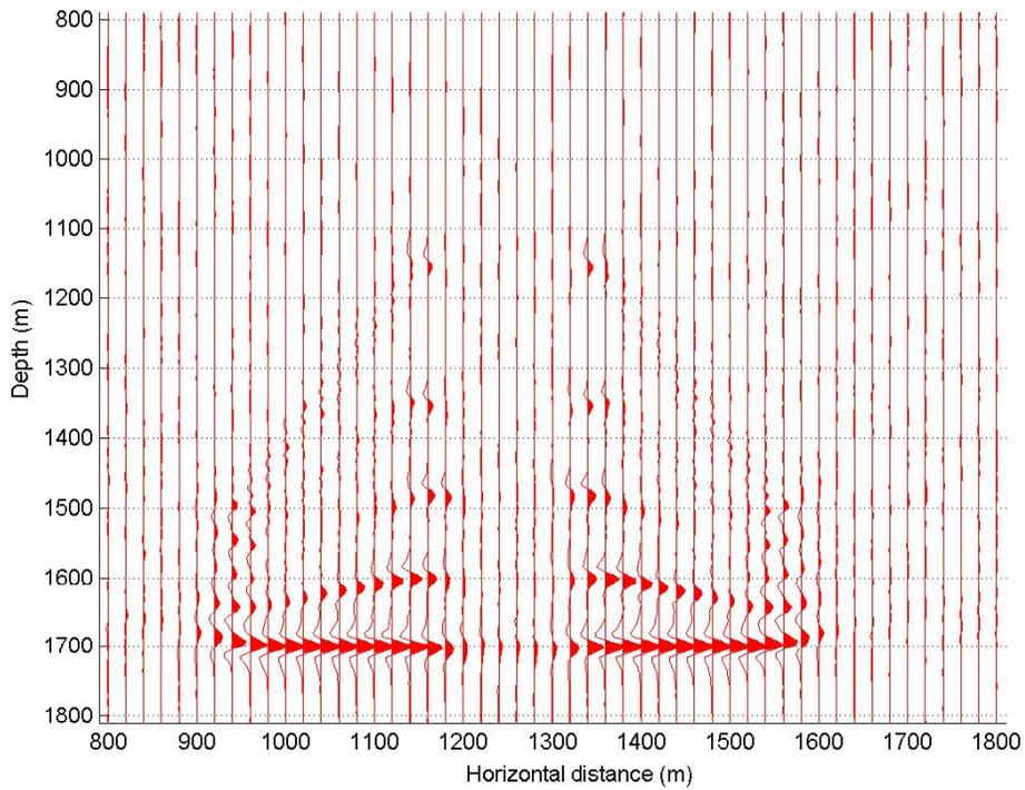
FIG. 7a. Migrated section (model 1) using shots every 400 m, from SP108 to SP120.
