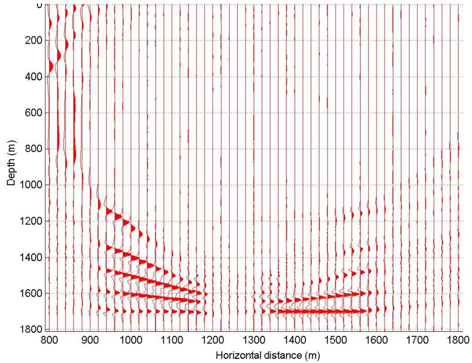
FIG. 6b. Migrated section (model 2) using shots every 400 m, from SP114 to SP127.
