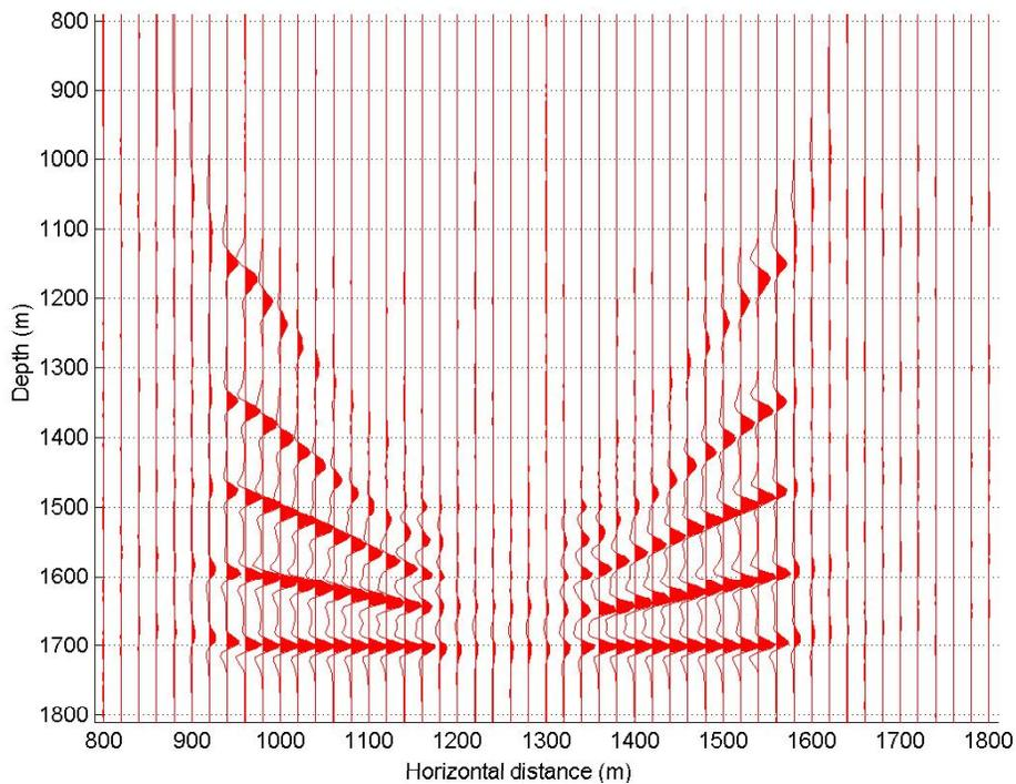
FIG. 4a. Migrated section (model 2) using shots every 100 m, from SP101 to SP127.
