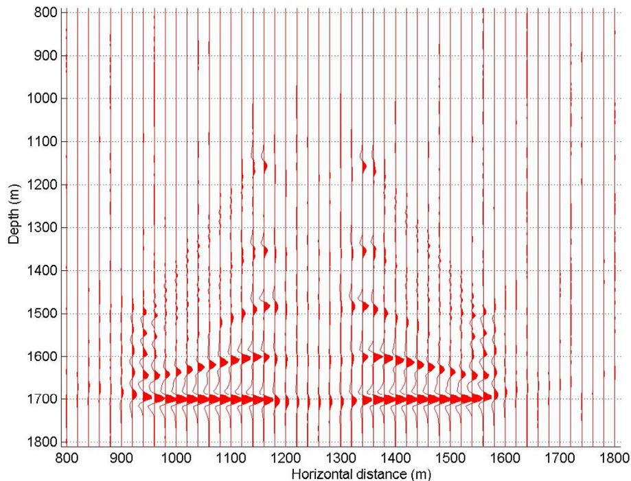
FIG. 3a. Migrated section (model 1) using shots every 100 m, from SP101 to SP127.
