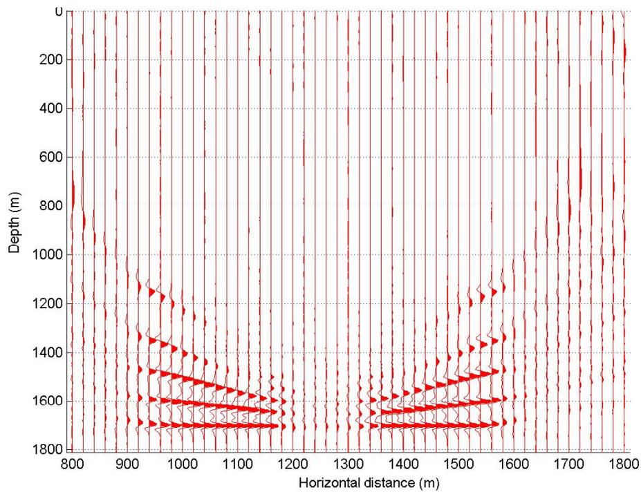
FIG. 8a. Migrated section (model 2) using shots every 400 m, from SP108 to SP120.
