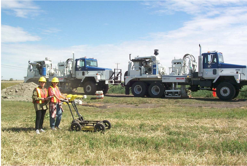
FIG. 1. Noggin plus 250 MHz and Smart Cart® near station 101 at the Calgary International Airport site. The two vertical vibrators used to shoot the seismic line are in the background.
