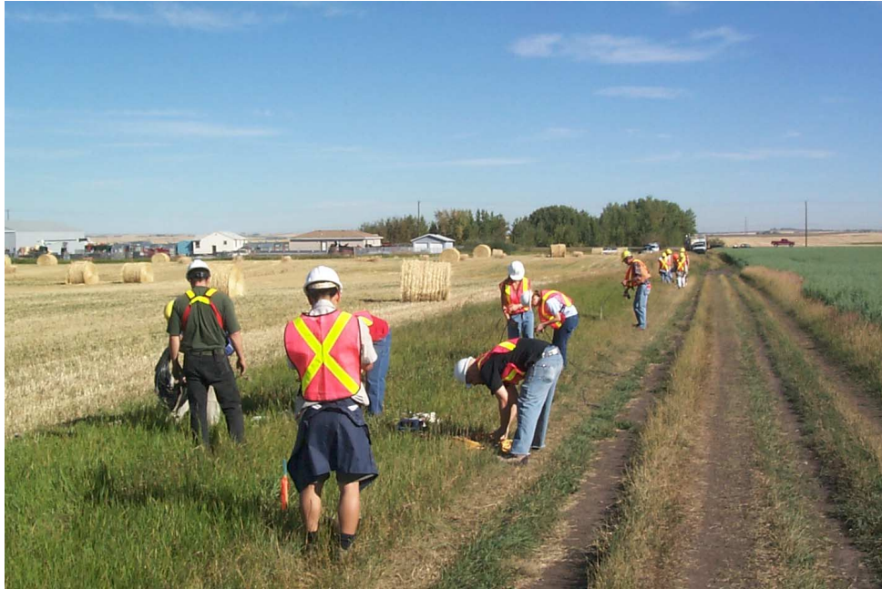
FIG. 2. North end of the 2.4 km seismic and GPR lines. Students deploy and plant 3-C geophones.
