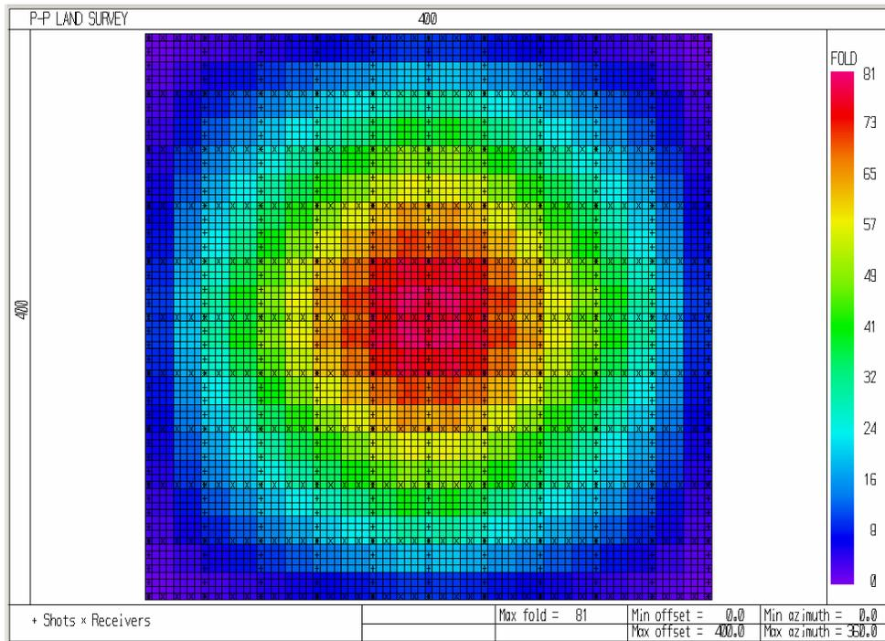
FIG. 8: P-P fold, coalbed methane 3C-3D seismic survey. Offsets up to 400 m.
