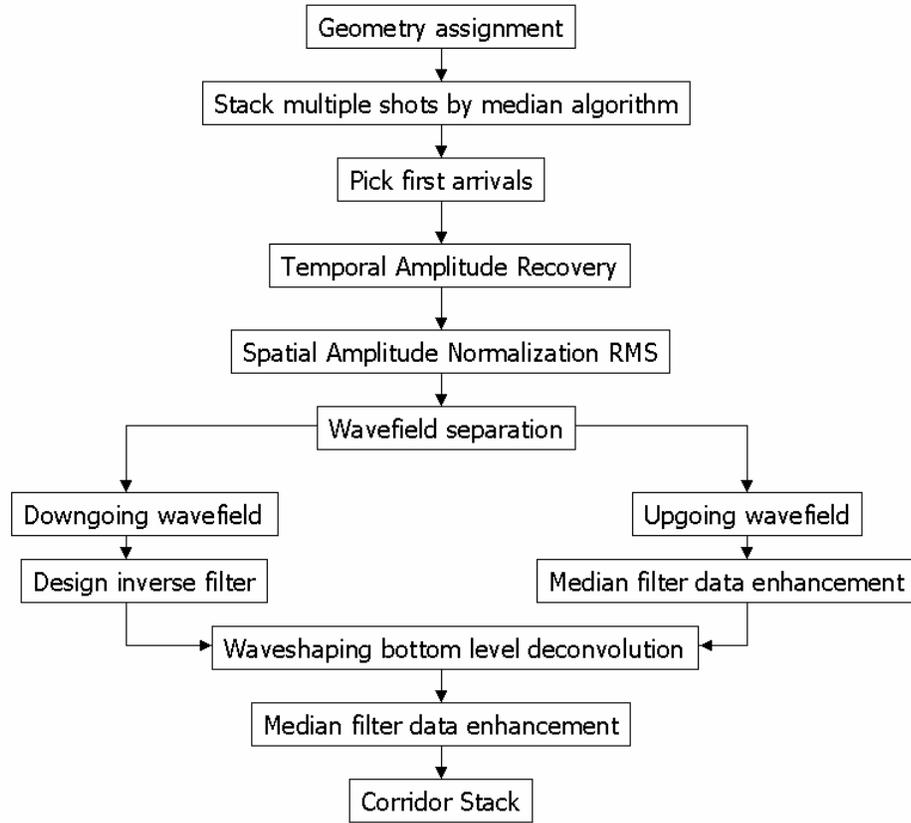
FIG. 5. Processing flow used to process zero-offset mini-P VSP data (Schlumberger).
