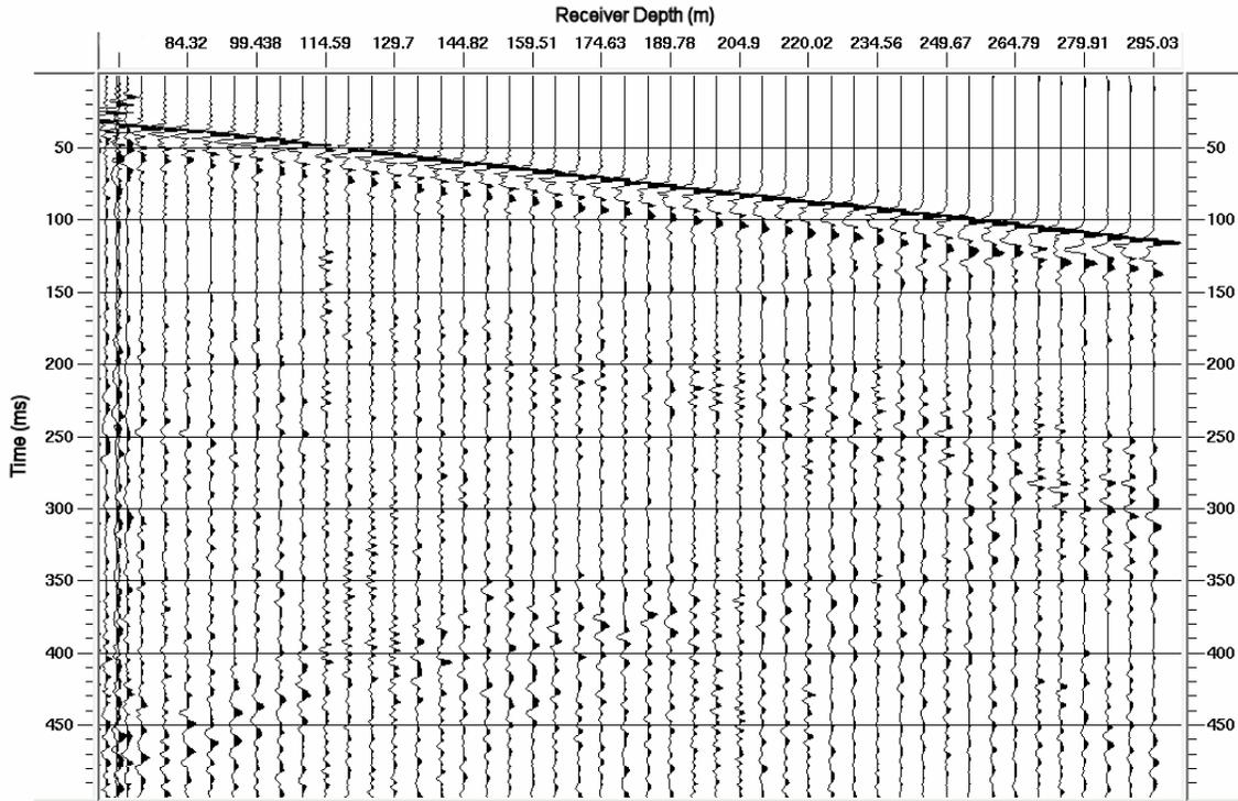
FIG. 2. Summed raw vertical-component data recorded for mini-P zero-offset vertical seismic profile at Red Deer. Automatic gain correction (200 ms operator length) applied.
