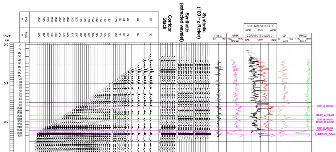
FIG. 6. Final corridor stack of upgoing P-wavefield from zero-offset mini-P data (Schlumberger).
