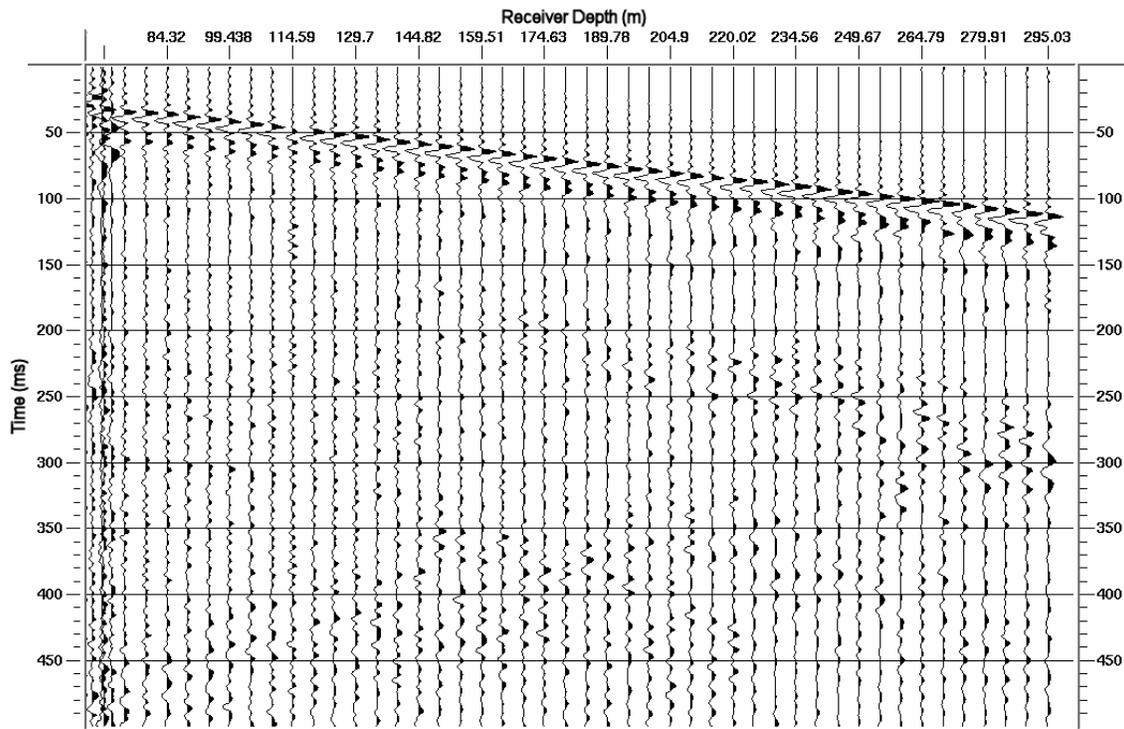
FIG. 3. Summed raw vertical-component data recorded for big-P zero-offset vertical seismic profile at Red Deer. Automatic gain correction (200 ms operator length) applied.
