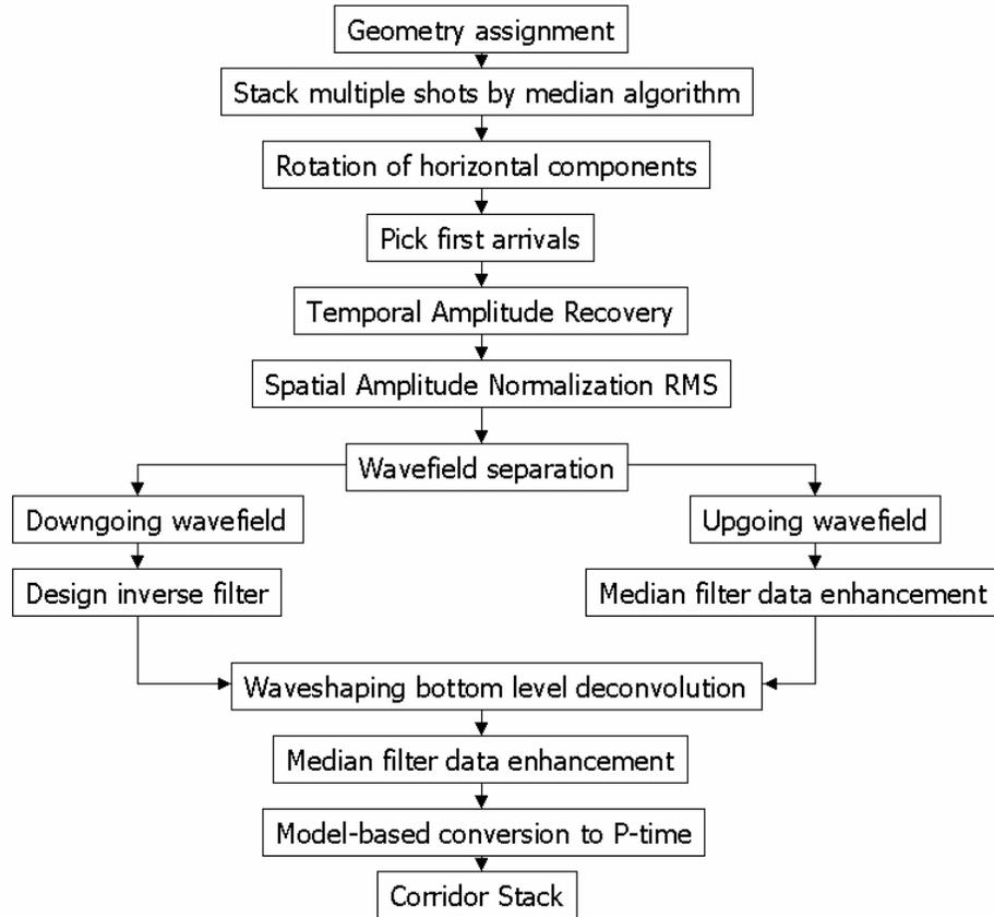
FIG. 8. Processing flow used by Schlumberger to process the zero-offset mini-S VSP data (Schlumberger).
