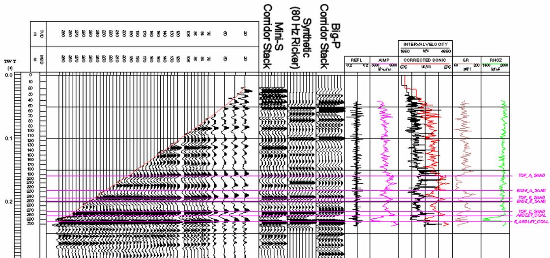
FIG. 9. Final corridor stack of upgoing S-wavefield from zero-offset mini-S data (Schlumberger).
