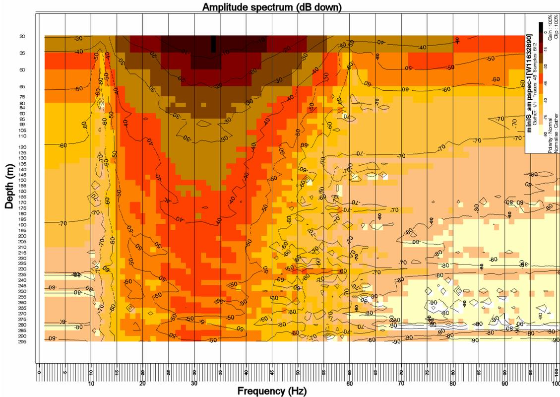
FIG. 13. Amplitude spectrum of raw zero-offset mini-S VSP data. Useable bandwidth ranges from 8-80 Hz (Schlumberger).
