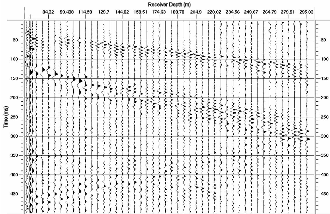
FIG. 4. Summed raw horizontal-component data recorded for mini-S zero-offset vertical seismic profile at Red Deer. Automatic gain correction (200 ms operator length) applied.
