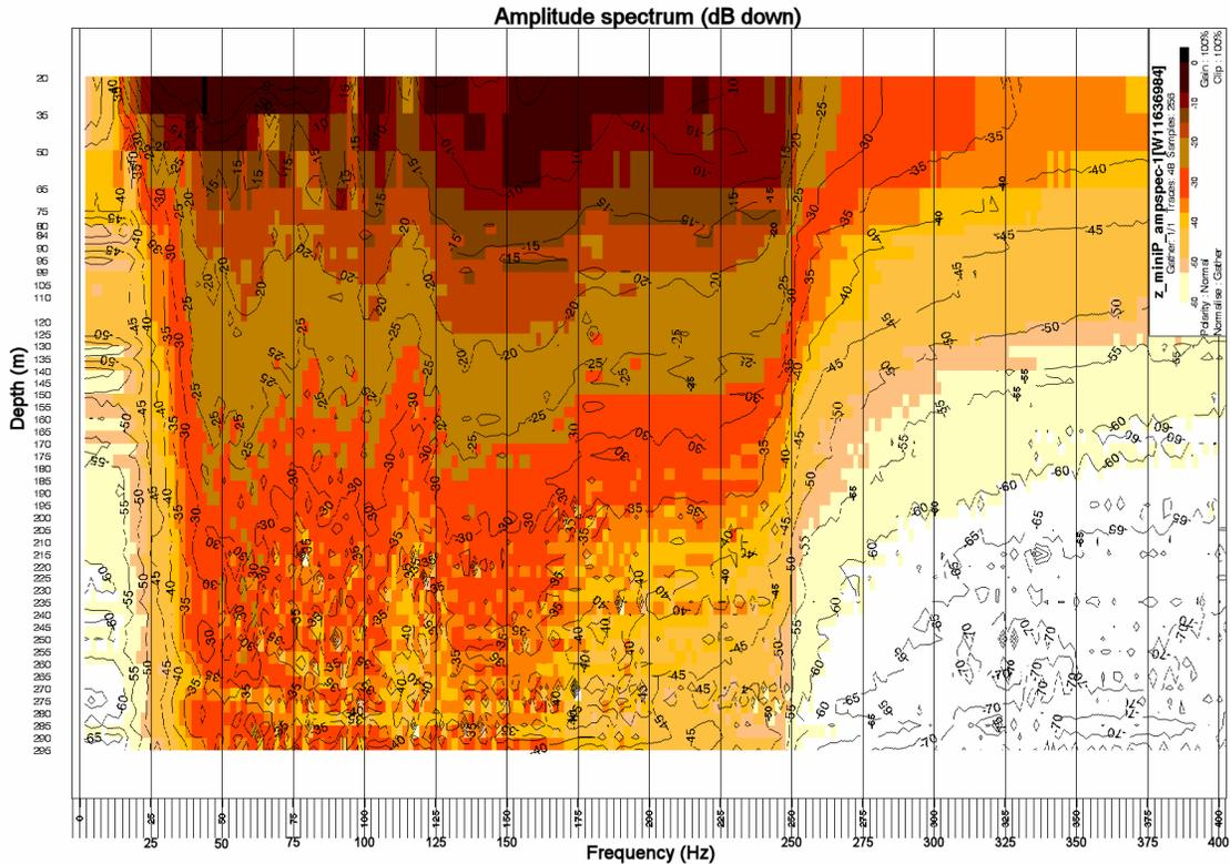
FIG. 12. Amplitude spectrum of raw zero-offset mini-P VSP data. Useable bandwidth ranges from 8-220 Hz (Schlumberger).
