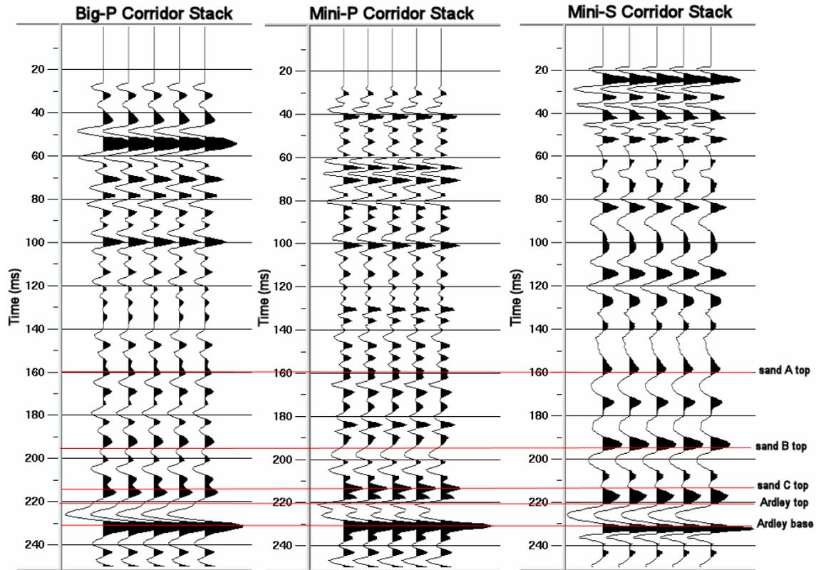
FIG. 10. Comparison of three final zero-offset corridor stacks. Improved resolution in the mini-P data set is immediately apparent.
