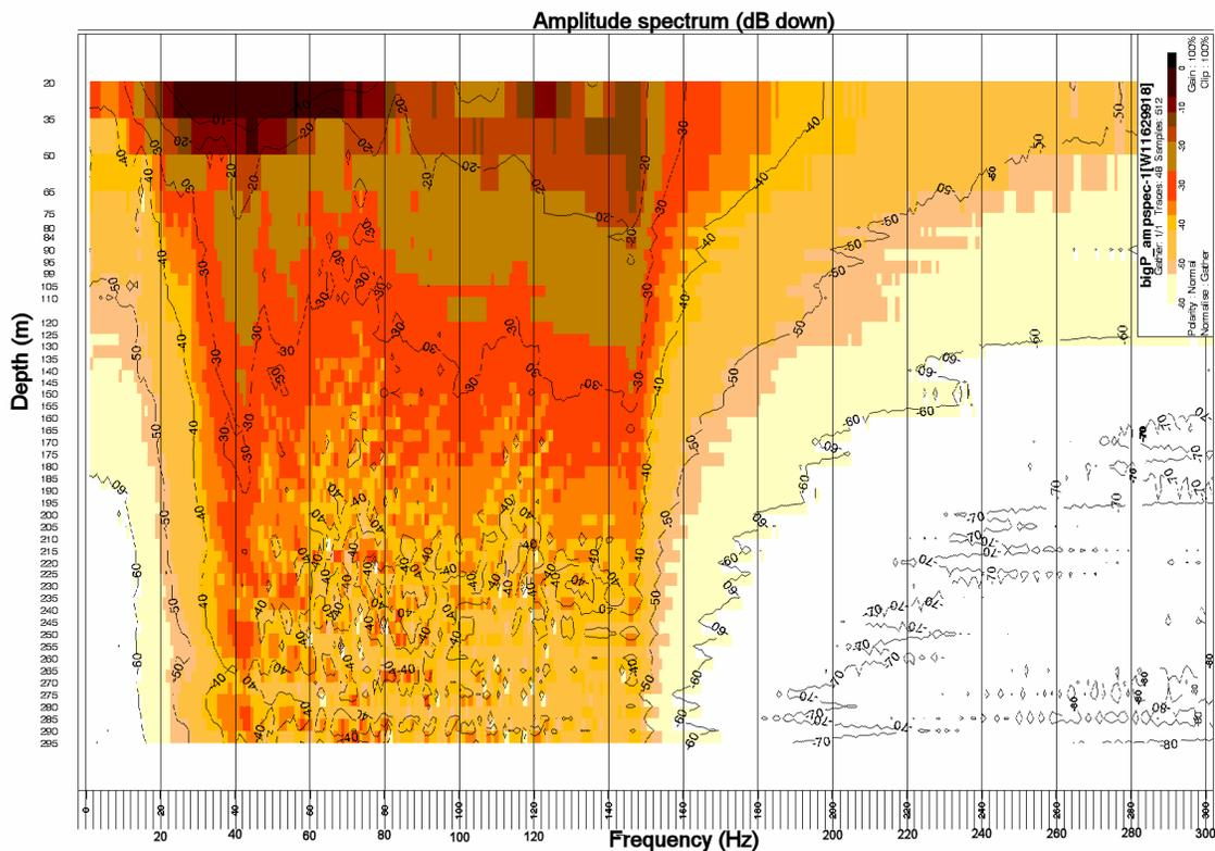
FIG. 11. Amplitude spectrum for raw big-P zero-offset VSP data. Useable bandwidth ranges from 15-150 Hz, with little attenuation of high frequencies, even at depth (Schlumberger).
