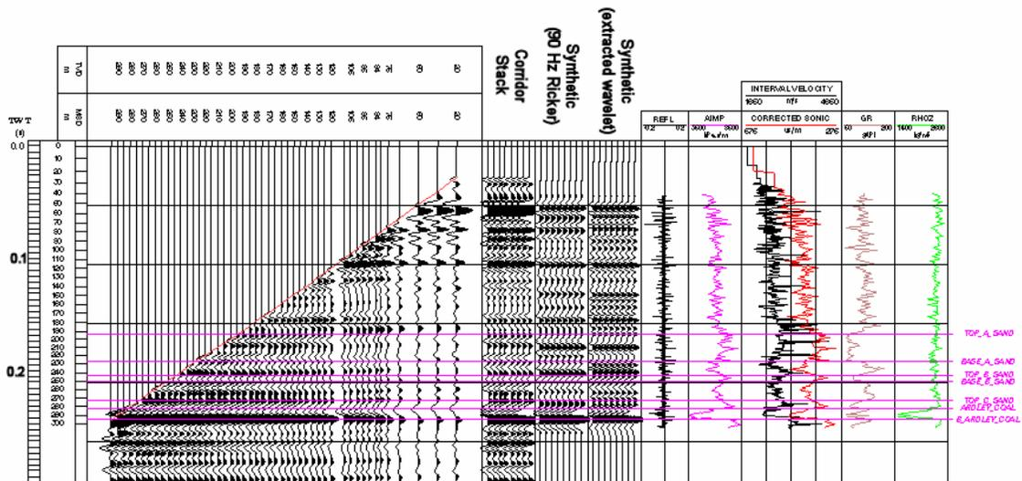
FIG. 7. Final corridor stack of upgoing P-wavefield from zero-offset big-P data (Schlumberger).
