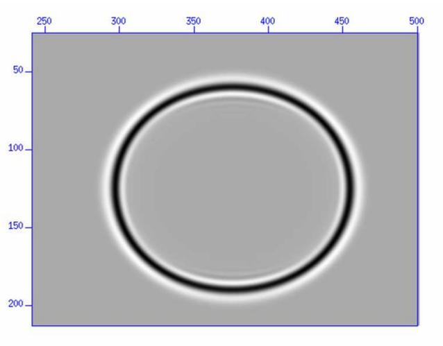
FIG. 1. Snapshot of the wavefront in medium with  $\epsilon = 0.2$  and  $\delta = 0.2$ .
