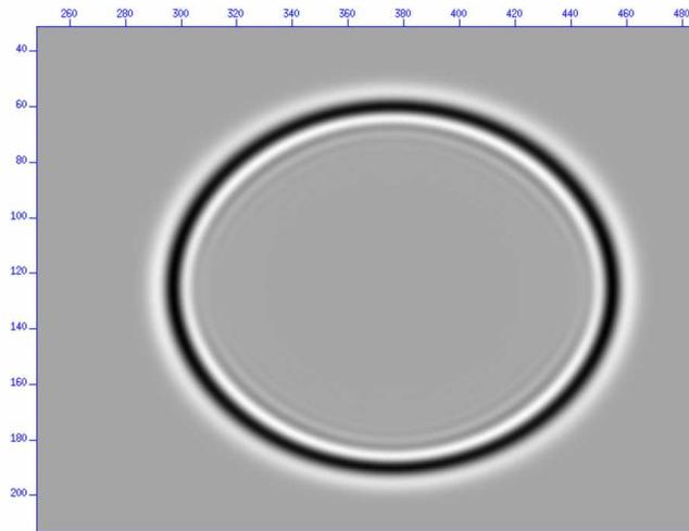
FIG. 3. Snapshot of the wavefront in medium with dip of  $\epsilon = 0.2$  and  $\delta = -0.2$ .
