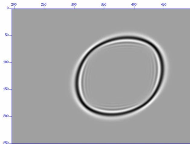
FIG. 6. Snapshot of the wavefront in medium with dip of 45°.
