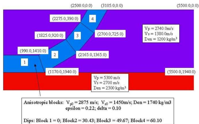
FIG. 8. Thrust sheet model (Courtesy Don Lawton).
