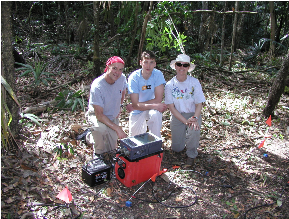
FIG. 4. Field crew (R. Stewart, N. Kaprowski, and J. Aitken) with Geometrics seismic recorder at the 3C-3D seismic micro-survey location in the plaza ruin.
