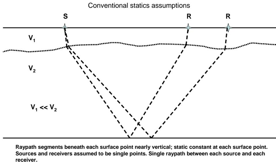
FIG. 1. Schematic showing the assumptions involved in the conventional statics model, which lead to the “surface-consistent” approach.
