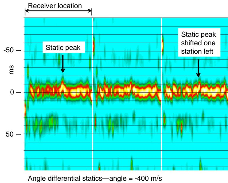
FIG. 8. Statics distribution functions for three consecutive common-angle gathers centred on -400 m/s. The prominent differential static flagged by the arrow in the left panel has shifted one station to the left on the right panel due to changed raypath angle between the two gathers.
