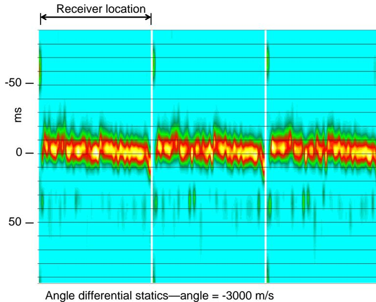
FIG. 6. Statics distribution functions computed for three consecutive common-angle gathers centred on -3000 m/s. These indicate differential statics shifts, from trace to trace, rather than absolute static shifts with respect to a pilot trace.
