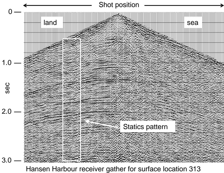
FIG. 3. A receiver gather from the Hansen Harbour 2D 3-C seismic survey. Data quality is much better on the portion of the gather where the shots were located on land rather than on floating ice. Note the pattern of static shifts outlined by the box.
