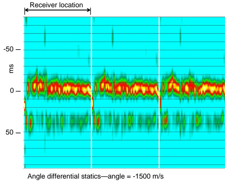
FIG. 7. Statics distribution functions for three consecutive common-angle gathers centred on -1500 m/s.
