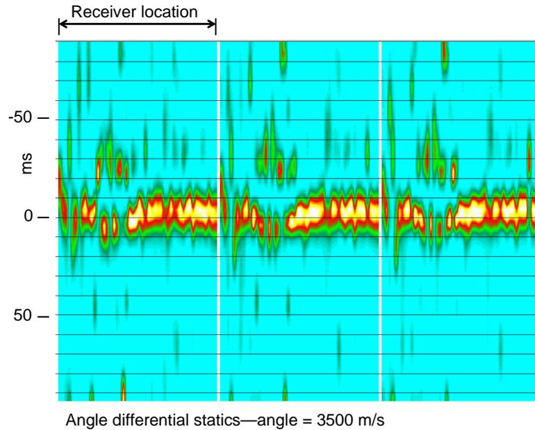
FIG. 11. Statics distribution functions for three common-angle gathers centred at 3500 m/s.
