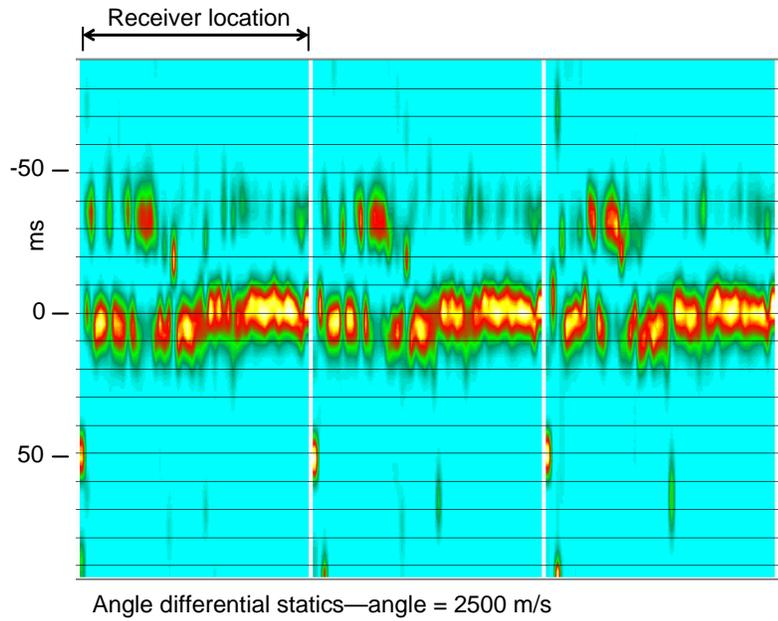
FIG. 10. Statics distribution functions for three common-angle gathers centred at 2500 m/s.
