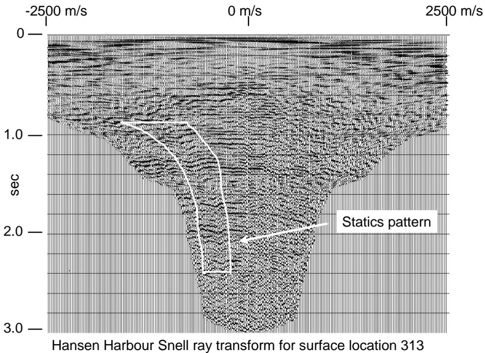
FIG. 4. Snell ray transform of the receiver gather shown in Figure 3. Each trace corresponds to seismic energy arriving at a single emergence angle at the surface.
