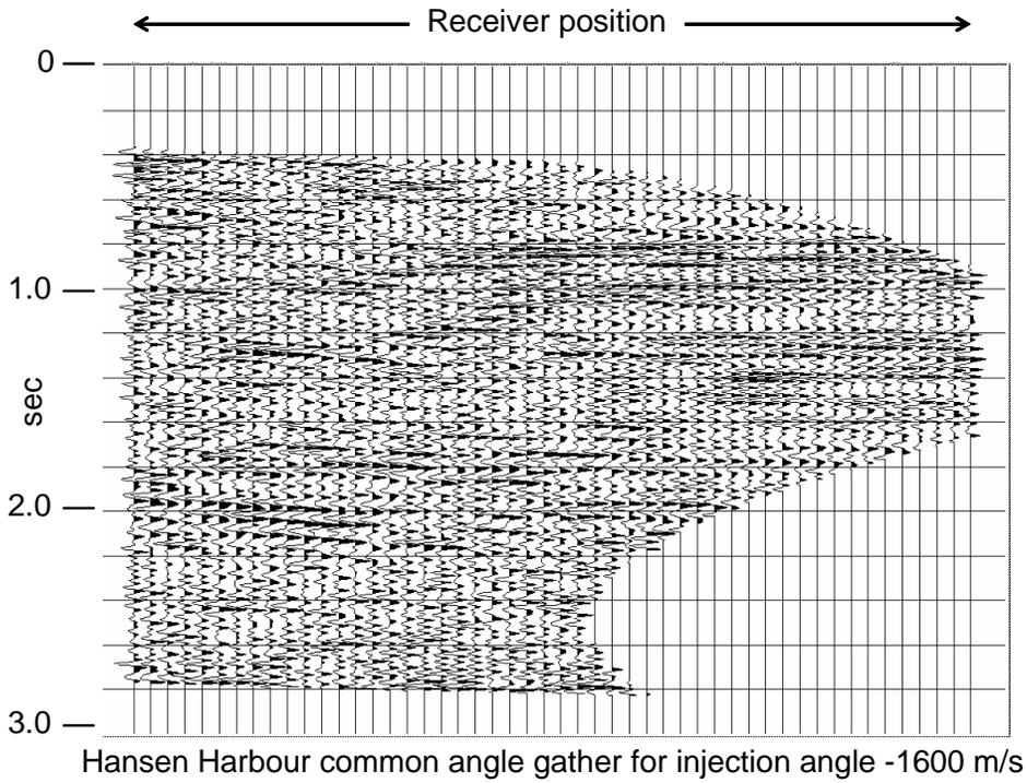
FIG. 5. A gather of Snell ray traces for which the emergence/injection angle is -1600 m/s. No large trace-to-trace statics are visible, but small ones can be seen.
