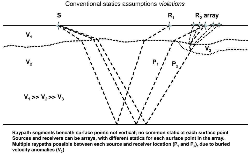
FIG. 2. Schematic showing some of the conditions which violate conventional statics assumptions.
