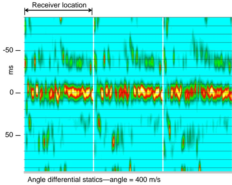
FIG. 9. Statics distribution functions for three common-angle gathers centred at 400 m/s.
