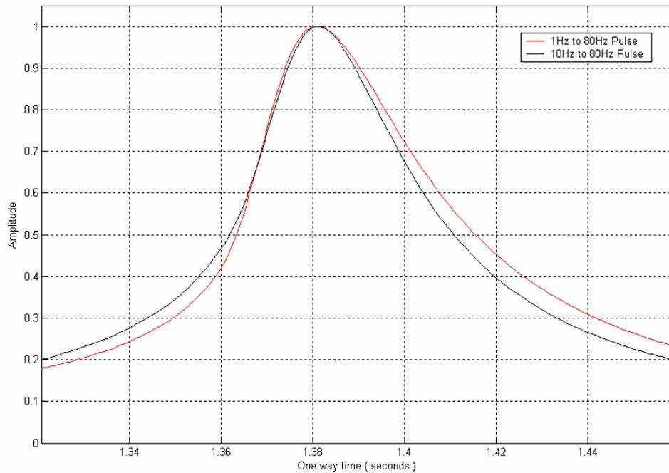
FIG. 2. Pulse comparison (aligned boxcar, 4000m depth, Q = 50).
