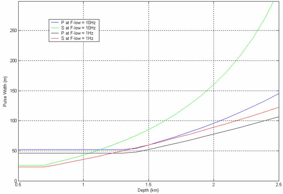
FIG. 3. -40dB noise floor  $\sin(x)/x$  resolution as function of depth ( $Q_P = 80$ ,  $Q_S = 40$ ,  $F_{max} = 80\text{Hz}$ ).
