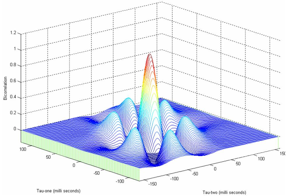
FIG. 5. Normalized auto-bicorrelation of signal without noise.
