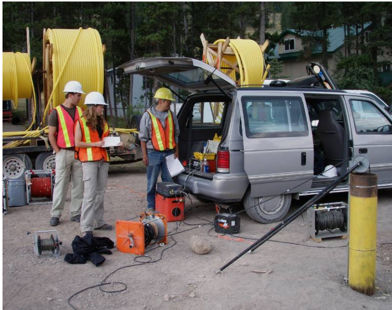
FIG. 12. Dr. Joe Wong of CREWES and assistants conduct a shallow VSP measurement using a 3C wall-clamped geophone tool.
