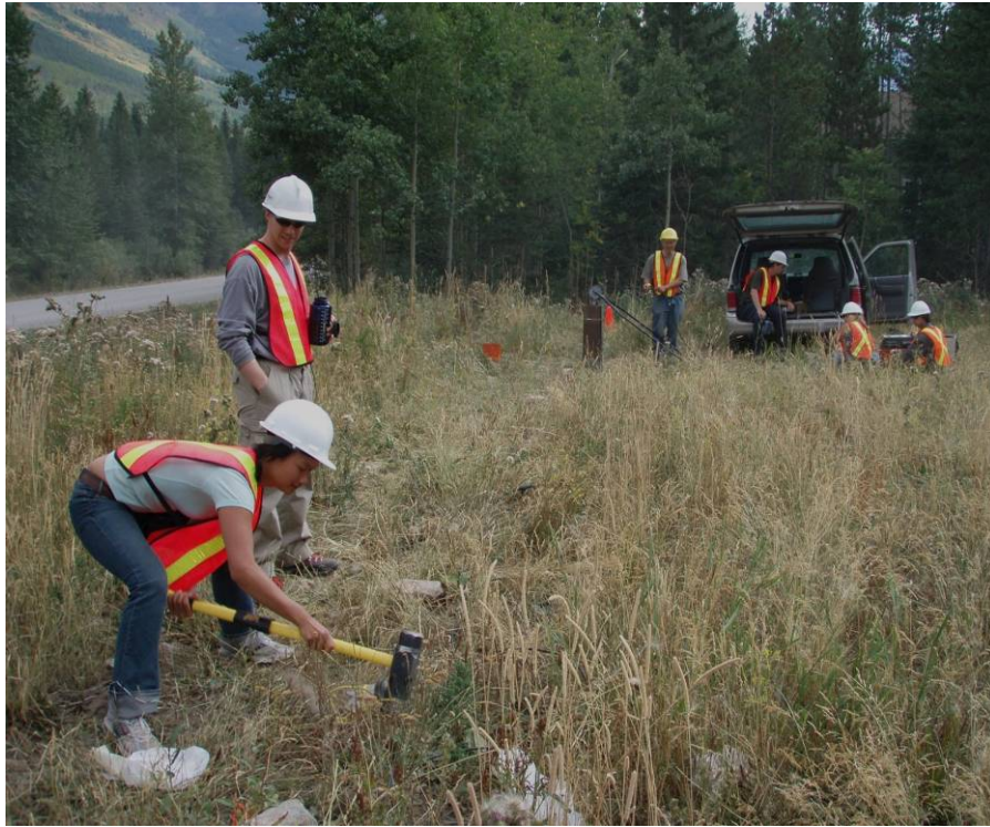
FIG. 13. Offset shallow VSP survey being conducted with a hammer-seismic source.
