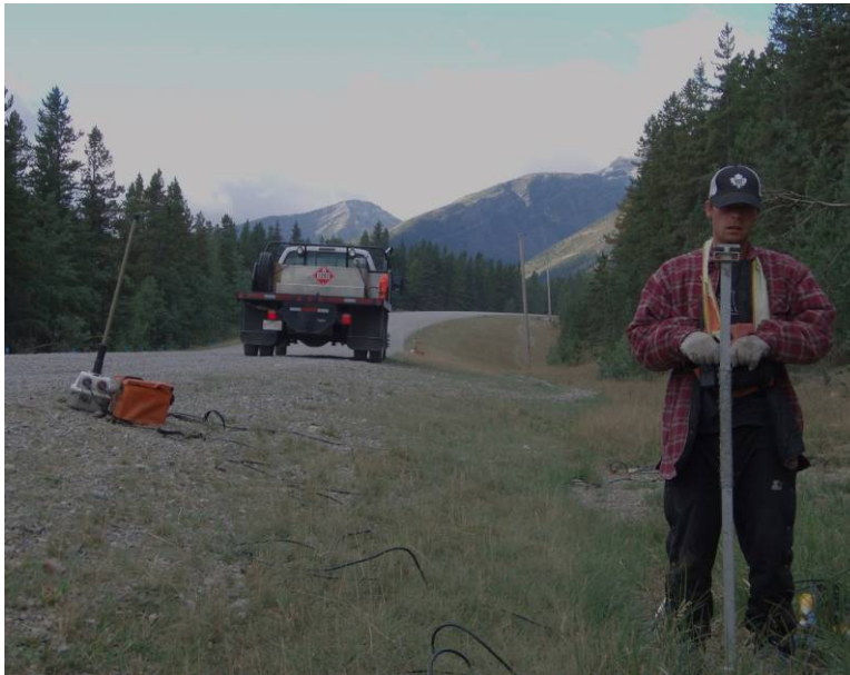
FIG. 8. Kinetex crewman orienting the digital 3C accelerometer. A VectorSeis cable-free telemetry box is seen in the left centre of the photo.
