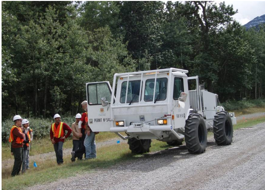
FIG. 7. The 17,000 lb. IVI vertical vibrator used as a seismic source in the ARAM and VectorSeis seismic lines.
