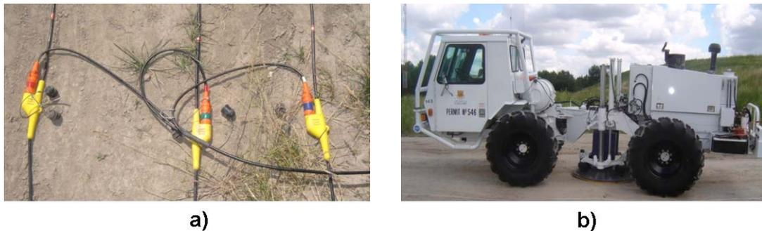
FIG. 6. Geophone cable connections were facilitated by using color codes for each component (left). Each Geode recorded a full dataset of a particular geophone component. The mini EnviroVibe, owned by the University of Calgary, was used as one of two seismic sources (right).
