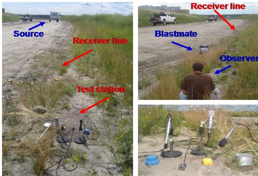
FIG. 3. Southwest view of the seismic line with the mini Vibe located at shot point one (left) and the seven-sensor test pad located at the northeast end (bottom right). The observer's computer was located about 3.5m north of the test station while the Blastmate monitor was located about 1 m east of the test station (top right) (Photos by first author).
