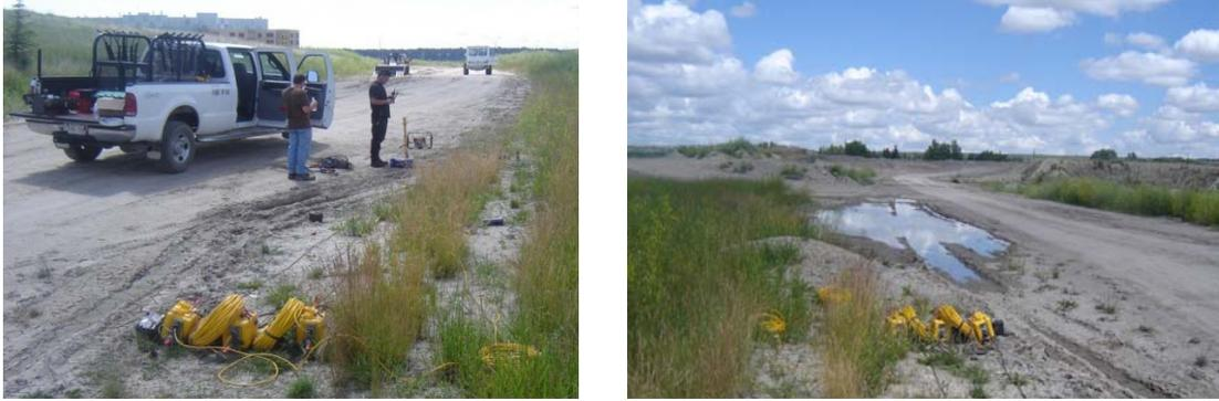
FIG. 7. CREWES staff preparing equipment (left) and north view of test site (right). The receiver line was deployed along the vegetation boundary to allow trafficking on the road.
