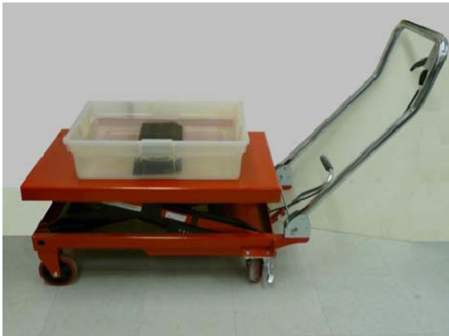
FIG. 13. Hand-operated hydraulic lift table for moving and positioning heavy models.
