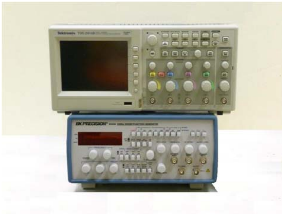
FIG. 10. Tektronix TDS 2014B digital oscilloscope for monitoring received signals (top); BK Precision 4040A signal generator for providing square control signal to activate MOSFET high-voltage switches (bottom).
