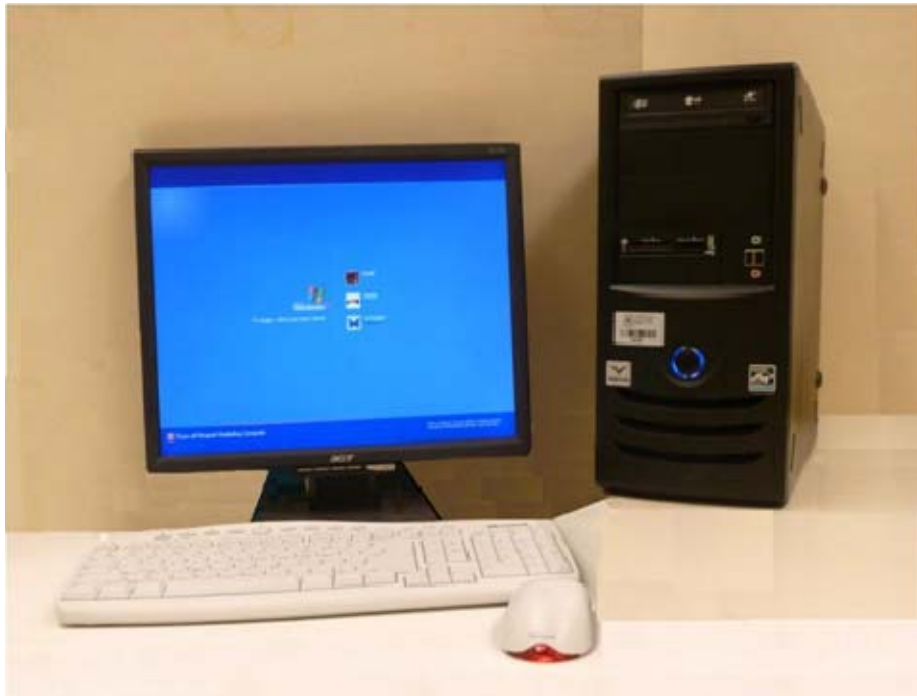
FIG. 12. System computer for motion control and acquisition. ACR-8020 and CS-1450 boards are installed inside the tower case.
