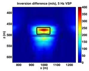
FIG. 8. The resulting VSP velocity estimate from inversion at 5 Hz, as a difference from the starting (background) velocity model. Ideally, the amplitude of the perturbation would be exactly +500 m/s. One wavelength at 5 Hz would approximately span this entire displayed region at the velocity of the target region. The black box marks the spatial extent of the actual perturbation.
