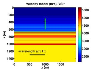
FIG. 2. Original velocity model plus steam-injection effect. The location of the VSP receivers is marked as a vertical green line at the injection site. The approximate wavelength at 5 Hz in the injected region is displayed for scale.
