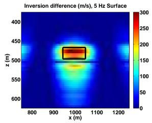
FIG. 6. The resulting surface-seismic velocity estimate from inversion at 5 Hz, as a difference from the starting (background) velocity model. Ideally, the amplitude of the perturbation would be exactly +500 m/s. One wavelength at 5 Hz would approximately span this entire displayed region at the velocity of the target region. The black box marks the spatial extent of the actual perturbation.
