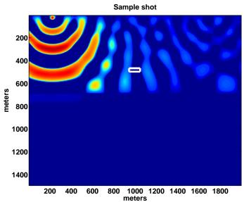
FIG. 5. Sample time slices of the forward-modelled data on the perturbed model. The white rectangle delineates the extent of the perturbation.
