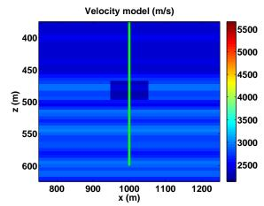
FIG. 3. Original velocity model plus steam-injection effect. The location of the VSP receivers is marked as a vertical green line at the injection site.
