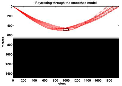
FIG. 4. Raytracing through the original model convolved with a 20 m Gaussian smoother
