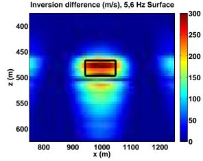
FIG. 7. The resulting surface-seismic velocity estimate from inversion at 5 Hz, as a difference from the starting (background) velocity model. Ideally, the amplitude of the perturbation would be exactly +500 m/s. One wavelength at 5 Hz would approximately span this entire displayed region at the velocity of the target region. The black box marks the spatial extent of the actual perturbation.
