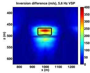
FIG. 9. The resulting VSP velocity estimate from inversion at 5 and 6 Hz, as a difference from the starting (background) velocity model. Ideally, the amplitude of the perturbation would be exactly +500 m/s. One wavelength at 5 Hz would approximately span this entire displayed region at the velocity of the target region. The black box marks the spatial extent of the actual perturbation.
