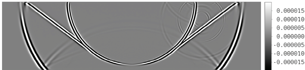
FIG. 6. A snapshot with a combined boundary of nonreflecting and absorbing at the bottom of the model, where N = 50 , and \varepsilon = 0.004 for the nonreflecting strip.
