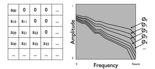
FIG. 1. Each column of the matrix represents a signal, with a Fourier amplitude spectrum. A plot of the spectra shows a decreasing sequence of functions.
