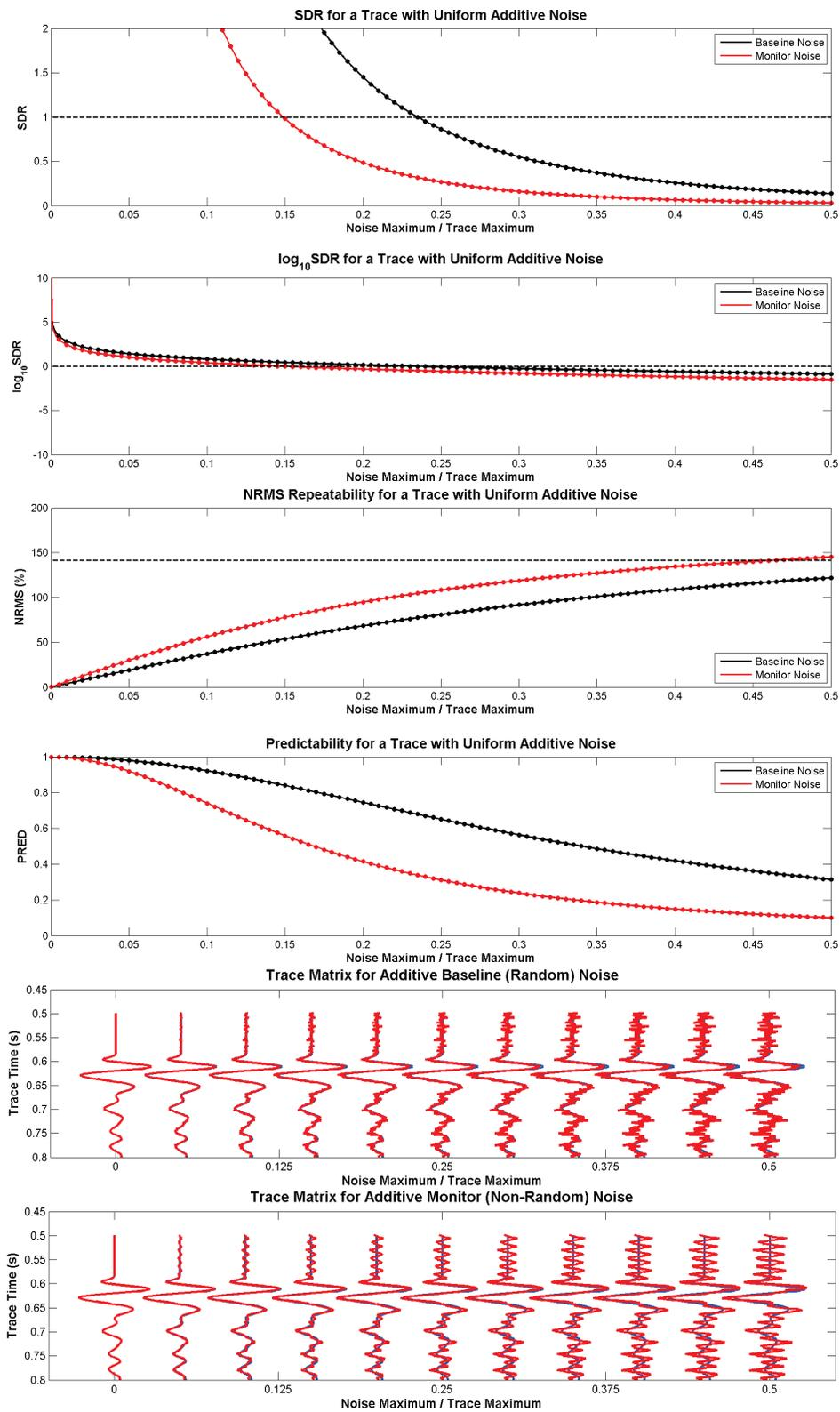
FIG. 5. From top to bottom: SDR,  $\log_{10}$  SDR, NRMS repeatability and predictability for additive noise experiment, showing addition of baseline (black) and monitor (red) noise. Two bottommost panels are wiggle displays of the noisy traces (red) overlapping the original trace (blue).
