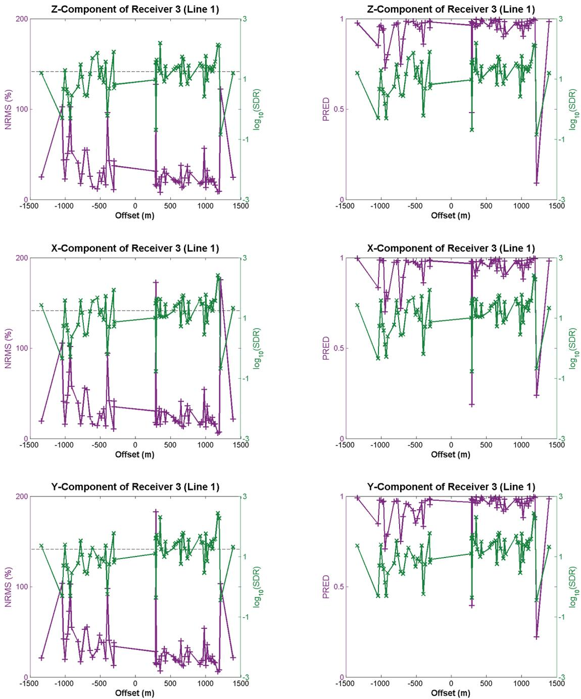
FIG. 7. Comparison of NRMS repeatability (left), predictability (right) and  $\log_{10}$  SDR of receiver 3 for Line 1. The z-component is shown at the top, x-component is shown in the middle, and y-component is shown at the bottom. The dashed line in NRMS plots indicates the theoretical noise line.
