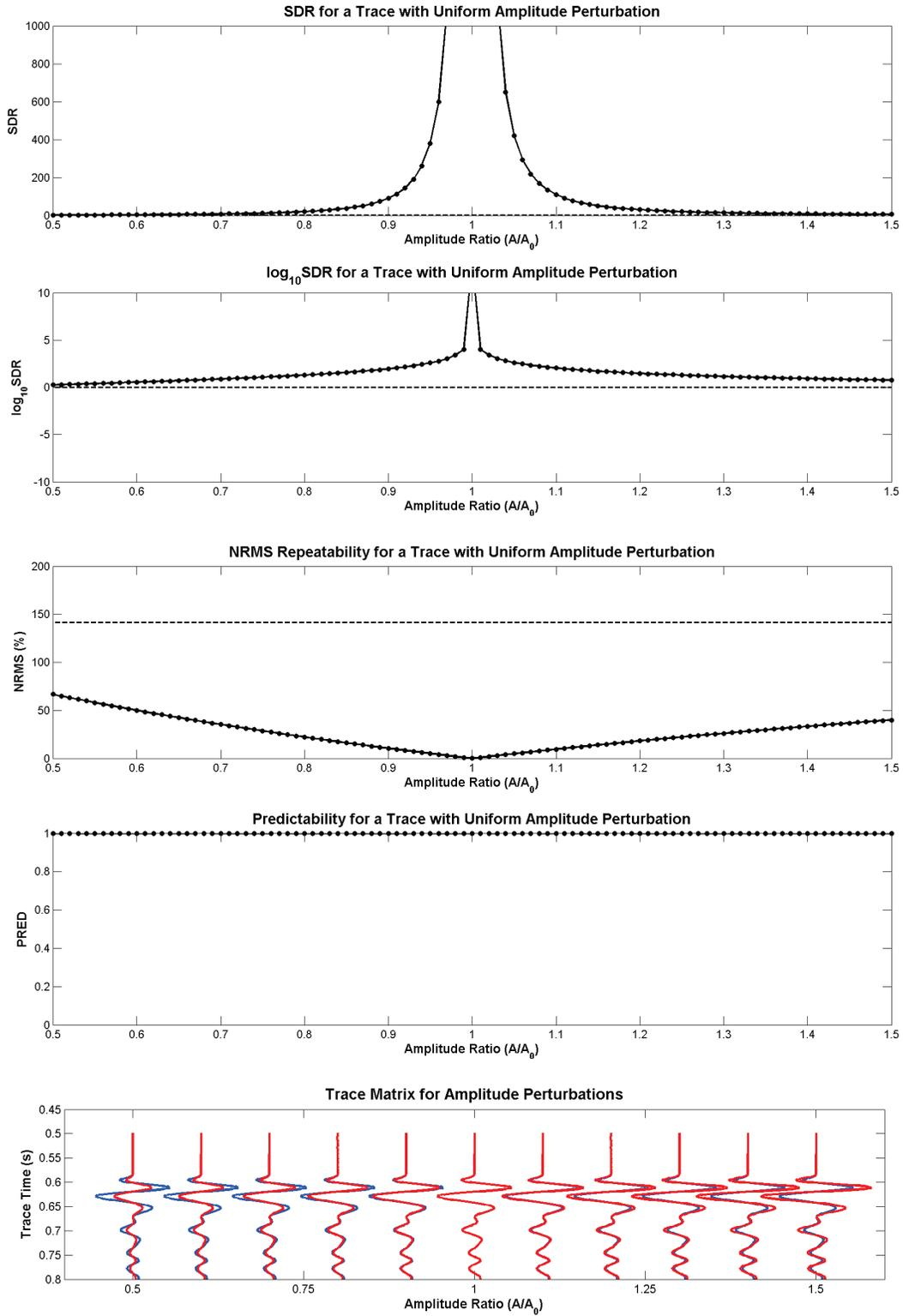
FIG. 4. From top to bottom: SDR,  $\log_{10}$  SDR, NRMS repeatability and predictability for amplitude experiment. Bottommost panel is a wiggle display of the amplitude modified traces (red) overlapping the original trace (blue).
