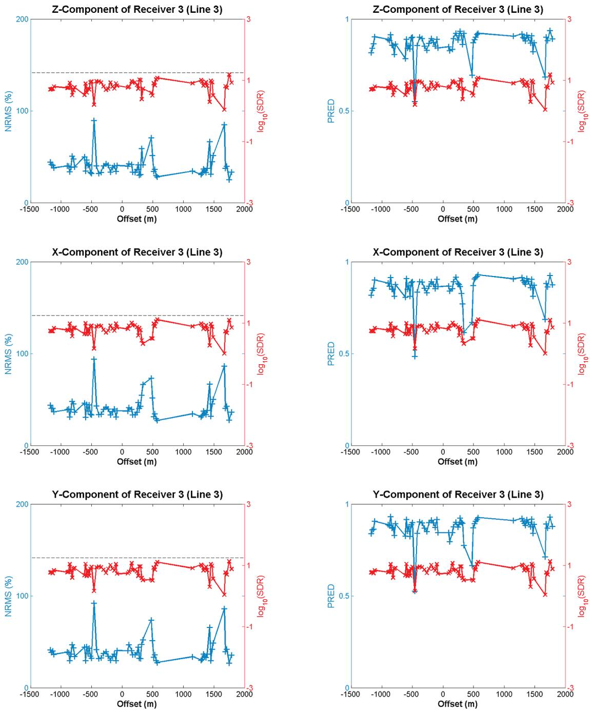
FIG. 9. Comparison of NRMS repeatability (left), predictability (right) and  $\log_{10}$  SDR of receiver 3 for Line 3. The z-component is shown at the top, x-component is shown in the middle, and y-component is shown at the bottom. The dashed line in NRMS plots indicates the theoretical noise line.
