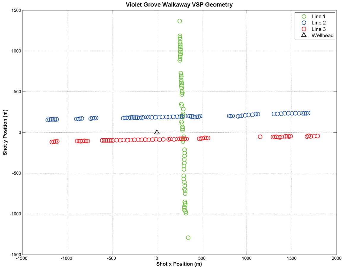
FIG. 1. Surface geometry for Violet Grove walkaway VSP used in this study.
