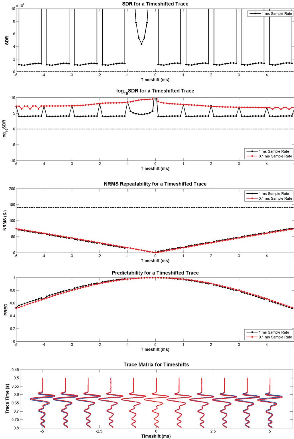
FIG. 3. From top to bottom: SDR,  $\log_{10}$  SDR, NRMS repeatability and predictability for time-shift experiment, showing traces left at the original sample rate (black) and traces resampled to 0.1 ms (red). Bottommost panel is a wiggle display of the time-shifted traces (red) overlapping the original trace (blue).
