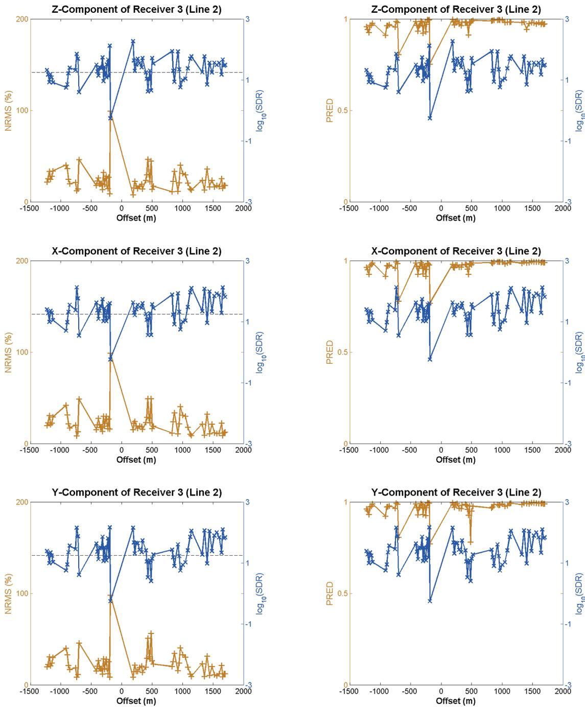
FIG. 8. Comparison of NRMS repeatability (left), predictability (right) and log<sub>10</sub> SDR of receiver 3 for Line 2. The z-component is shown at the top, x-component is shown in the middle, and y-component is shown at the bottom. The dashed line in NRMS plots indicates the theoretical noise line.
