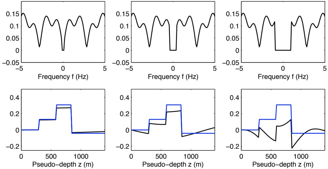
FIG. 1. Linear inverse scattering reconstruction of a two-layer medium with progressive loss of low frequency content. Top row: data spectra; bottom row: linear reconstruction at full bandwidth (blue) and with low frequencies removed (black). Left column: 0 Hz missing; middle column: 0-0.5 Hz missing; right column: 0-1 Hz missing.
