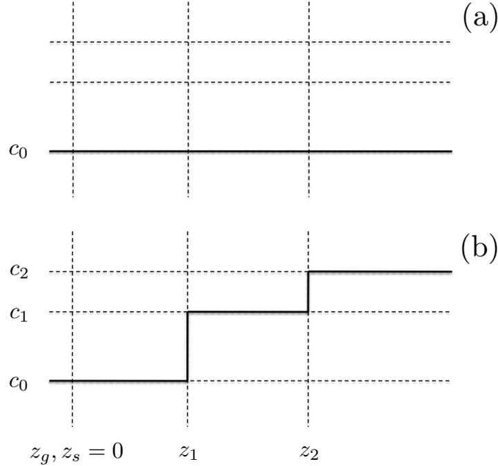
FIG. 2. Models used for analytic calculation of a single FWI iteration. (a) Initial, or background medium, a homogeneous wholespace with velocity  $c_0$ ; (b) The “actual” medium, consisting of two reflectors.
