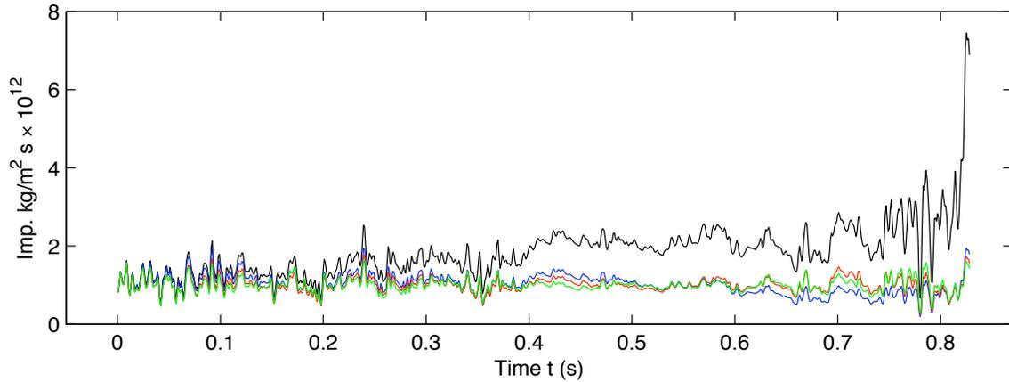
FIG. 4. Impedance inversion of reflectivity series estimated from Hussar well data at well 12-27. Black: full bandwidth; blue: lowest 1 Hz missing; red: lowest 5 Hz missing; green: lowest 10 Hz missing.
