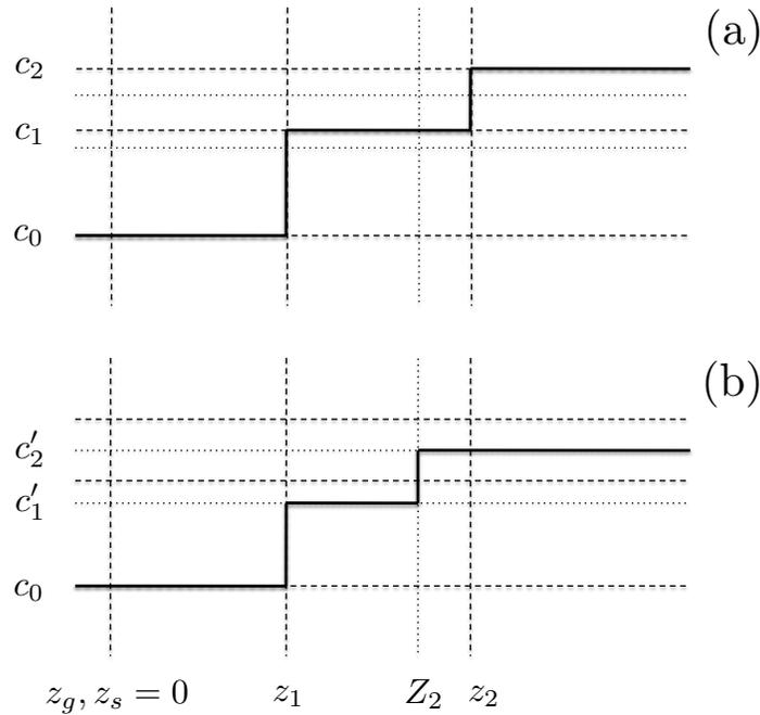
FIG. 3. True and estimated Earth models after iteration 1: (a) correct, or “actual” Earth; (b) FWI result. Two interfaces have been constructed, with error in the relative amplitudes and in the placement of any interface underlying Earth material *not* included correctly in the background model.
