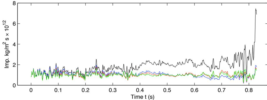
FIG. 4. Impedance inversion of reflectivity series estimated from Hussar well data at well 12-27. Black: full bandwidth; blue: lowest 1 Hz missing; red: lowest 5 Hz missing; green: lowest 10 Hz missing.
