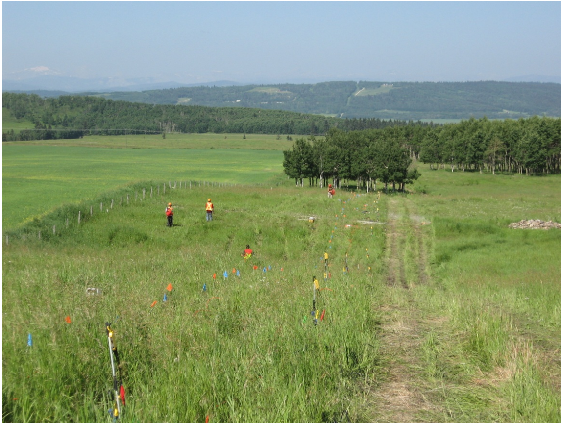
FIG. 2: Layout of the reflection seismic survey at Priddis. Flags show the geophone locations and the ruts show the route of the vibroseis truck.
