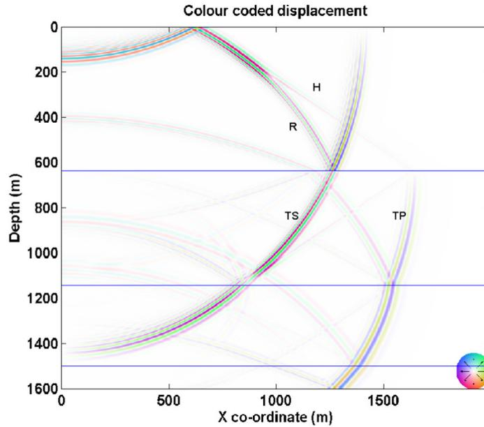
Figure 2: A snapshot of the computer model showing the wave fronts that will appear at the surface in Figure 1. The water bottom is at 635 m. R is the reflected wave, H is the head wave, TS is the transmitted shear, and TP is the transmitted pressure wave. The head wave has lower amplitude than the reflected wave.
