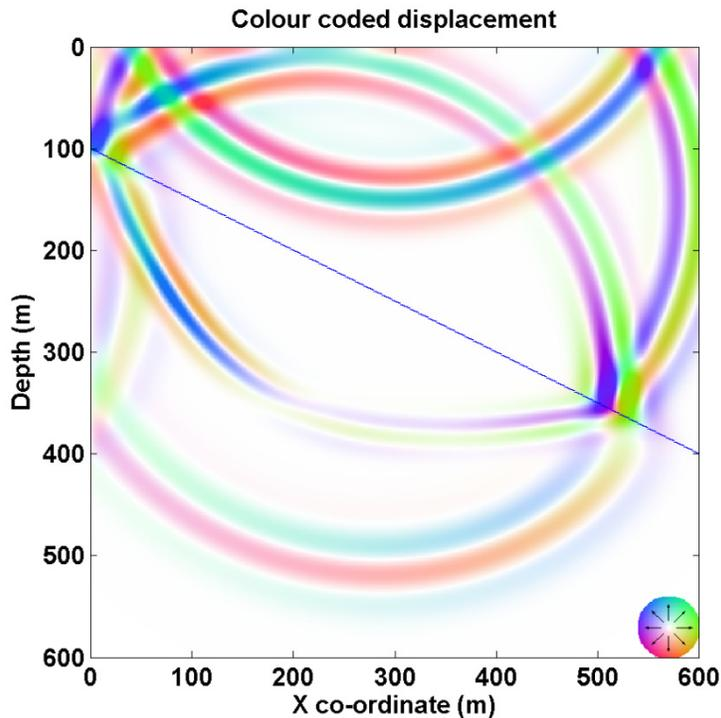
Figure 3: A snapshot of wave fronts from an explosive source in the water zone above the boundary which slopes down to the right. Note that above the boundary the wave fronts are simple arcs which were reflected from the surface and the boundary itself. Below is the elastic zone, where the waves are split into shear (slower) and pressure (faster).
