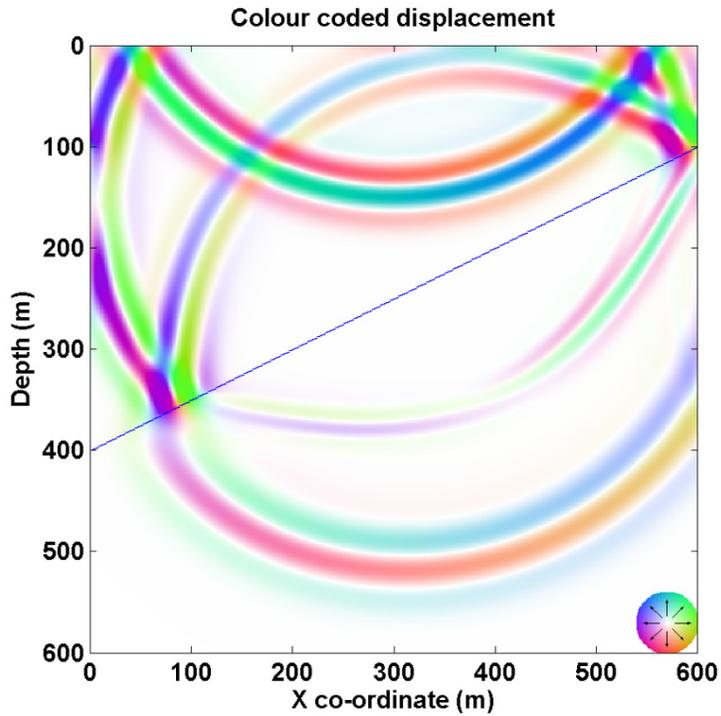
Figure 4: A wave fronts snapshot as in Figure 3, but with the boundary slope down to the left. The slope here is 50%
