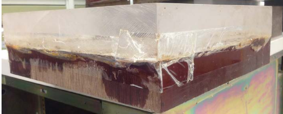
FIG. 4. A physical model consisting of a Phenolic layer under a Plexiglas layer, and representing a fractured reservoir overlain by isotropic overburden. Laboratory to field scale is 1:10,000 in both length and time. Scaled thicknesses of Plexiglas and Phenolic layers are 480 m and 450 m respectively.
