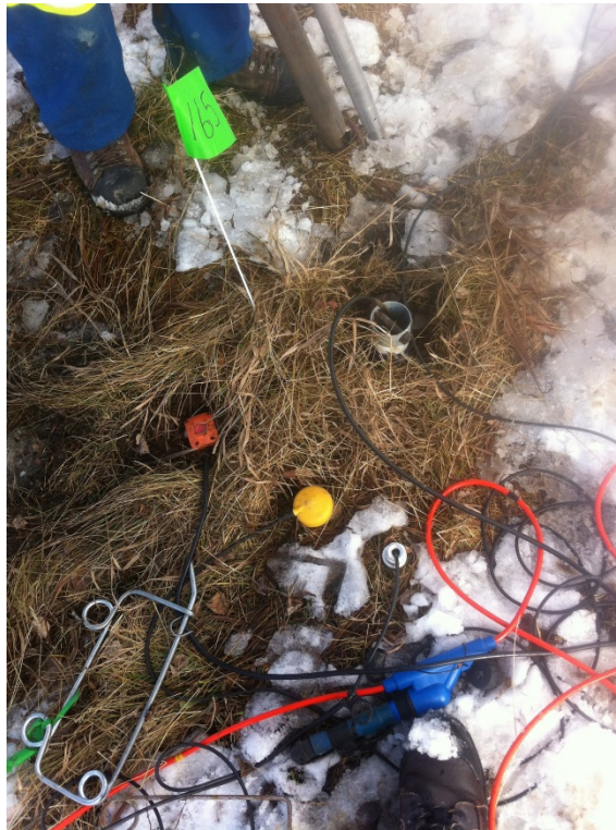
Figure 3: The sensors under test at station 165. The top of the ground screw appears slightly above and right of center. The comparable 3-component SM7 surface geophone is to the left in the orange case.
