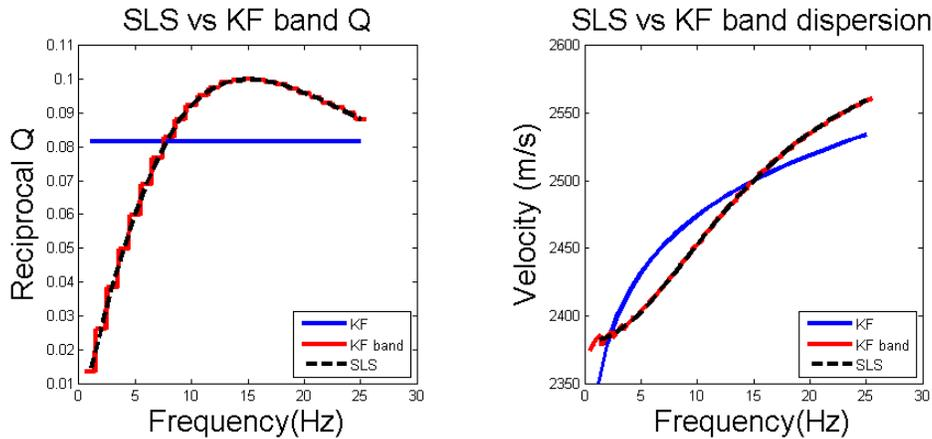
FIG. 2. Comparison of SLS with best fitting KF, and band-defined KF. Due to the highly dissimilar behaviour of the model types, the KF result is a poor approximation of the SLS behaviour. The band-defined KF is capable of matching the SLS behaviour much more closely, though still differs in dispersive behaviour on each band.
