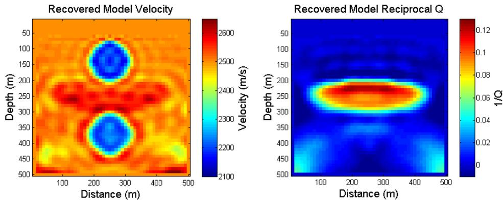
FIG. 8. Recovered velocity (left) and Q (right) using flexible KF FWI at 25Hz. Results compare favourably to true model (figure 4).
