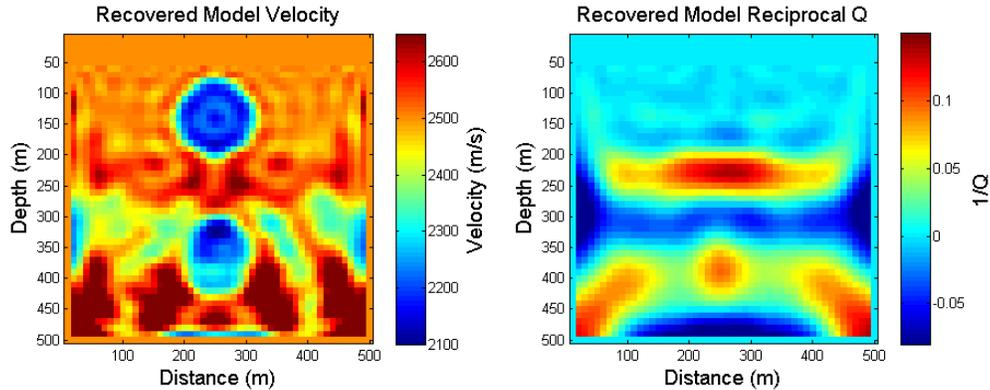
FIG. 6. Recovered velocity (left) and Q (right) using KF anacoustic FWI. Recovered velocity is inferior to that using acoustic FWI (figure 5).
