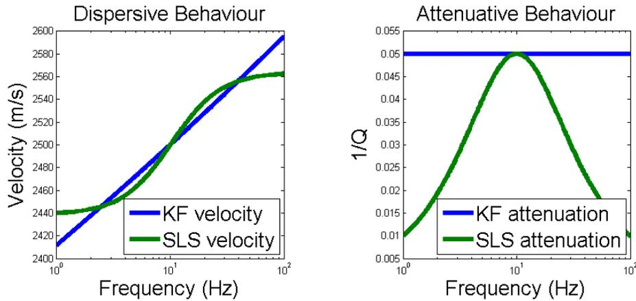
FIG. 1. Comparison of SLS and KF models for velocity 2500m/s at 15Hz and  $Q=20$ . Left: Velocity comparison. Right: Attenuation comparison. Note the semilog scale.
