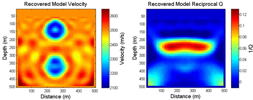
FIG. 7. Recovered velocity (left) and Q (right) using flexible KF FWI at 15Hz. Considerable improvements are evident in comparison to figure 6. Results compare favourably to true model (figure 3).
