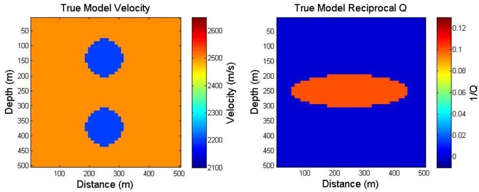
FIG. 3. True model velocity (left) and Q (right) for SLS model type at 15Hz.
