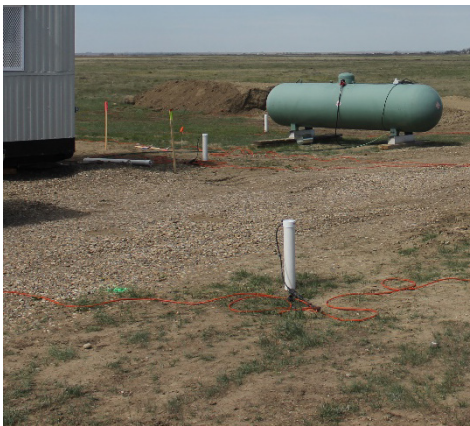
FIG. 8. A permanently installed geophone.
