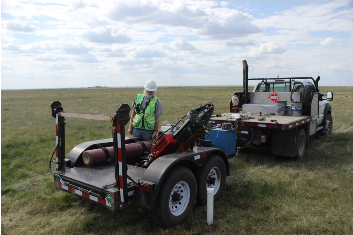
FIG. 6. The s-wave thumper source.
