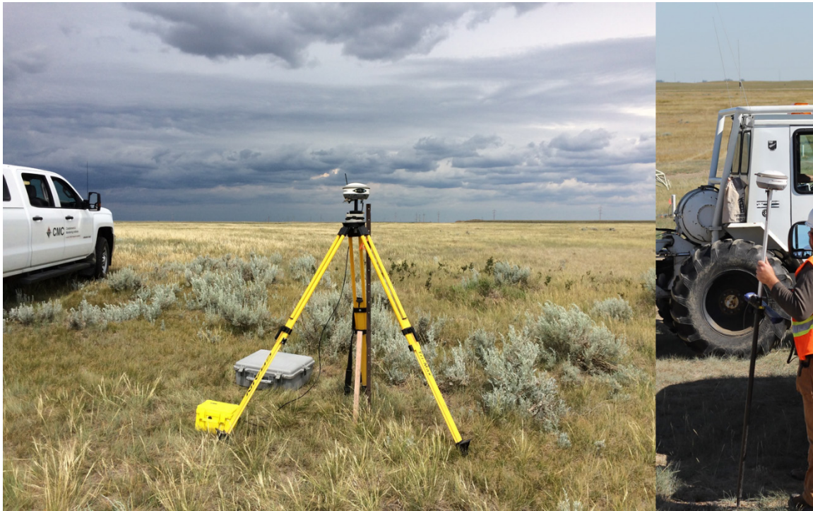
FIG. 7. The differential GPS, base station on the left, rover on the right.
