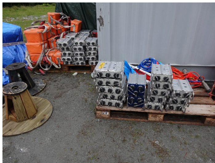
FIG. 2. Aries RAMS, taps, batteries, and cables ready for deployment.
