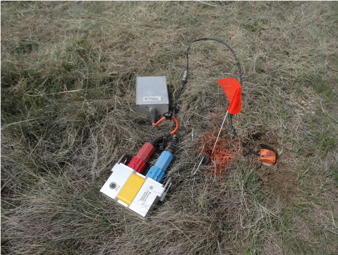
FIG. 3. A Hawk node, battery, and 3C geophone.
