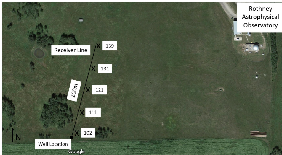
FIG. 2. Field location map. Source locations marked with X and source point number.
