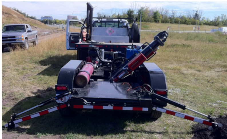
FIG. 1. CREWES Thumper source. Shown in S-wave generating mode, at 45° incidence.
