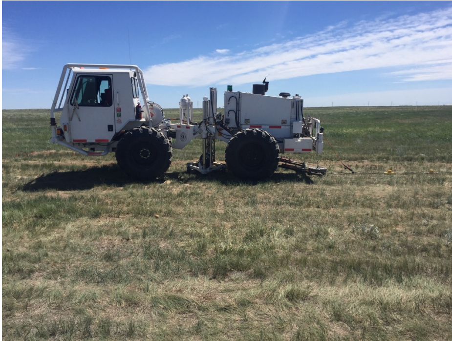
FIG 2. Echo Seismic Ltd.'s S-wave Envirovibe and land streamer.
