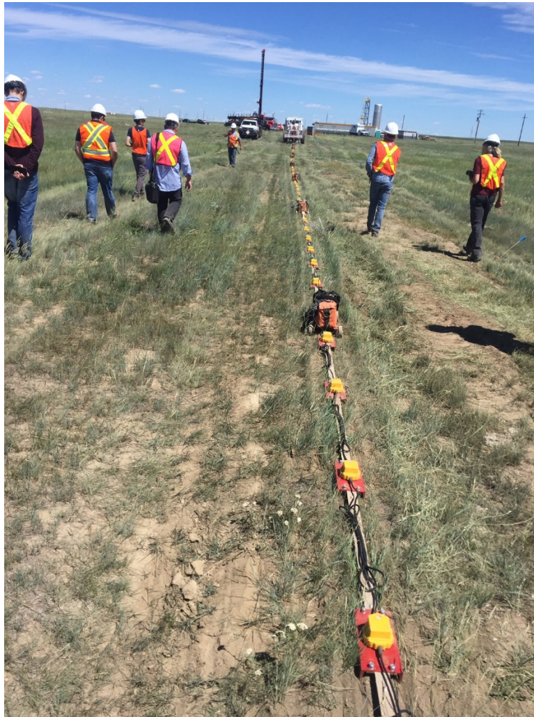
FIG 1. Echo Seismic Ltd. multicomponent land streamer.
