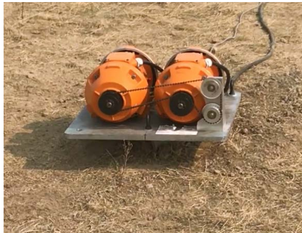
FIG. 3: GPUSA surface linear vibrator mounted on baseplate, attached to helical pile.
