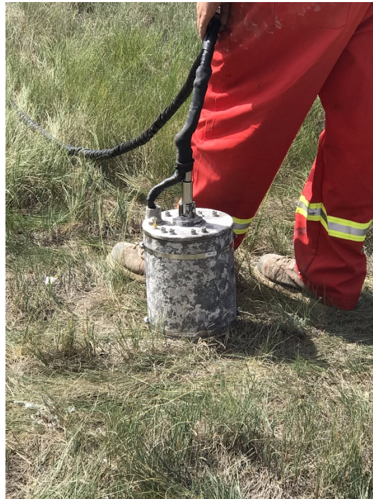
FIG. 2: GPUSA borehole linear vibrator prior to installation.
