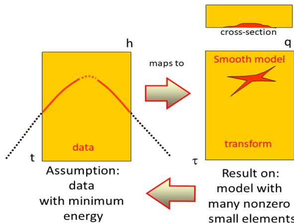
FIG. 3. Standard transforms principle:  $l_2$  norm inversion.
