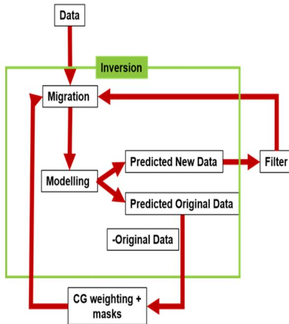
FIG. 12. A general flow for combining predictions from migration model with original data. Filter can include other processes, like 5D regularization or matching filters
