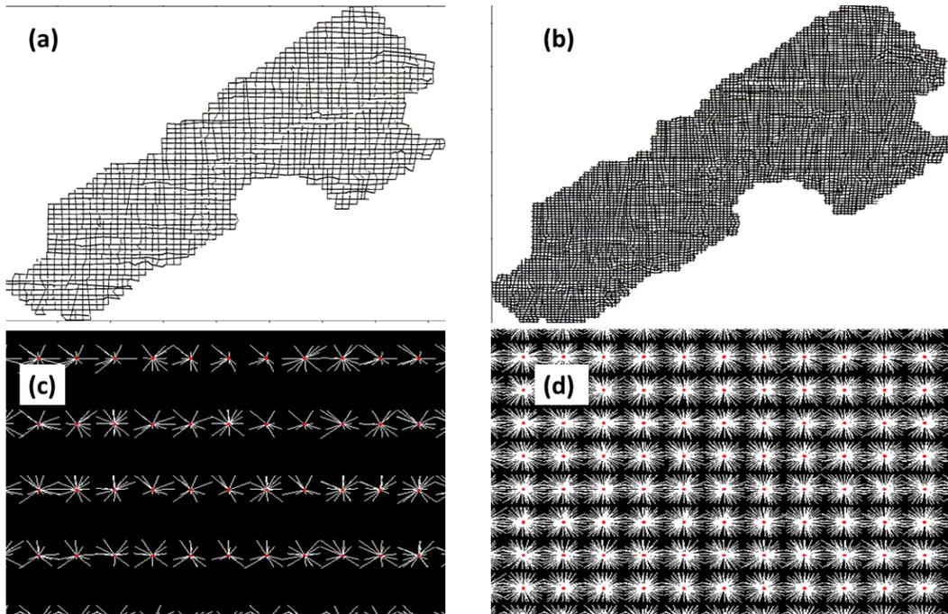
FIG. 5. A real 3D geometry plotted in acquisition coordinates a) before interpolation b) after interpolation. The same geometry plotted in interpolation coordinates c) before interpolation d) after interpolation
