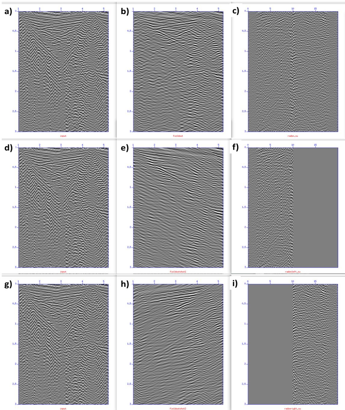
FIG. 12. De-blending of shots acquired by CREWES, (top row) both shots predicted by hybrid Radon transform, (middle row) first shot obtained by muting of right panel, (bottom row) second shot obtained by muting of first panel
