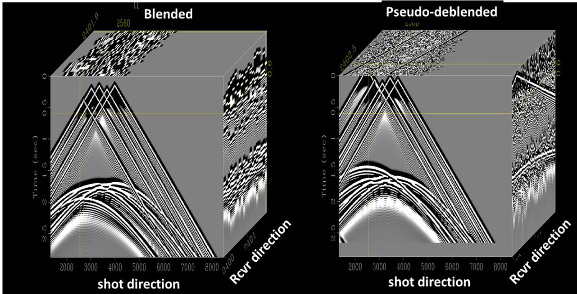
FIG. 4. Volume expansion produced by pseudo-deblending.
