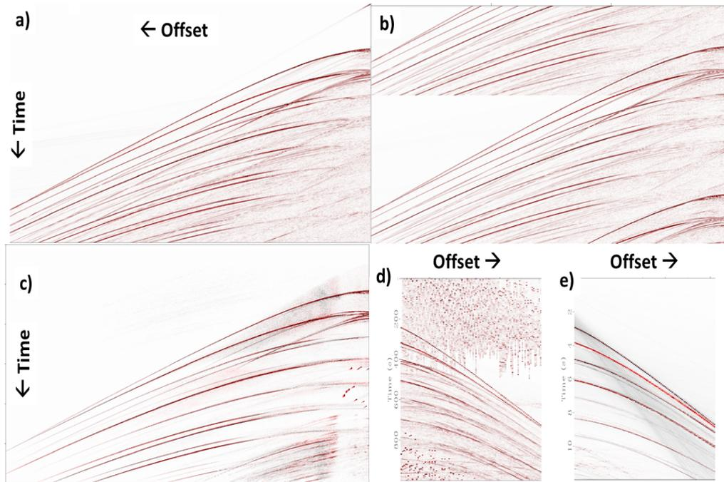
FIG. 10. Deblending by inversion in continuous recording in complex salt structure.
