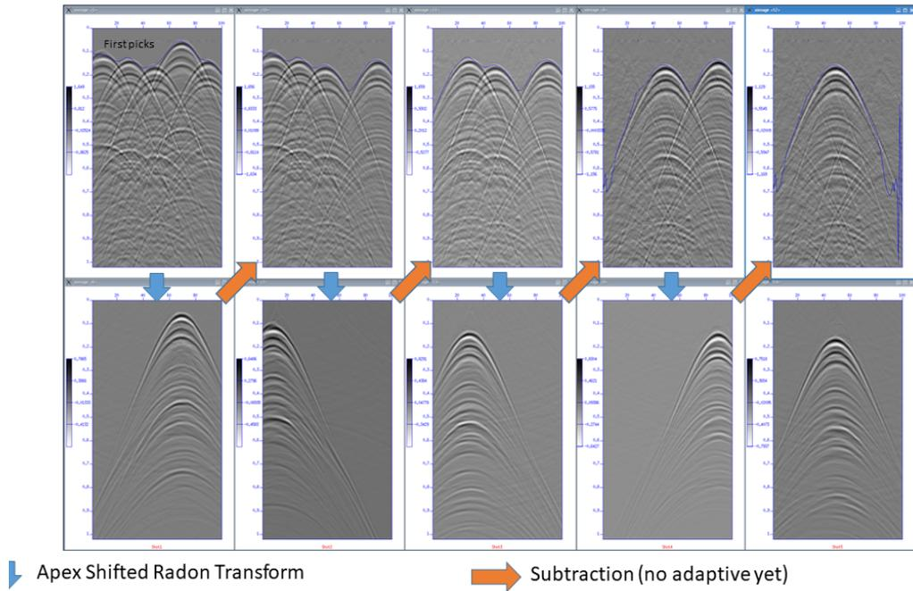
FIG. 14. A five-shot gather deblended by an Apex Shifted Radon Transform sequence
