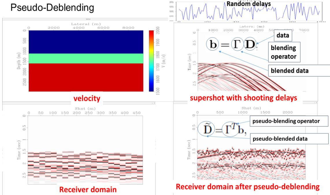
FIG. 3. When applying the pseudo-deblending operator, coherence is restored only for the particular shot whose delay is correctly compensated.
