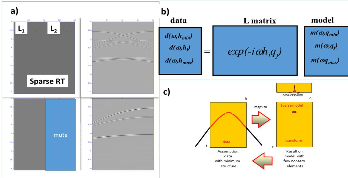
FIG. 11. a) Separation of shots without time dithering. Left, synthetic example where two different operators are used to separate the events. Upper right) Schematics of the Radon frequency domain operator illustrating its dependence on the offset. Bottom right) sparseness principle
