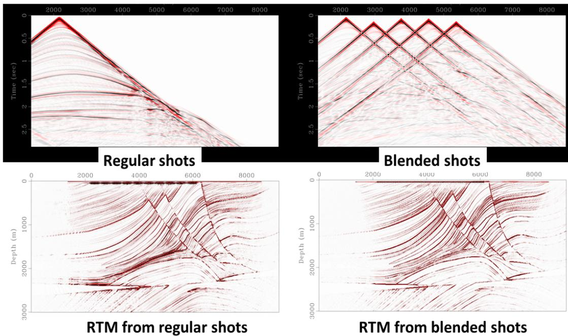
FIG. 15. First column, regular data migrated by RTM. Second column) Five-shot blended data migrated by LSRTM.
