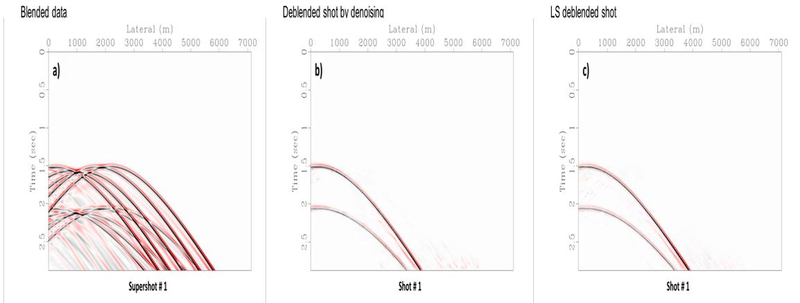
FIG. 7. Deblending by denoising and inversion techniques: a) One supershot (5 blended shots), b) One shot separated by denoising, c) The same shot separated by inversion.
