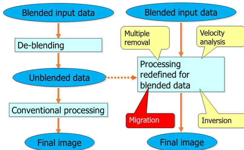
FIG. 2. Two different approaches for blended data processing (Verschuur, 2011).
