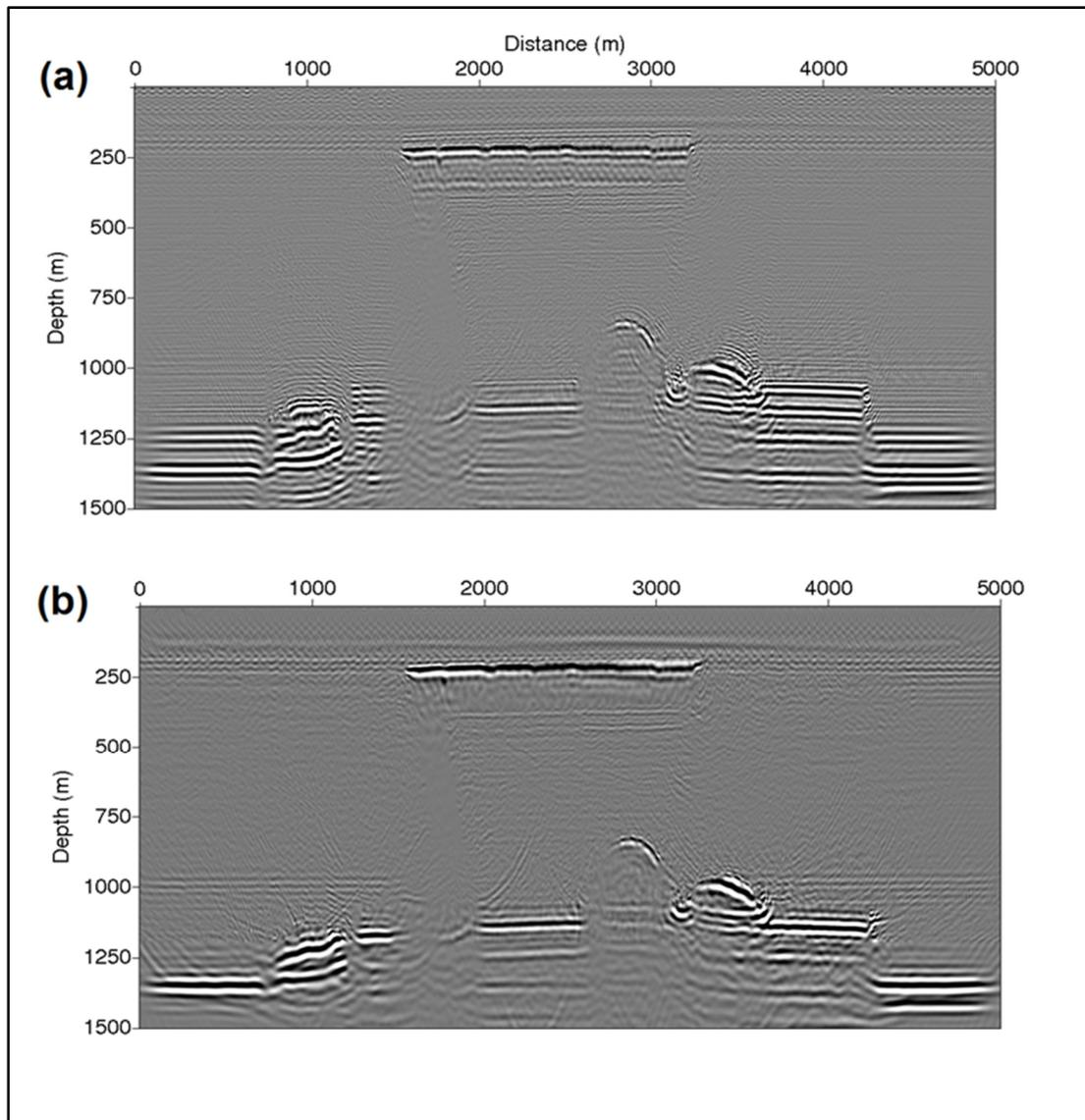
Figure 6: (a) Depth-migrated images produced with surface-only data before multiple suppression. Fictitious layers are present at the base of the model. They can be eliminated by muting amplitudes below 1800ms in all seismograms. (b) Depth-migrated image after suppression of multiples. In both cases, the dike, the bottom boundary of the sill, and the deeper targets are not well imaged.
