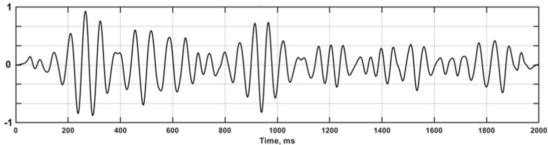
Figure B1: A possible source signature produced by a drill-bit interacting with rock.
