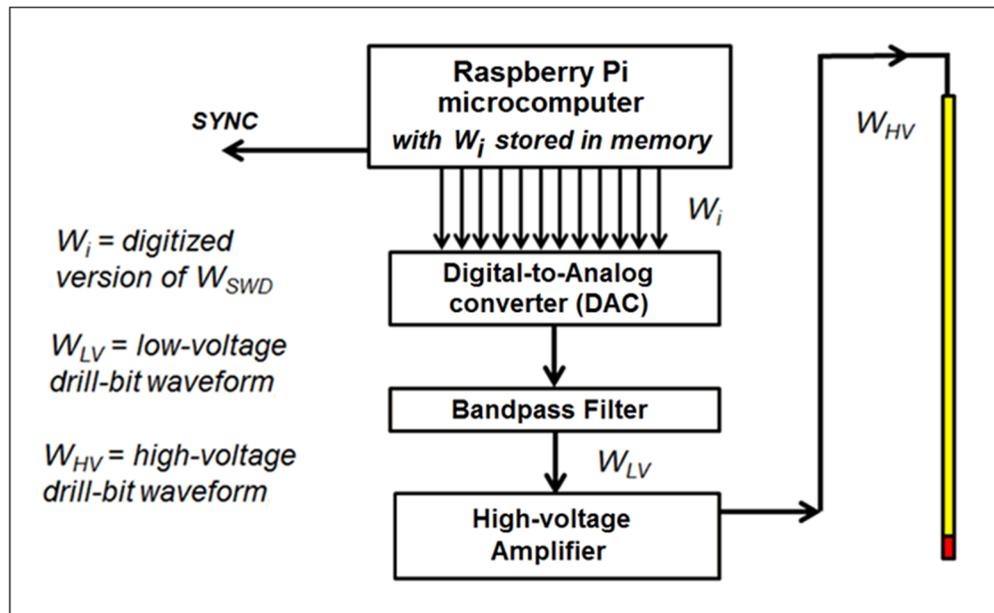
Figure A2: Schematic diagram showing an electronic design for producing high-voltage waveforms for driving a piezopin source transducer (shown in yellow). The SYNC signal is needed for synchronized stacking of received seismograms.
