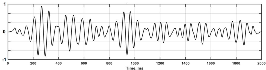
Figure A1: A possible source signature produced by a drill-bit interacting with rock.
