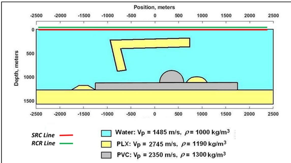
Figure 1: A physical model for studying seismic illumination, showing surface-only sources and receivers. The high-velocity sill-and-dike body acts as a blocking structure. The x-coordinate of all sources and receivers are nominally 0m, and all survey lines run along the y-axis. The water-air interface is about 1350m above the source and receiver survey lines.
