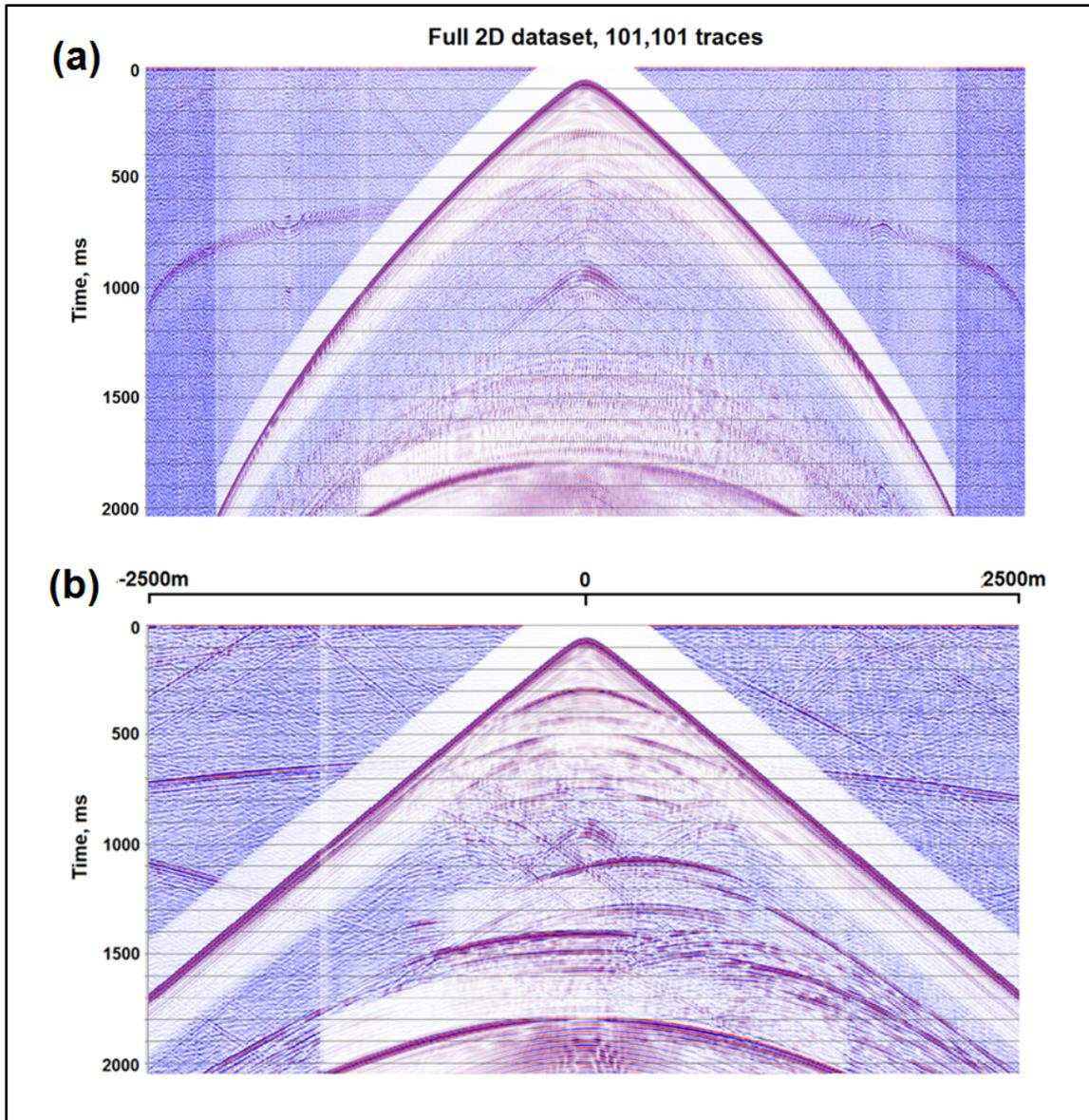
Figure 2: (a) AGC plot of all seismograms from the 2D survey, sorted into common-offset gathers (AGC window=1000ms). The relevant reflections from the targets lie above 1700ms. The hyperbola at 1800-2000ms is the primary reflection from the water-air interface. (b) AGC plot of a sample common-source gather (AGC window=200ms). The bottommost hyperbola is the primary reflection from the water-air interface
