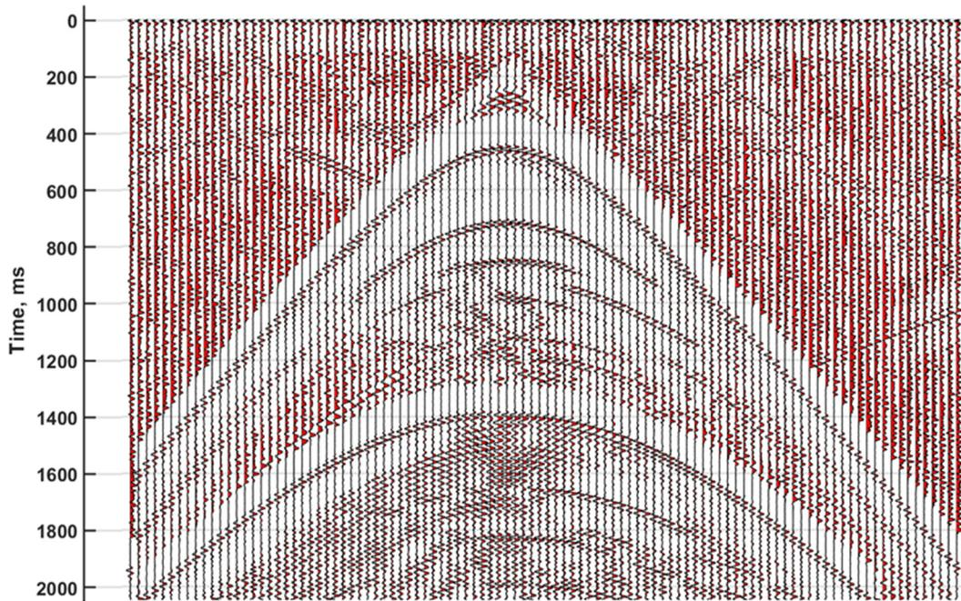
Figure B2: AGC display of a common-source gather recorded with an impulsive subsurface source (AGC window = 200ms). Individual seismic arrivals are clearly discernible.
