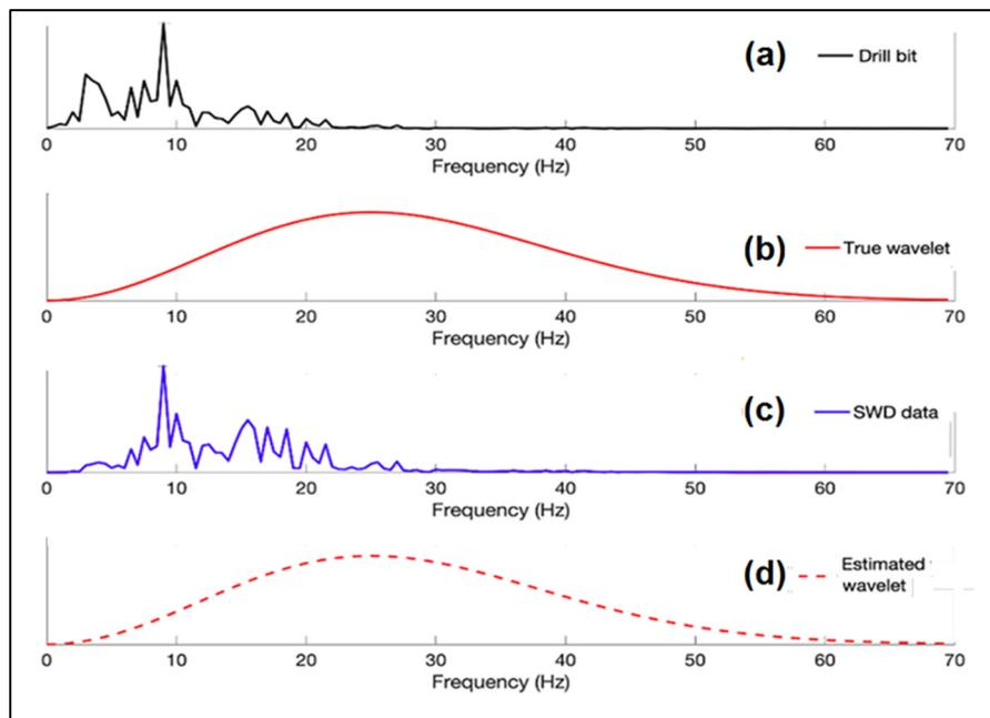
Figure B5: Frequency-domain equivalent of convolution and deconvolution of a drill-bit waveform with an impulse-response wavelet: Spectrum (c) is the product of spectra (a) and (b); Spectrum (d) is spectrum (c) divided by spectrum (a) plus a small stabilizing factor.
