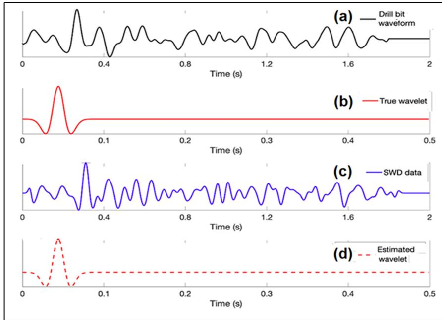
Figure B4: Time-domain convolution and deconvolution of a drill-bit waveform (a) with an impulse-response wavelet (b). In SWD acquisition, recorded trace (c) is the convolution of ((b) with (a)). Trace (d), a version of trace (b) estimated from trace (c), is recovered by deconvolution.
