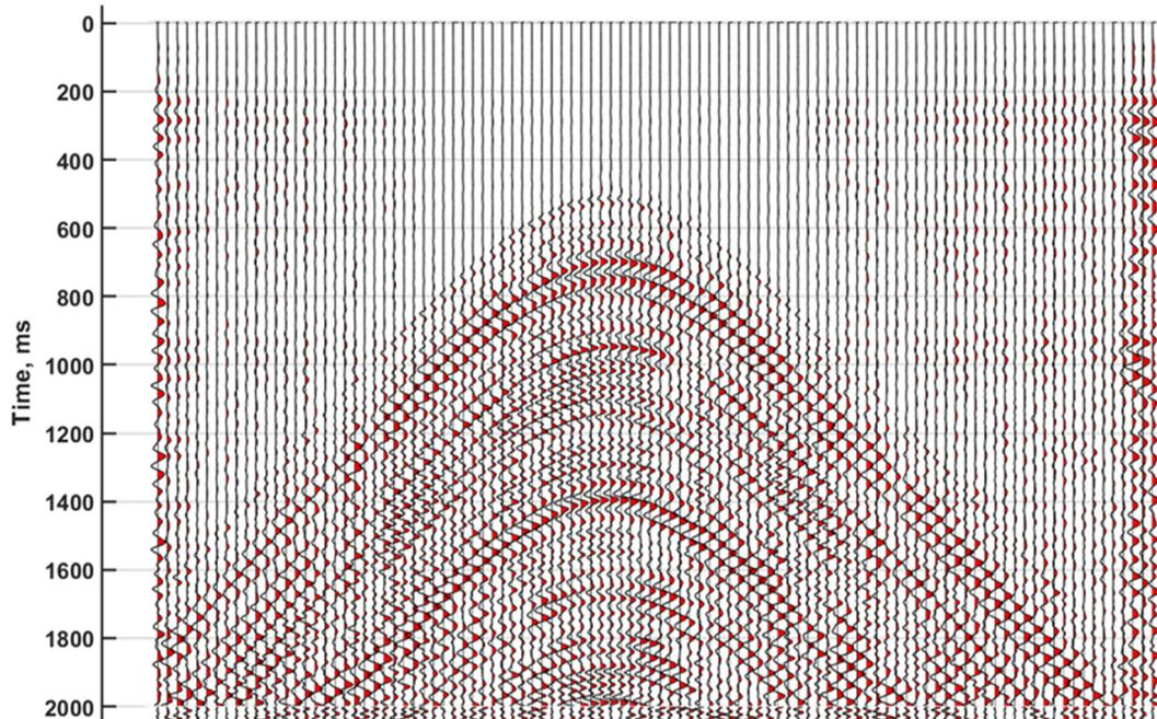
Figure B3: Normalized display of the common-source gather in Figure B2 convolved with the drill-bit signal on Figure B1. It is not possible to see individual seismic arrivals clearly.
