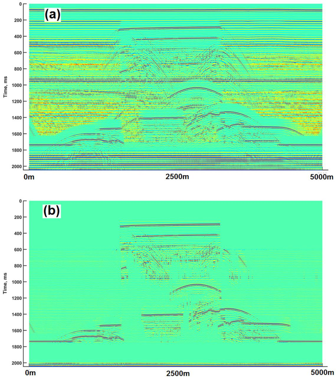
Figure 3: (a) AGC plot of unprocessed data from the high-resolution zero-offset survey, showing many (low-amplitude) extraneous events that may pose challenges to processing and imaging. Trace spacing is 5m. (b) The same display after applying amplitude discrimination. Reflections from the main boundaries of the physical appear with less interference from extraneous events.
