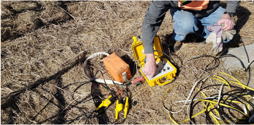
FIG. 3. The Geostuff downhole interface and control box. This one has been modified to use an Aries RAM battery to power the clamping mechanism.
