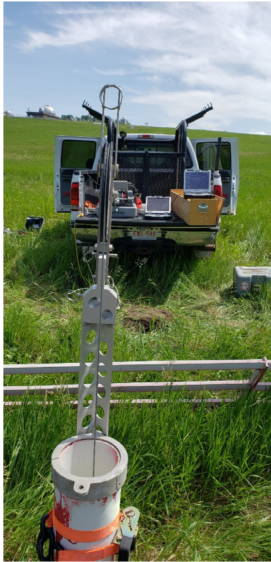
FIG. 14. The Mount Sopris equipment mounted on the back of a pickup truck. The winch cable also has the electrical connections built in and can be seen going down the test hole via a wheel to avoid the sharp edge of the well casing.
