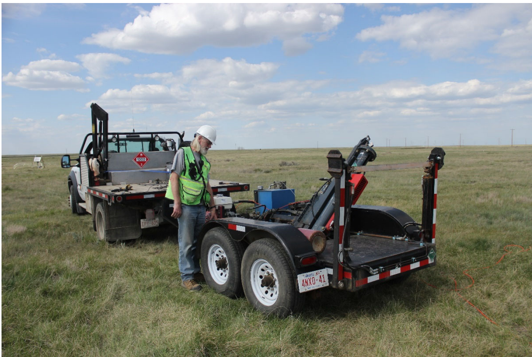
FIG. 6. The nitrogen spring shear wave capable thumper. Malcolm for scale.
