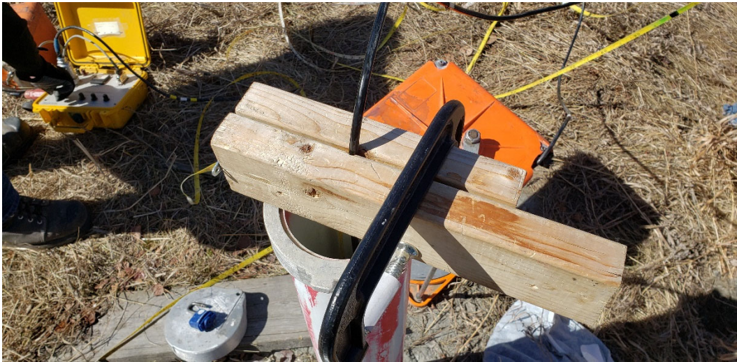
FIG. 11. The top of the eastern test well at the Rothney Astrophysical Observatory field. The Geostuff cable is clamped using to pieces of wood hinged together and held tight with a c-clamp. The Geostuff box is in the top left of the picture.
