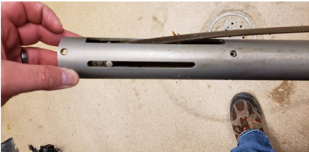
FIG. 4. The bow spring clamp that holds the tool in place in the well/test hole.
