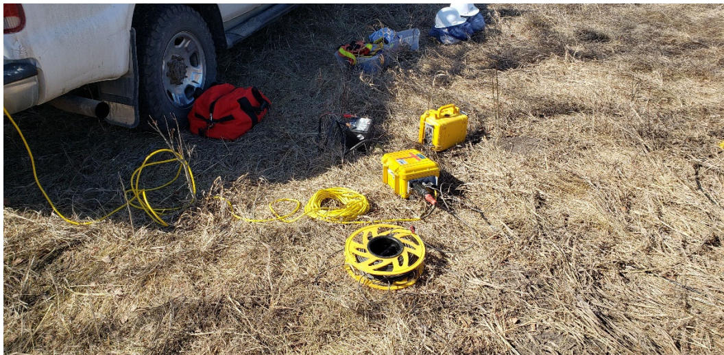
FIG. 12. The Geode node that the downhole geophone is connected to in front of a spare Geode.
