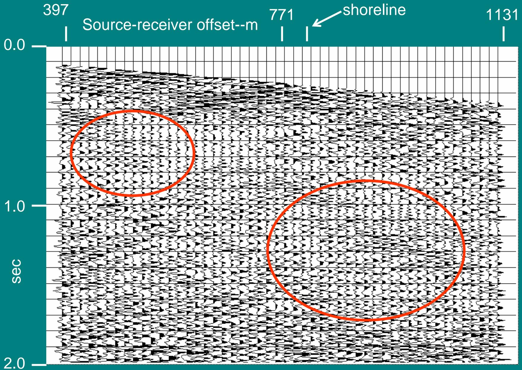
**Gabor deconvolution applied in X-T domain—R-T domain spectral clipping**
