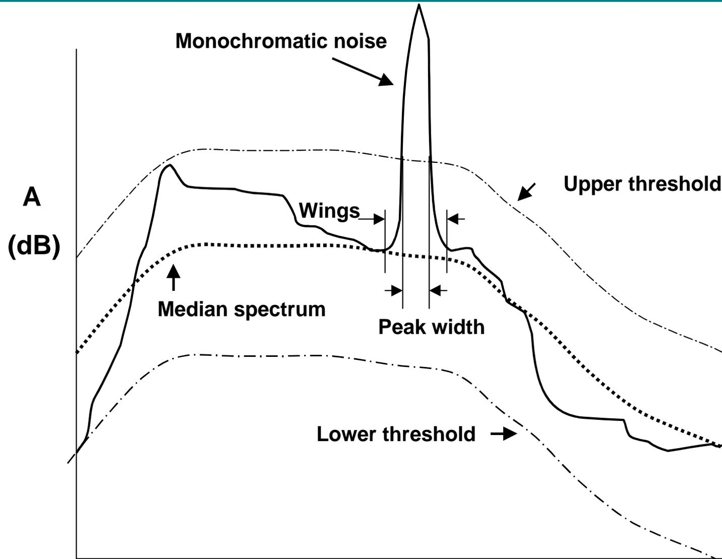
Median spectrum computed from raw spectrum; threshold curves placed parallel to median; peaks in raw spectrum exceeding threshold are flagged
