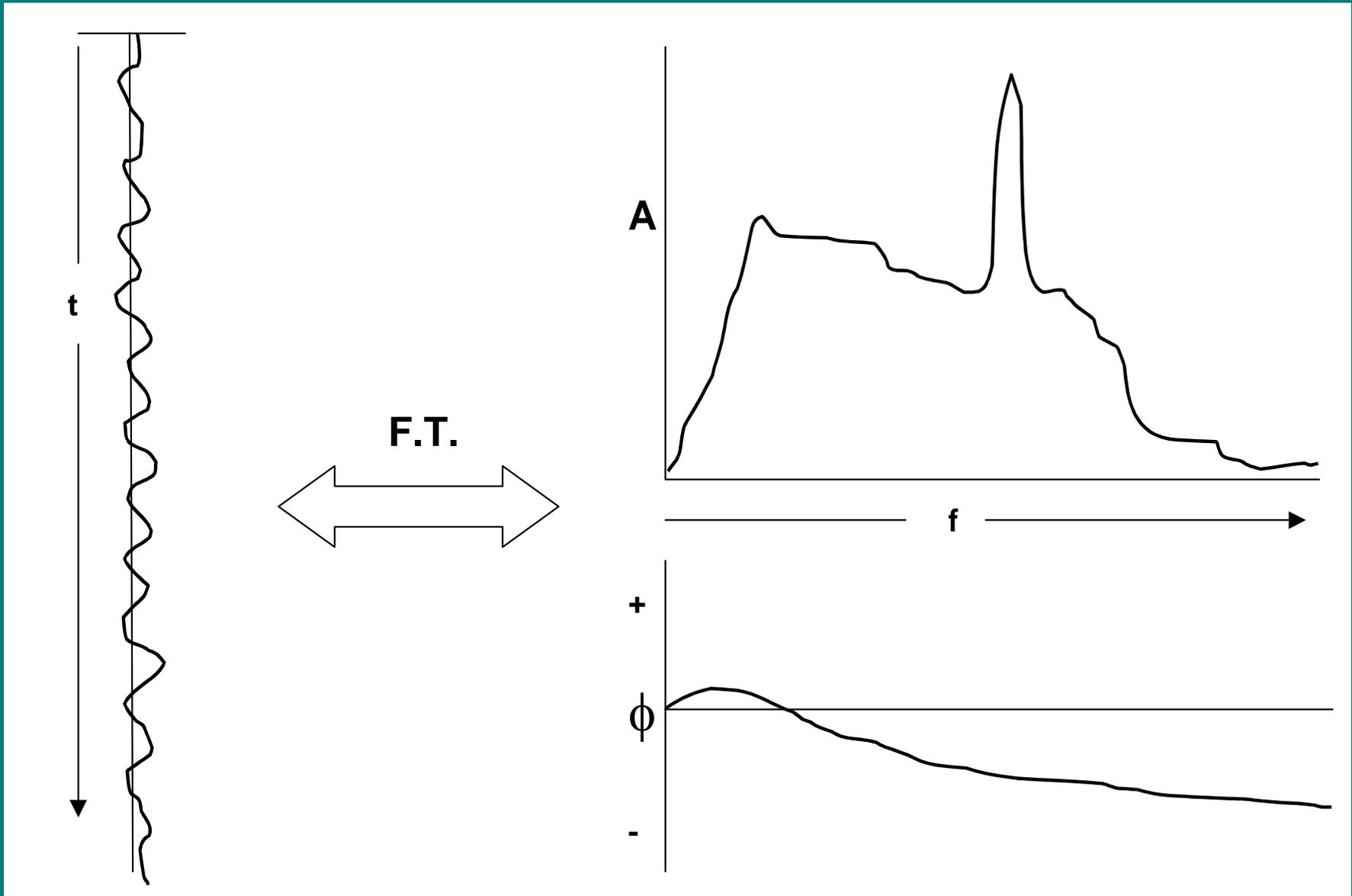
**Seismic trace contaminated with monochromatic noise is transformed to frequency domain**
