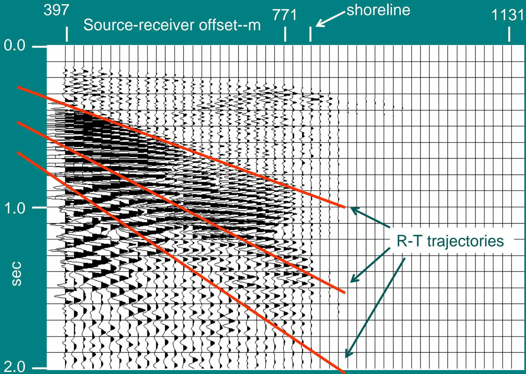
**Unscaled raw shot gather: source point on floating ice. R-T trajectories encounter monochromatic noise, due to dispersion of ice wave**
