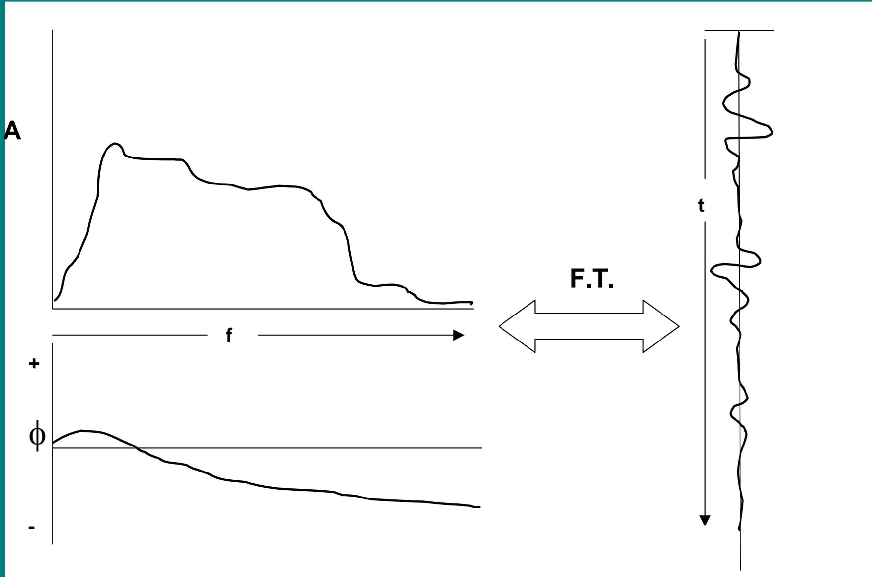
**Edited spectrum is transformed back to seismic trace, sans monochromatic noise**
