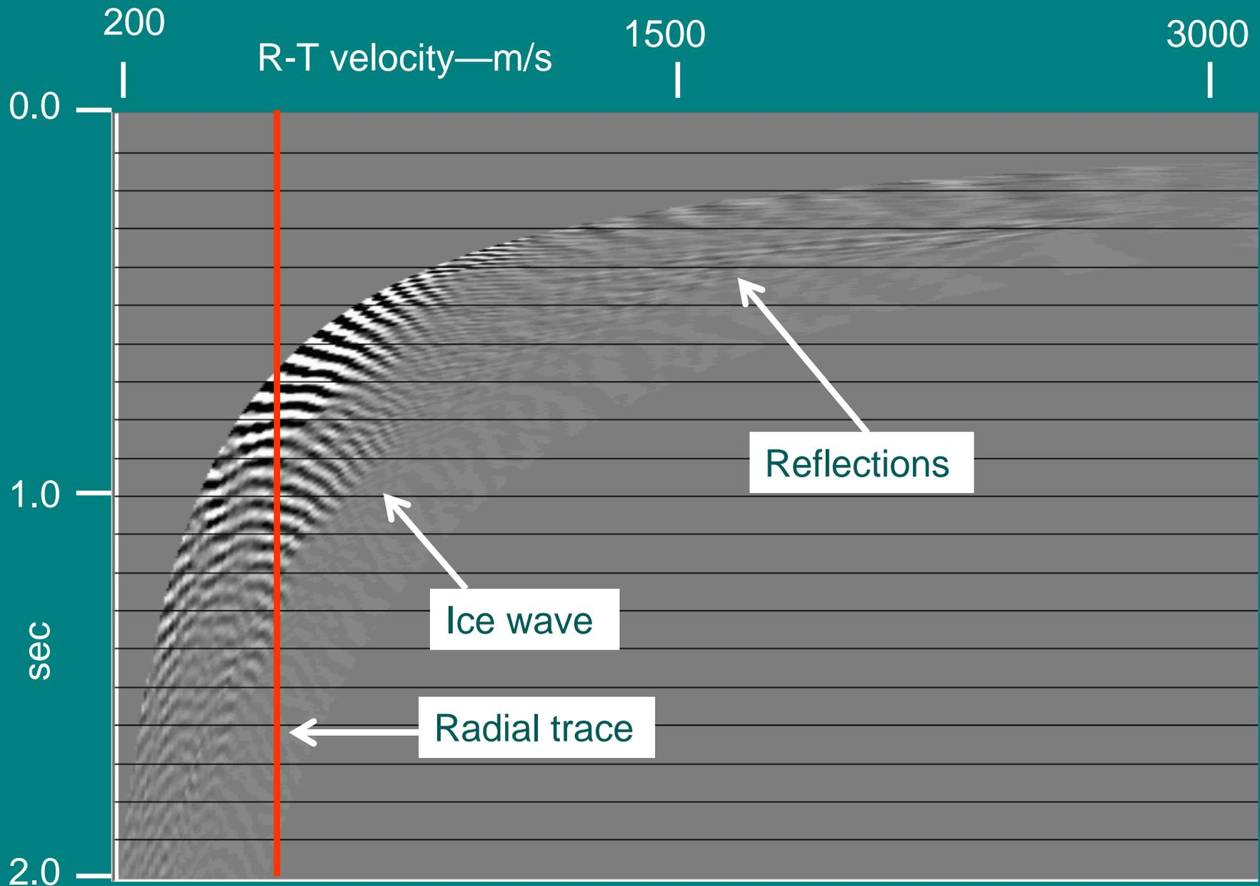
**R-T fan transform of raw shot gather—ice wave on radial trace is monochromatic**
