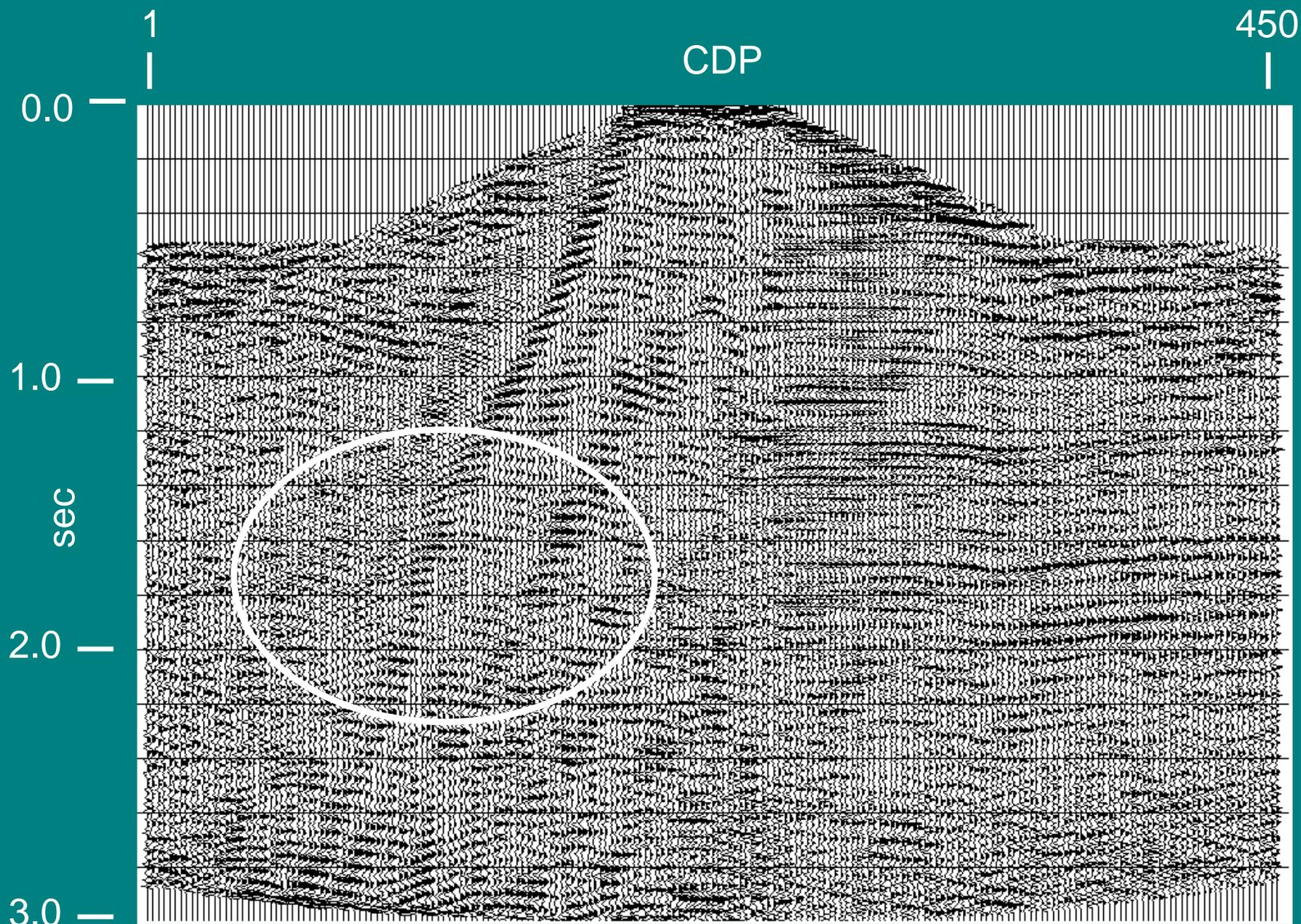
**Brute stack of Hansen Harbour line with no ice wave filtering**
