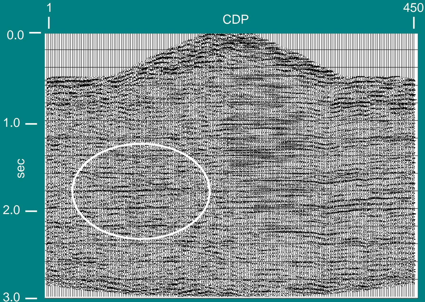
**Brute stack of Hansen Harbour line after ice wave filtering**
