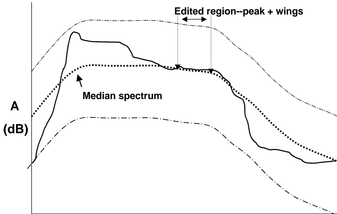
Flagged raw spectral amplitudes are replaced with median values,
