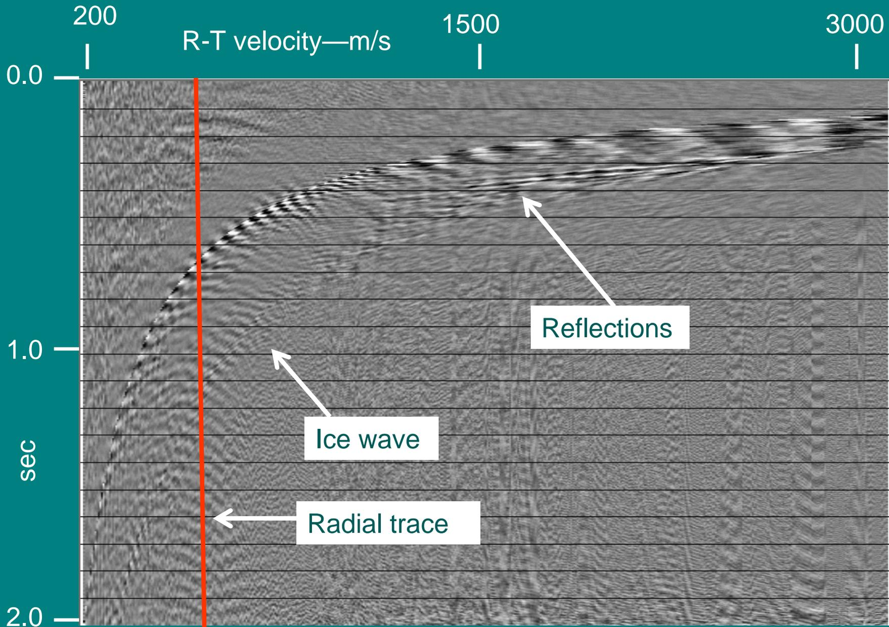
**R-T fan transform of raw shot gather after spectral clipping—monochromatic noise greatly attenuated**
