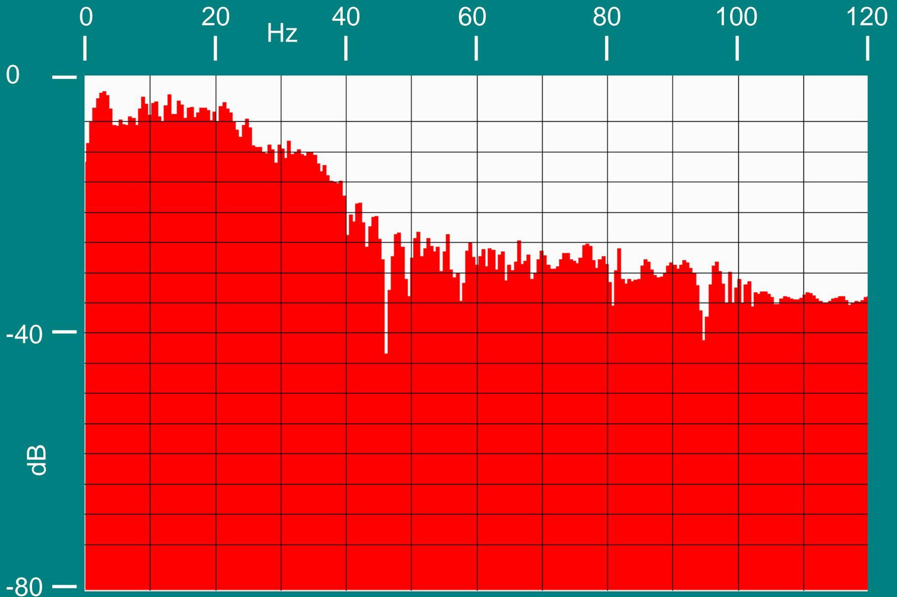
**Spectrum of radial trace with ice wave noise after spectral clipping**
