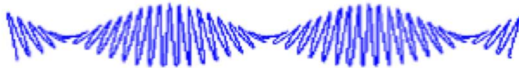
Figure 12 The Twisted Strip Cable – another broad-side sensitive cable based on the “shaped fibre” concept. A sinusoid is made of fibre in one plane (the strip) and then twisted to achieve sensitivity in all directions.
