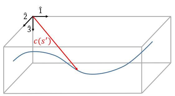
Let **c** be a vector pointing from the origin to a point at a distance s' along the cable, such that,
