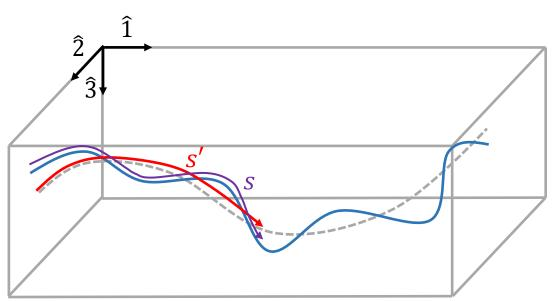
Knowing the arc length of the total cable-fibre system *s* is crucial to the model. Following the previous formulaic development for the cable arc length.
