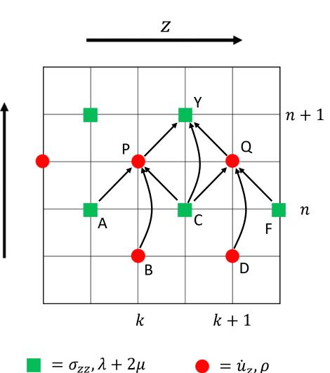
The velocity-stress finite difference formulation is unique because it solves the system of equations on a staggered grid, improving accuracy and stability,
