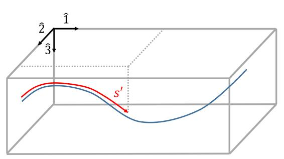
The arc length is the sum of the length of each derivative component along the cable,
