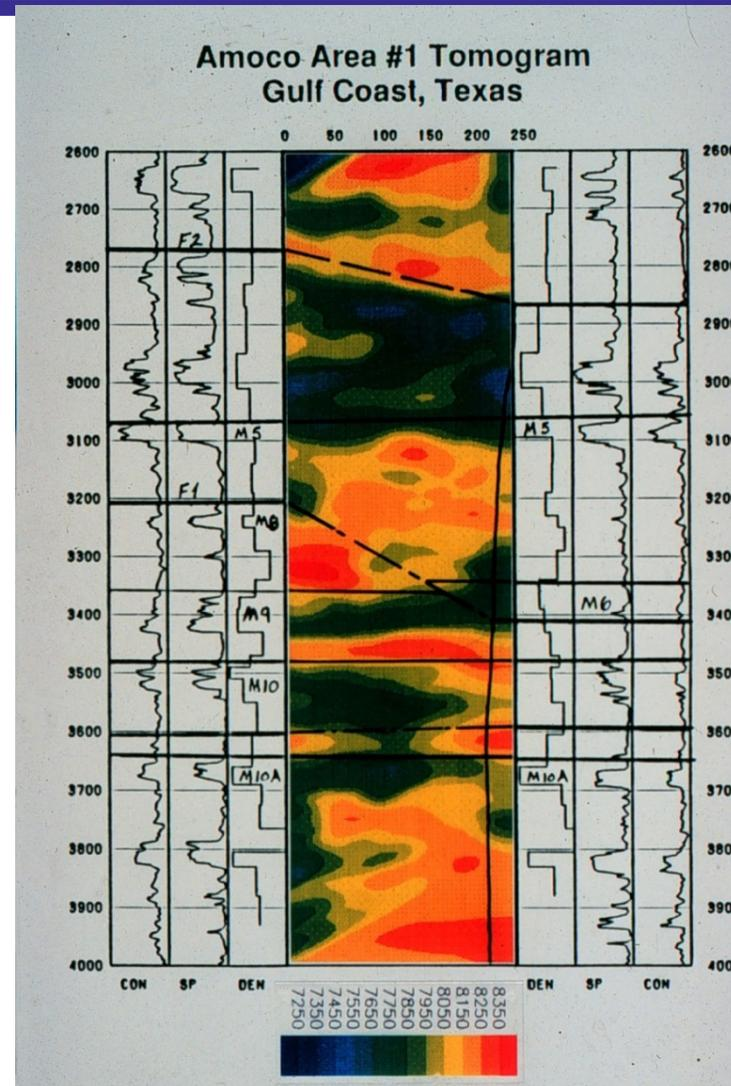
This cross-borehole tomogram, from Harris et al. (1990 SEG annual meeting ) and later shown in Lines (1991), indicates the location of two faults between boreholes in East Hastings field, Texas.
