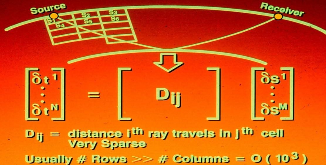
These sets of equations are iteratively solved and  $\mathbf{D}$  is updated at each iteration after ray tracing with the updated slowness model. Convergence is said to occur when the differences between data and modeled traveltimes are small enough.
