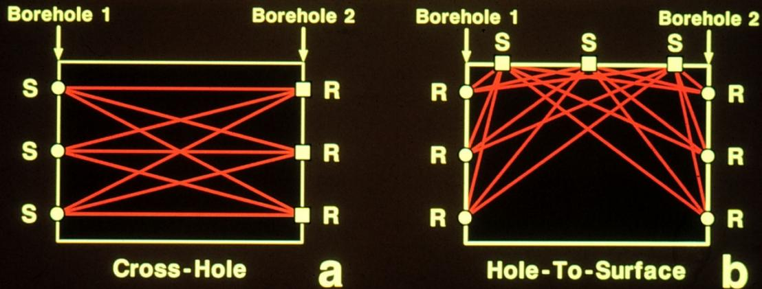
Combining these borehole configurations will allow us to do CT scans of the Earth – albeit with incomplete apertures.
