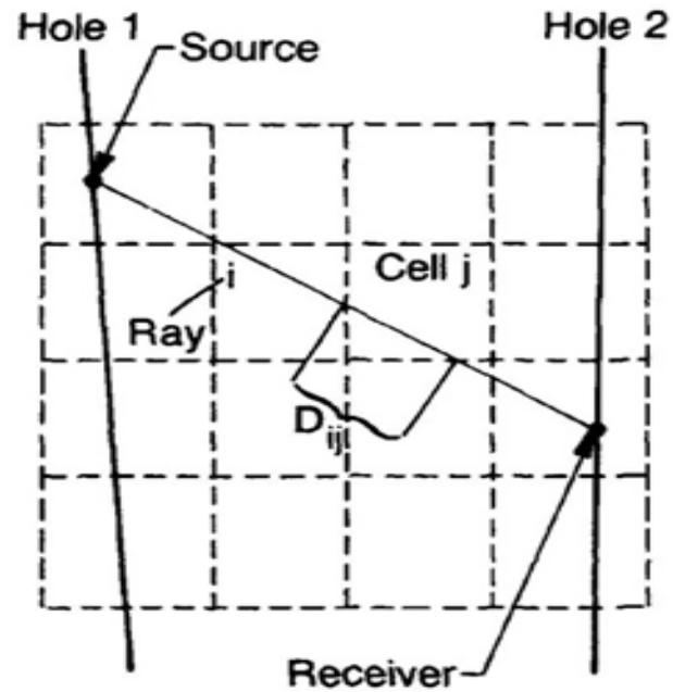
*The  $i$ th ray travels a distance  $D_{ij}$  in the  $j$ th cell (after Bording et al., 1987).*
