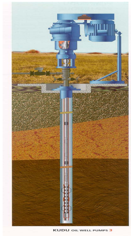
Figure 1.2 A schematic diagram of a cold production oil pump (courtesy of Kudu Oil Well Pumps)
