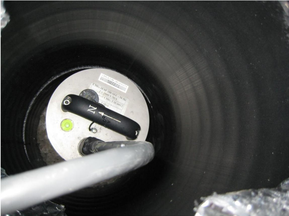
**Figure 1.5 Photo of seismometer at station INUQ.**
